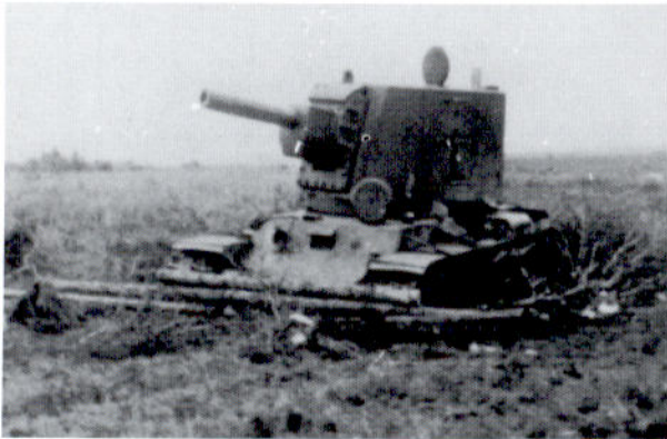
The war in Finland convinced the Red Army of the need for a heavy howitzer tank to destroy bunkers. A small number of KV hulls were modified with a special large turret, fitted with a 152 mm howitzer, later called the KV-2. This early production KV-2 of the 5th Tank Division was abandoned in its entrenchment near Alitus, Lithuania, during Operation 'Barbarossa' in June 1941. (US National Archives)
