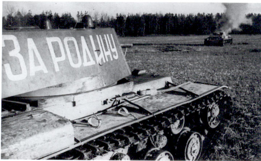
A colourfully marked KV-1 Model 1941 moves forward past a smouldering German PzKpffw IV on the Southwestern Front in 1942. This is one of the original KV-1 Model 1941 configurations with the early pattern welded turret, early style resilient roadwheels, and the initial pattern turret ring appliqué. The slogan on the turret is Za Rodinu – 'For the Homeland'.
