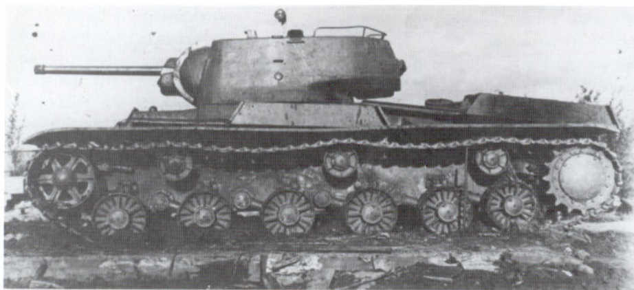
In 1942 there were some experiments to mount artillery rockets on tanks such as this KV-1K. Two armoured boxes were fitted on the fenders, each containing two rail launchers for RS-82 Katyusha rockets. Ultimately, this idea was dropped, probably due to the inaccuracy of the rockets. (R. Ismagilov)
