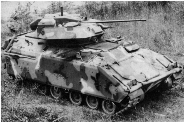
The CFAST was one of the early attempts to up-arm the Bradley to respond to future Soviet infantry vehicle developments. In the event, the new BMP-3 is not well armoured, and the end of the Cold War has pushed the follow-on COMBAT programme into a low-priority slot. (United Defense LP)
