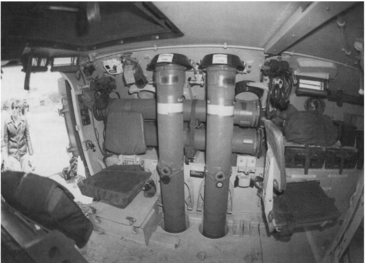
The left hand interior of the M2 Bradley IFV has stowage for four TOW or Dragon anti-tank missiles. This places them within easy reach of the crewman in the left rear of the troop compartment for reloading the TOW launcher. (Author)
