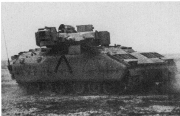
This rare shot shows one of a handful of Bradleys fitted with the VLQ-7 Stingray electro-optical jammer deployed to Saudi Arabia for 'Desert Storm'. This medium energy laser device was designed to blind electro-optical sensors such as tank sights, and was fielded as a possible response to Iraqi use of lasers to blind troops.
