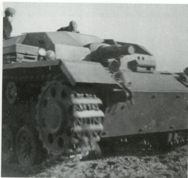
The second series of Sturmgeschütz Ausf. A was, for some unknown reason, built on the chassis of the Pz.Kpfw. III Ausf. G. As the frontal armour on the existing Pz.Kpfw. III was only 30 mm thick, an additional 20 mm plate was bolted on to create a 50 mm front. This series may be identified by the armoured air intake covers on the upper nose plate and the hull side escape hatch. (Karl Heinz Munch)
