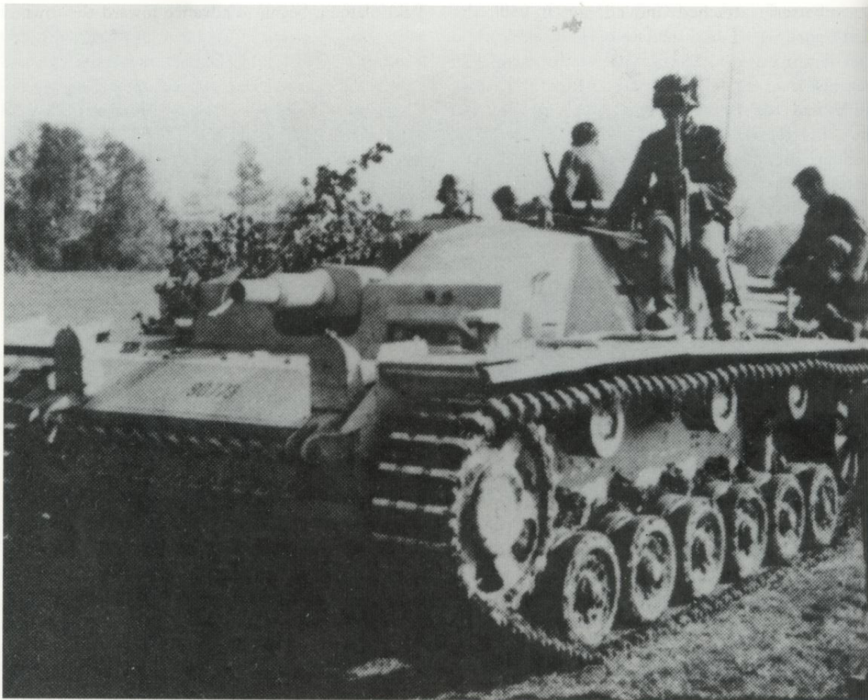
A Sturmgeschütz Ausf.E (Fgst.Nr. 90773) with the superstructure of an Ausf.D – an arrangement which typifies the gradual changes introduced to the vehicle during its production run.
