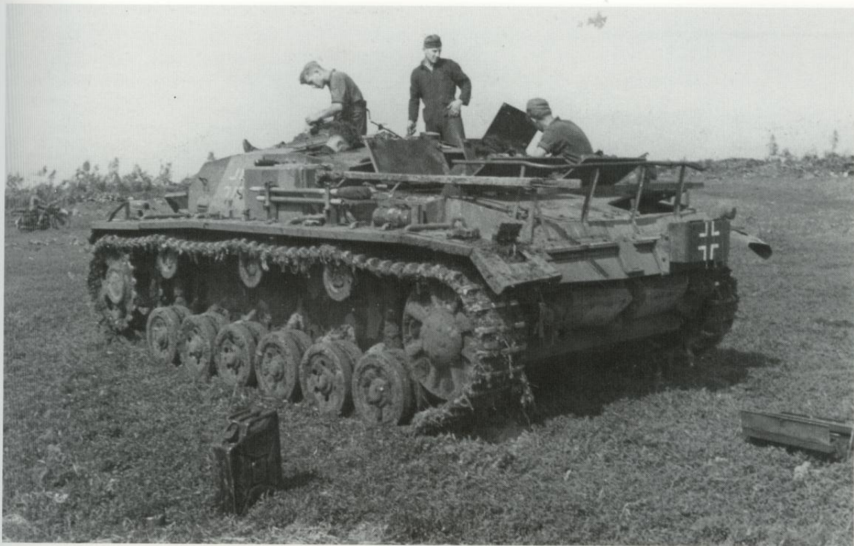
Rear view of a Sturmgeschütz Ausf. B. This vehicle is a later production Ausf. B with the new cast drive sprocket and the armoured housing for the smoke candle rack. (Bundesarchiv 77 3064 4)
