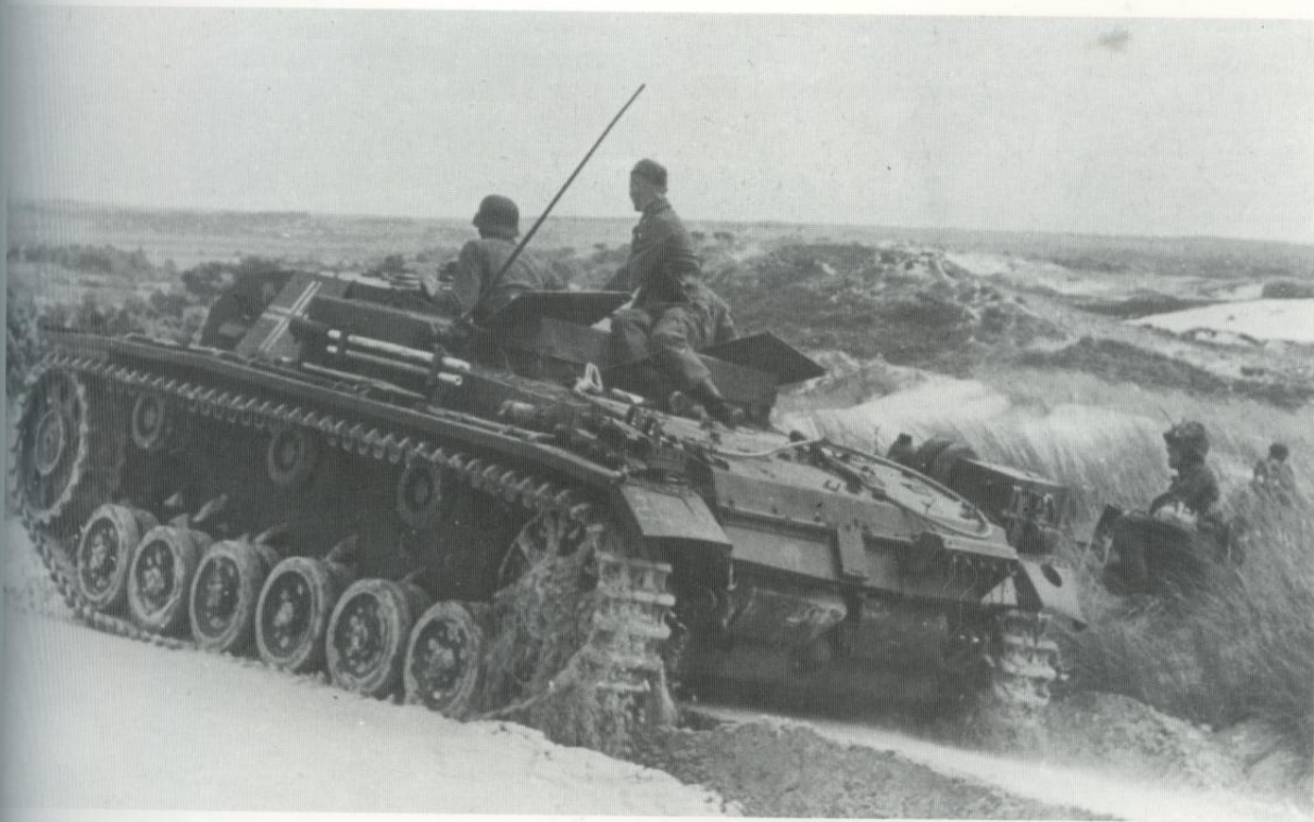
Rear view of one of the first Sturmgeschütz Ausf. B delivered to Sturmatterie 667 on 12 September 1940. The old drive sprocket has been modified by fitting a spacer to accommodate the wider Kgs 61/400/120 track. (Bundesarchiv rot 79/67/8)
