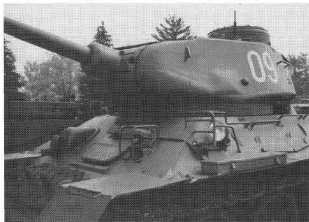
The T-34-85s built in Poland and Czechoslovakia in the early 1950s can be distinguished by their turret castings, which are noticeably smoother than Soviet examples. In addition, the shape of these turrets is also somewhat different. This Czechoslovak-manufactured T-34-85 went through the post-war rebuild, being refitted with a Czech Notek night driving lamp instead of the usual Soviet type. It served with the East German NVA, but was later donated to the Canadian tank museum at Camp Borden near Ottawa.
