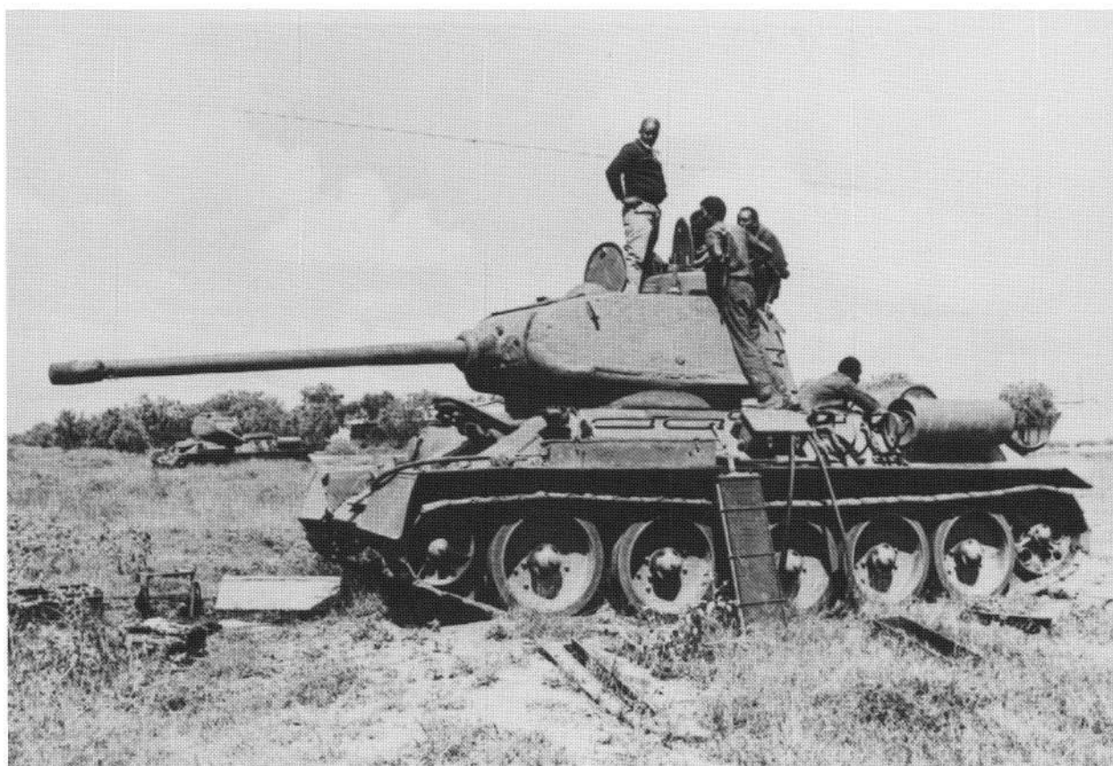
Above: During the war between Ethiopia and Somalia over the Ogaden in 1978, the T-34-85 was used by both sides. Here, Somali engineers repair a captured Ethiopian T-34-85 Model 1969 for use by the Western Somali Liberation Front. This vehicle has the full Model 1969 retrofit, including the rear fuel rack, the infra-red night driving equipment, and the external fuel pump. The turret is a post-war composite type with the split mushroom ventilators.
