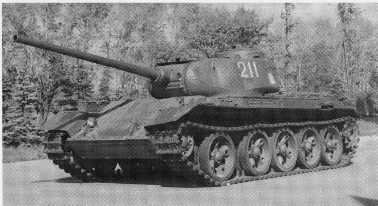
The successor to the T-34-85 was the T-44 medium tank. The turret of the T-44 bears many similarities to the T-34-85, though in fact it is substantially different in many details. This is a rebuilt T-44M preserved at the World War 2 memorial at Poklonna hills southwest of Moscow. It still retains the original narrow tracks, but has been rebuilt with the 1969 starfish wheels.
