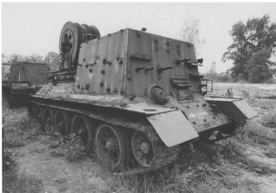
Following the retirement of many T-34-85s in the 1960s, the Polish Army's WITPiS converted some surplus chassis into the WPT-34 armoured evacuation tractor. This vehicle, currently preserved at the Polish Army Museum near Warsaw, has much of its specialised tools removed, providing a clearer view of the new superstructure.
