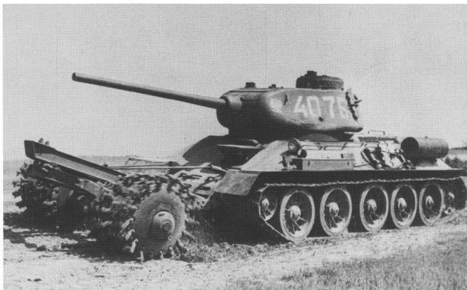
The T-34-85 could be fitted with the PT-34 mine trawl. These were used in special tank regiments for breakthrough operations to help clear defensive mine belts. This is a post-war example mounted on a Polish T-34-85. (Janusz Magnuski)
