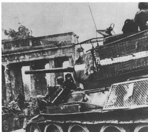
During the battle for the Seelow Heights on the approaches to Berlin, tankers of the 11th Tank Corps and several other units created improvised anti-panzerfaust screens by taking bed springs from German homes and fastening them to the turret and hull side. The aim was to detonate the panzerfaust warhead before it struck the armour, weakening its penetration power. This T-34-85 of the 36th Tank Brigade, 11th Tank Corps, rests at the foot of the Brandenburg Gate in May 1945 following the capture of Berlin.
