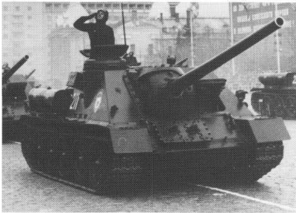
An SU-100 Model 1969 takes part in the May 1990 Victory Day celebrations in Moscow commemorating the 45th anniversary of the war. This appears to be an SU-100 built during the war, but it features the Model 1969 upgrades including the starfish wheels, fuel pump external storage box and the infra-red driver's headlight.
