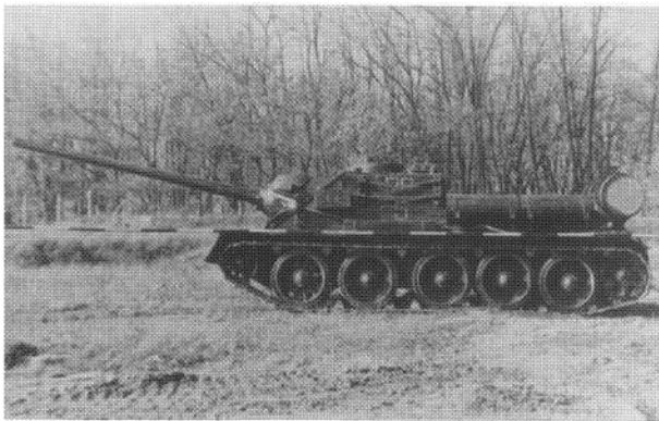
The SU-100 Model 1969 still serves in several armies, including the Romanian Army as seen here. This vehicle shows many of the Model 1969 refits, including the fuel pump box and cable assembly on the superstructure side, and the new storage racks for 200-litre fuel drums on the hull rear.
