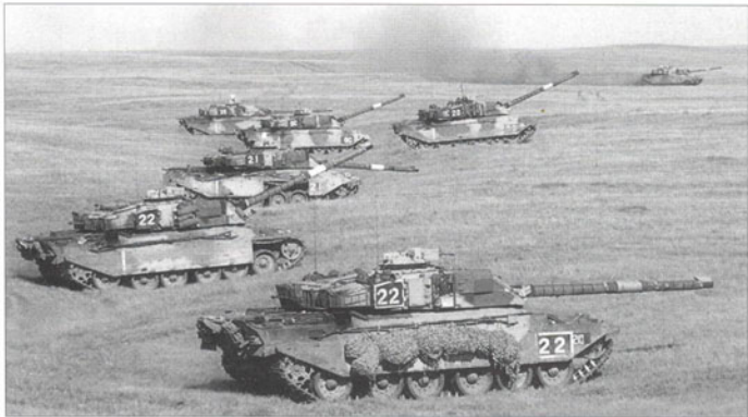
A group of Challenger 1s shelter in a fold in the ground on the wide open prairie at BATUS in Canada - those of 1st Armoured Squadron (white fume extractors and white stripes on rear bazooka plates) are at 'check fire' with their main armaments fully elevated while the one at full depression is checking the Muzzle Bore Sight. In the foreground is a Challenger 1 of 2nd Armoured Squadron which can be identified by the white border around the call sign. (Media Ops Land Command)
