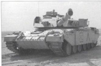
With the armoured door of the TOGS barquette open, a Challenger 1 Mark 3 of The Queen's Royal Irish Hussars displays the full array of supplementary armour fitted to the Challengers of 1st (UK) Armoured Division during Operation Granby, with Chobham armour panels along the sides and Explosive Reactive Armour (ERA) on the glacis plate and toe. (QRIH)
