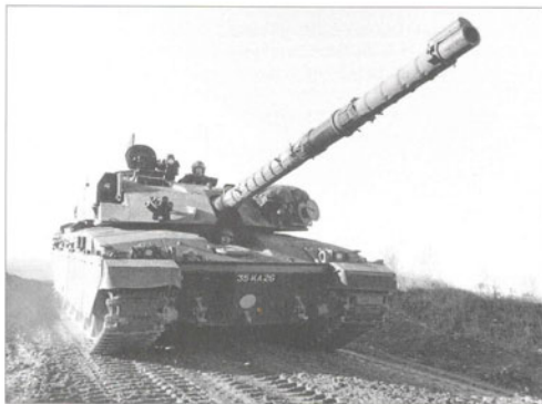
A Challenger 1 Mark 2 of 2nd Royal Tank Regiment moves off on a 'battle run' on the tank gunnery ranges at Hohnle during 1989. With a high reputation for gunnery, 2 RTR failed the cut for CAT '87 which was to have far reaching ramifications to the future of Challenger. Here, the L11A5 120mm with its thermal sight is shown to advantage. (MOD)
