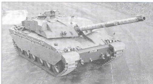
ABOVE The first production model Challenger was delivered to the British Army on 16 March 1983 during a ceremony at the Royal Ordnance Factory Leeds. Although this vehicle has the armoured barbette for TOGS on the turret side, TOGS was still under development so this is a Challenger Mark 1. Once TOGS was installed the tank became a Mark 2. (MOD)
