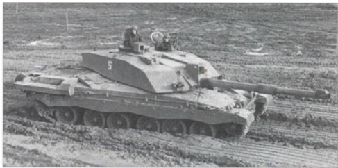
V5 - the fifth Challenger 2 prototype churns through the mud during a demonstration before the Defence Minister of Saudi Arabia on Salisbury Plain in 1993. This model features TECs or Thermal Exhaust Cows which are a wartime fitting to reduce the tank's thermal signature. (MOD)
