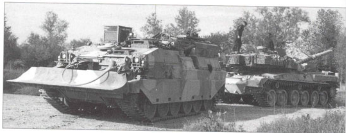
Camouflaged in the characteristic yellow and green disruptive stripes of OPFOR (Opposing Forces) vehicles, a CRARRV prepares to tow a Chieftain of 1 RTR during Exercise Phantom Bugle on Salisbury Plain in June 1995. CRARRV has a multi-purpose blade which can operate as an earth anchor, dozer blade or stabiliser for the hydraulically-operated crane, with all controls under armour and is equipped with a hydraulically-driven double capstan winch and an independent auxiliary winch. (Tim Neate)
