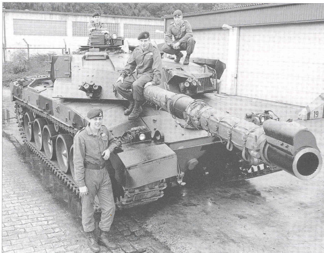
ABOVE The first production model Challenger was delivered to the British Army on 16 March 1983 during a ceremony at the Royal Ordnance Factory Leeds. Although this vehicle has the armoured barbette for TOGS on the turret side, TOGS was still under development so this is a Challenger Mark 1. Once TOGS was installed the tank became a Mark 2. (MOD)
