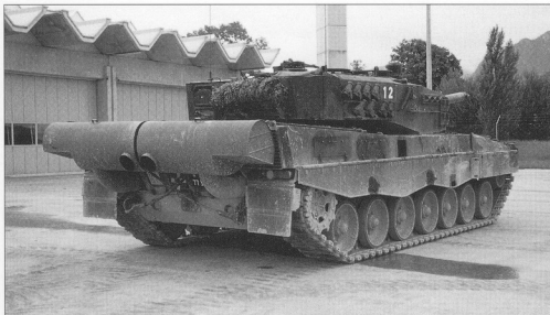
Switzerland was the first country to adopt extra noise-reducing mufflers with their Pz 87 as seen here on a vehicle of the Armour School in Thun. (Andreas Kirchhoff)
