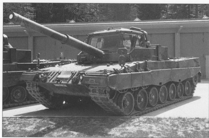
The driver training tank is basically a regular Leopard 2 MBT with a glasshouse cabin, extra weight and dummy gun instead of the regular turret. The licence plate number is quite interesting, as it denotes that this vehicle came off the assembly line at MaK immediately before the TVM II. (Gerd Schwiers)
