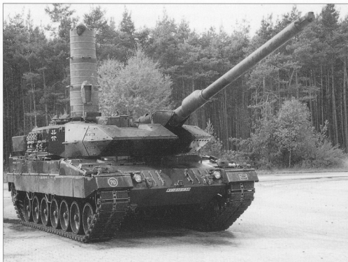
Two Leopard 2 A5's were used for troop trials with the longer 120 mm L/55 smooth bore gun at the German Armour School in 1997, with both crews coming from PzBtl. 33. The vehicle shown here has just finished a deep wading operation and the three-piece snorkel is attached to the commander's station. (Michael Jerchel)
