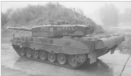
This Leopard 2 A4 (second batch) was used to test a pair of mufflers, already a common sight on the Swiss Panzer 87. (Uwe Schnellbacher)
