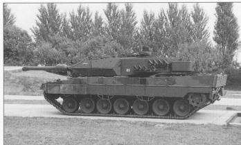
A recently completed Leopard 2 A5 on the test course at MaK in Kiel, where it was converted from a seventh-batch vehicle. The new components have not yet been painted in the proper camouflage colours. (Michael Jerchel)
