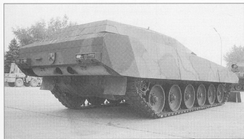
This rear view of the EGS trial vehicle reveals the large mufflers carried at the rear. Although bearing a close resemblance to the Leopard 2, it is in fact a new chassis with larger road wheels and has a lower hull that is optimised for mine protection. (Michael Jerchel)
