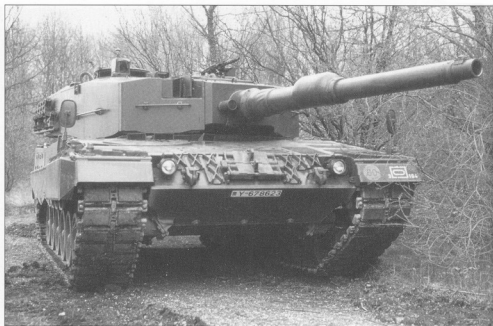
Three pre-series vehicles and two pre-series turrets were delivered in 1978 to the German Armour School in Münster. Shown here is the third pre-series chassis with the second pre-series turret and fake tactical markings. (Krauss-Maffei-Werkfoto)
