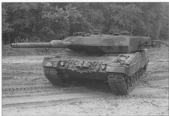
A Leopard 2 A5 NL of 42nd Tank Battalion, the first unit so equipped, which received its first improved Leopard 2 in May 1997. The Dutch-built smoke mortars are clearly seen on the turret side. (Michael Jerchel)
