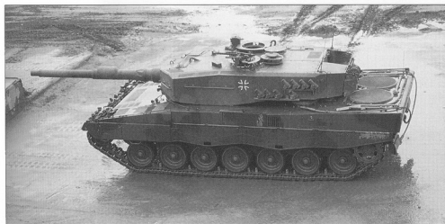
Late sixth-batch vehicles introduced new forward sections for the side skirts, as seen here at a demonstration exercise in Münster during 1992. (Michael Jerchel)
