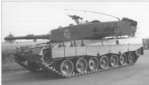
A Leopard 2 NL of 41st Tank Bataljon, with the unit crest applied to its turret sides, is seen here during exercise 'Free Lion' in September 1988. The FN MAG machine gun, Dutch smoke mortars and antenna base are shown to good advantage. (Michael Jerchel)
