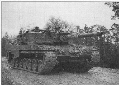
Up to 18 grousers can be fitted to the tracks in place of rubber pads for use on soft ground or snow, as seen here on a Leopard 2 A4 (sixth batch) on exercise at the CMTC in Hohenfels. (Carl Schulze)
