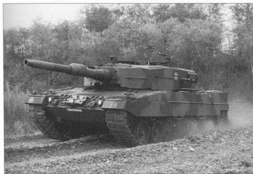
The eighth batch introduced new rear sections for the side skirts and slightly reshaped mounts for the smoke mortars. The collimator of the muzzle reference system is not yet fitted. (Krauss-Maffei-Werkfoto)
