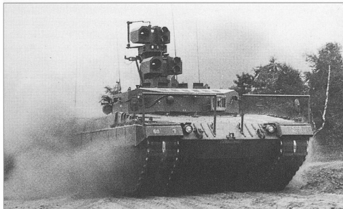
This rather unusual looking VT-2000 (Versuchsträger experimental vehicle) was intensively tested at the Armour School as part of the IFIS programme. (FMZ/Panzertruppenschule)
