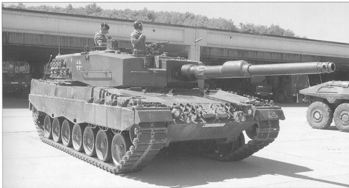
The divisional reconnaissance battalions were also equipped with the Leopard 2 A4. This fifth-batch vehicle of PzAufkIBtl. 2 shows the collimator at the right side of the barrel's end, fitted in 1994. (Michael Jerchel)
