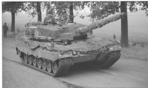
A Leopard 2 NL of 41 Tankbataljon, seen during exercise 'Light Viper' in 1993. Camouflage netting is draped around the turret to break up the vehicle's silhouette. (Michael Jerchel)
