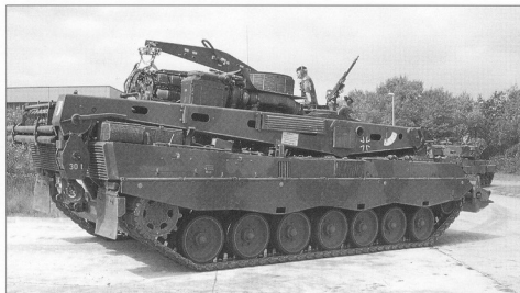
A Bergepanzer 3 Büffel of PzBtl. 33, with a spare power pack on the special rack attached to its engine deck, during an exercise in 1994. The power pack weighs about 6100 kg. (Michael Jerchel)
