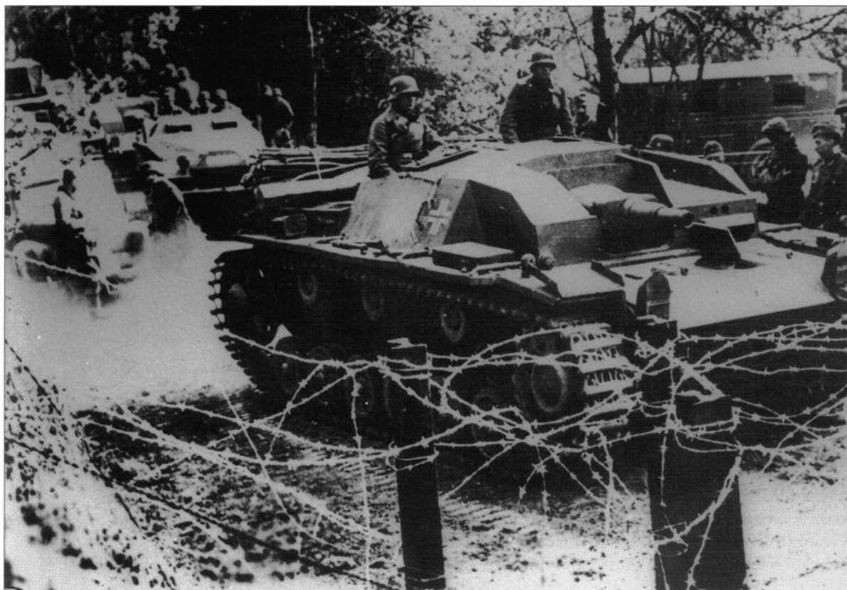
The PzKpfw III's most famous derivative, the Sturmgeschütz (assault gun). This early example, armed with a L/24 75mm howitzer, was one of only four batteries employed during the 1940 campaign in France. (RAC Tank Museum)
