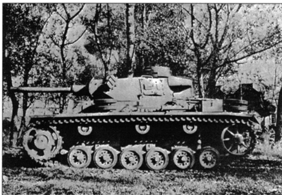
The flame-thrower version of the PzKpfw III closely resembled the Ausf. L and M, but was recognisable by the thicker barrel of the flame projector tube. The cylinder dimly visible at hull rear is part of the deep-wading exhaust system. (Imperial War Museum)
