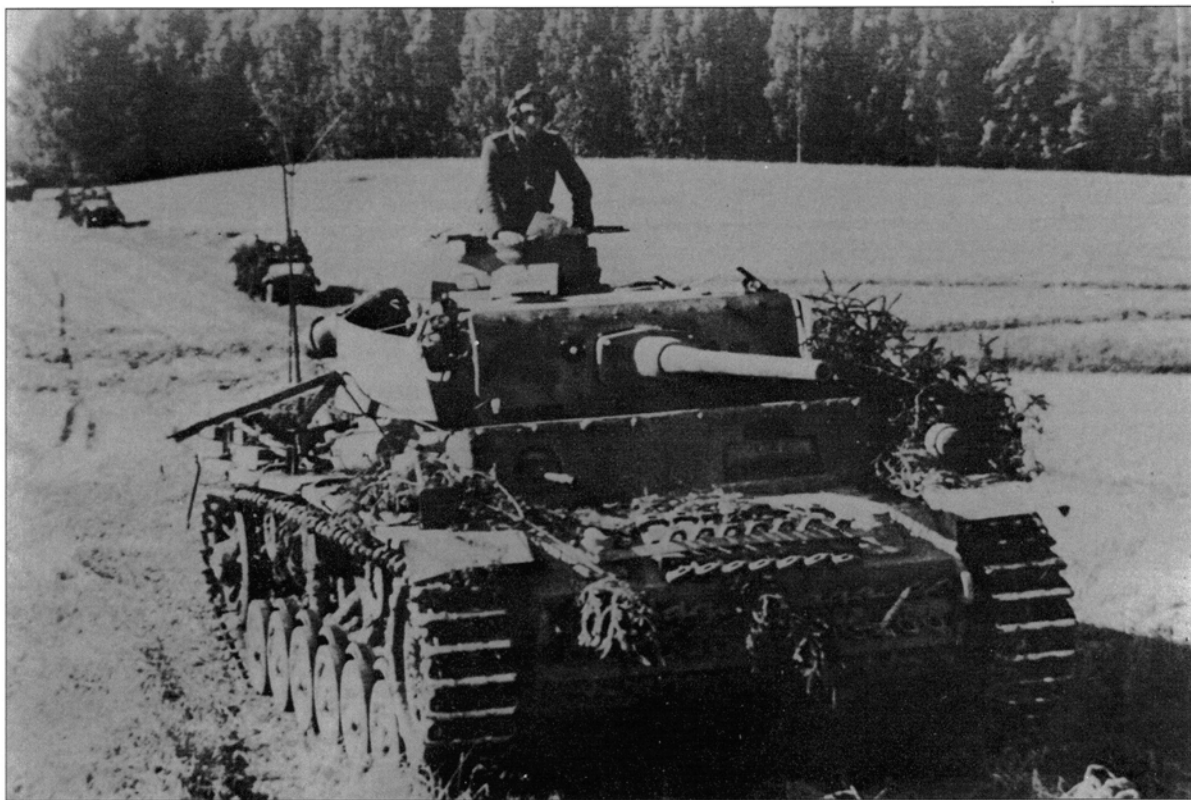
Later versions of the Panzerbefehlswagen III dispensed with the frame aerial and employed a branched antenna instead, as carried by this example working with a Panzergrenadier unit. (Bundesarchiv)
