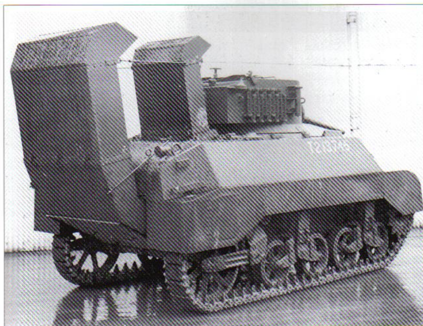
Britain was one of the main recipients of the M3A3 light tank, where it was known as the Stuart V. By this stage of the war, it was used primarily as a reconnaissance tank. Prior to the Normandy landings, they were fitted with deep wading trunks for amphibious operations as seen here. (The Tank Museum)
