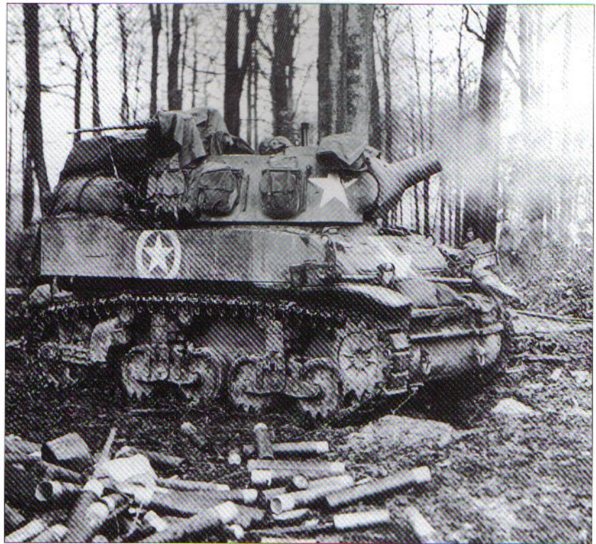
The only self-propelled gun version of the Stuart to reach production was the M8 75mm howitzer motor carriage. This mounted a short 75mm howitzer in an open turret on a modified M5 light tank hull. There were six of these assigned to each armored cavalry squadron, providing fire support to other vehicles in the unit with their short-barreled 75mm howitzer. This is a US Army M8 75mm HMC of Troop E, 106th Cavalry Reconnaissance Squadron during the fighting near Karlsbrunn on 2 February 1945. This vehicle is fitted with the Kelsey-Hayes road-wheels, and the standard T16 block track with grousers attached for better traction in mud. (US Army MHI)
