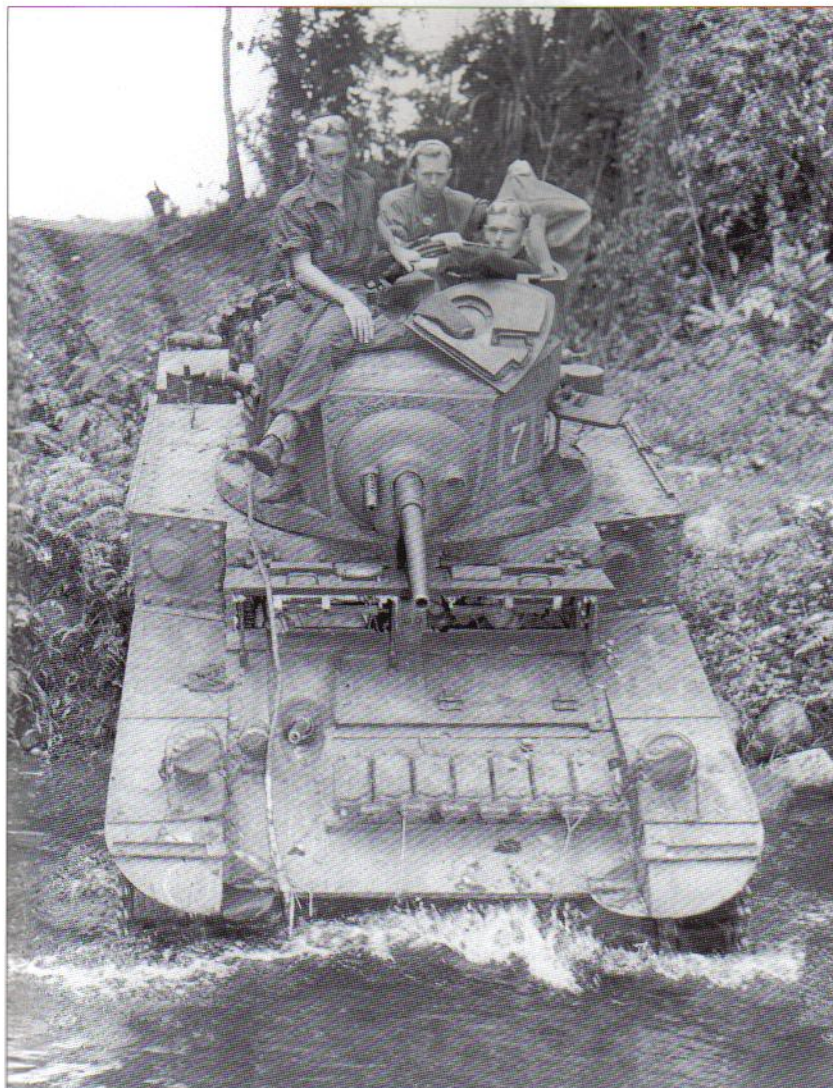
Australia began receiving Stuart light tanks via the British Lend-Lease allotments from the autumn of 1941. Before being introduced to combat in New Guinea, the vehicles were modified in Australian workshops, with the addition of a protective ring around the base of the turret to prevent the Japanese infantry from jamming it. This is a Stuart of the 2/6th Armoured Regiment during operations near Popendetta, New Guinea, on 19 May 1943. It uses the third turret type. (US National Archives)
