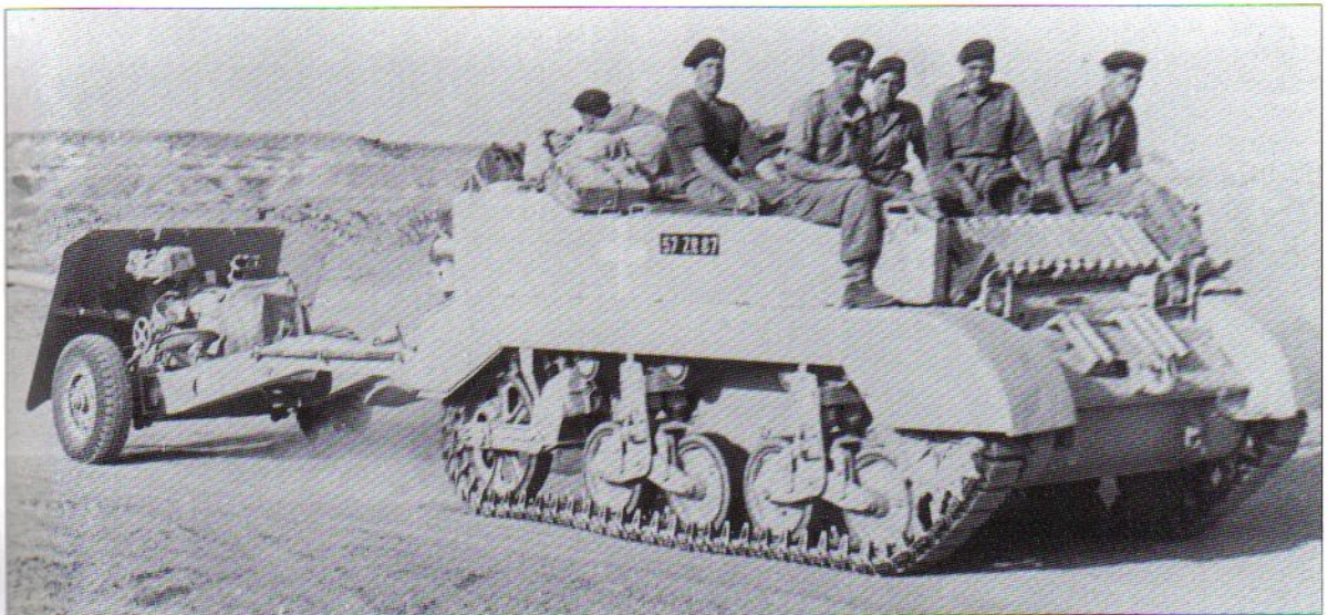
Although no longer in use as a tank, the British Army continued to use the Stuart in secondary roles after the war: this Stuart VI (M5A1) is used as an artillery tractor for a 17-pdr. anti-tank gun. (The Tank Museum)
