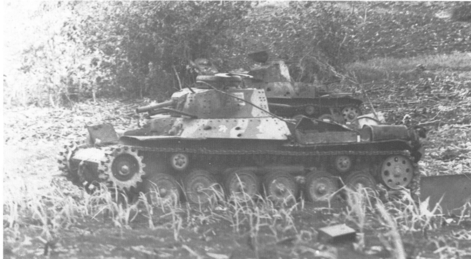
Before dawn of 16 June 1944 on Saipan, the 9th Tank Regt. launched the largest single Japanese tank counter-attack of the Pacific War; only 12 of 44 tanks committed survived the attempt. Photographed after the battle, a Type 97 Chi-ha (foreground) can be seen to have taken at least three 75mm hits; the ensuing fire has charred the kikusui turret emblem characteristic of this unit, but the 5th Co. insignia can still be seen—see Plate F2. In the background is a Type 95 Ha-go of the same unit. (US Navy)
