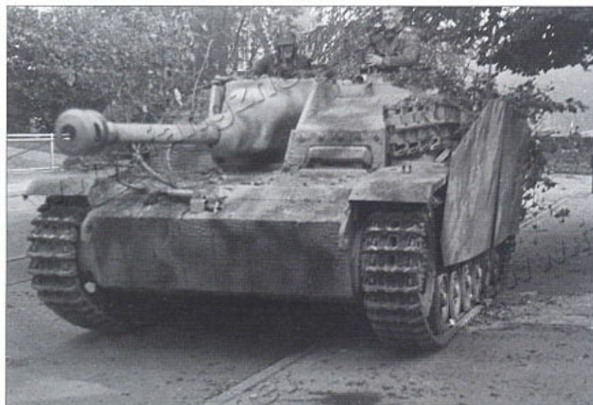
A Sturmgeschütz Ausf.G in Arnhem. This Sturmgeschütz Ausf.G. was completed in August 1944. The Rundumsfeuer machine gun is missing due to shortages while the coaxial machine gun fitted in the welded gun mantle from June 1944 did not appear in the cast mantle until October 1944. The Zimmerit coating was discontinued during September 1944. From August 1944 the camouflage was painted at the factory and at this period was intended to simulate light passing through foliage. (BA)
