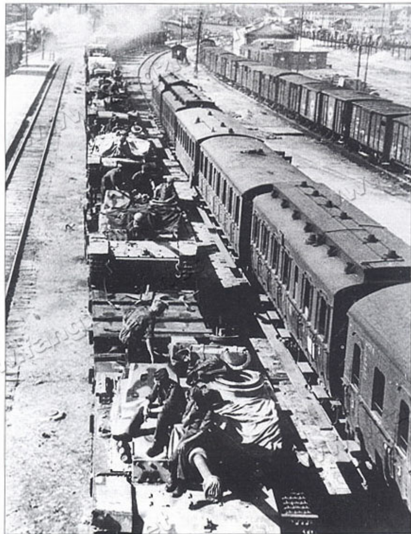
The Sturmgeschütz-Abteilung of SS 'Das Reich' being moved by train. The Sturmgeschütz nearest the cameraman has the solid 80 mm hull armour that was introduced in May 1943 but still has the smoke grenade launchers that were eliminated in the same month. (BA)
