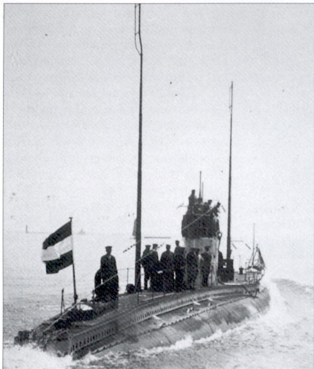
This vessel, seen from astern, is captioned on the original photograph as U-49. Her shape and configuration resembles more closely a UBIII type boat however. The wireless masts can be seen to good effect.
