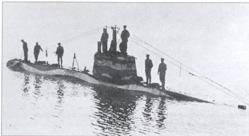
UB4, one of the early UBI Class boats. Note the disruptive camouflage pattern that has been applied to her hull and conning tower. These patterns were extremely effective.
