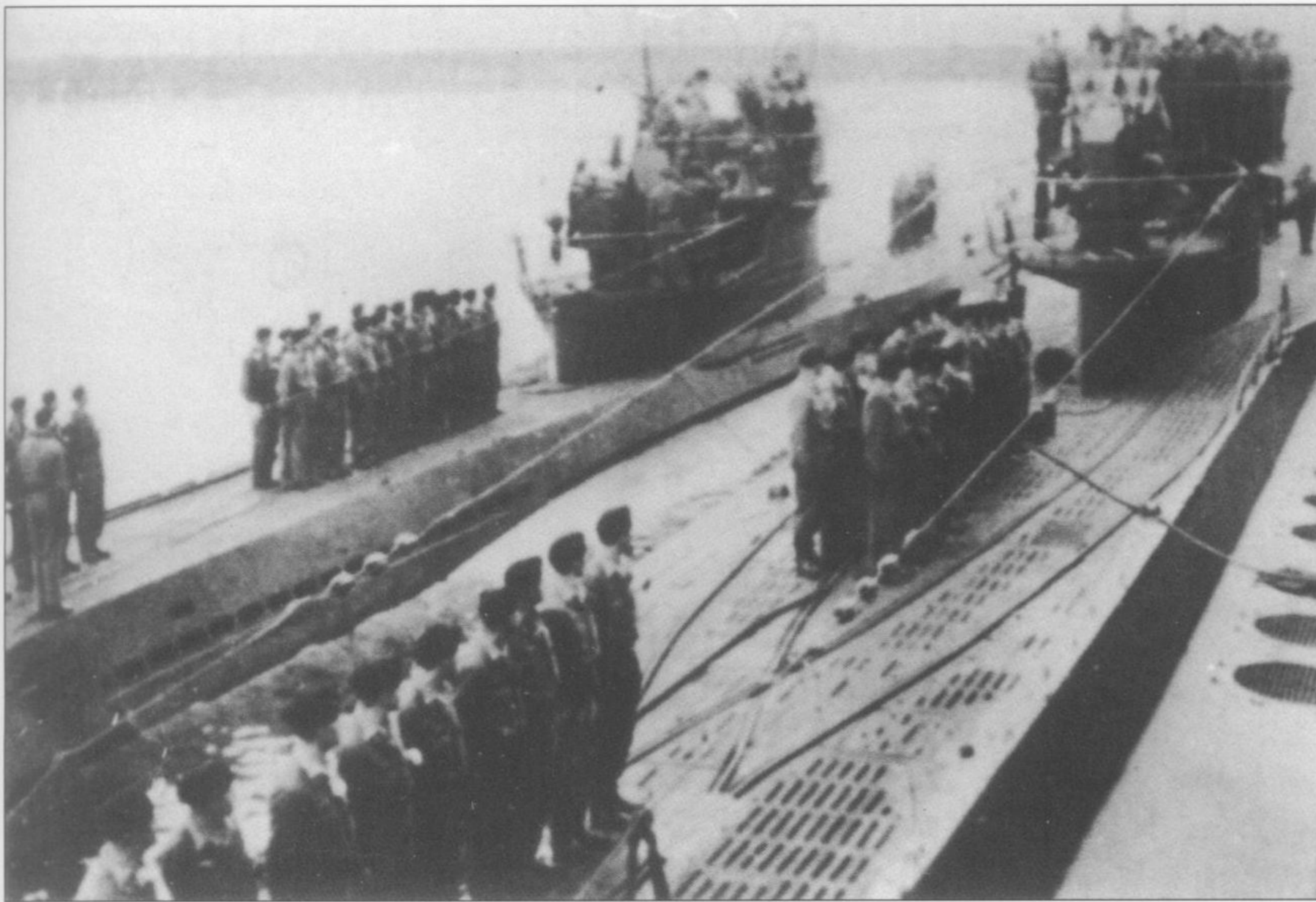
ABOVE At right on this shot is U-219, a Type XB minelayer. Its large size is apparent by comparison to the Type IX lying alongside. Note the rails on the decking to allow movement of mines.
