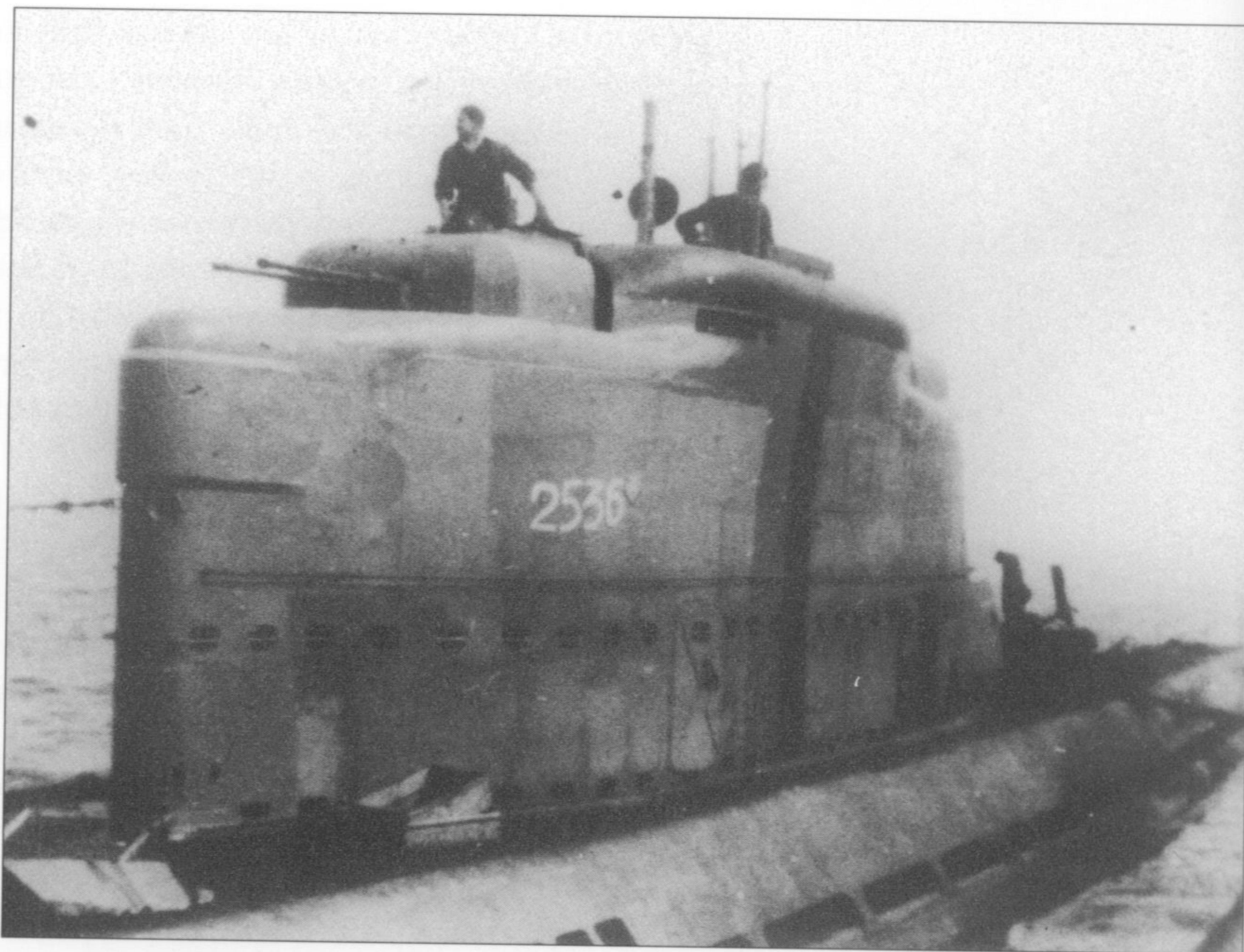
A view of the streamlined conning tower of a Type XXI, U-2536, under Oberleutnant zur See Ulrich Vöge. Note the forward twin 2 cm flak gun turret. This particular boat was still being worked up when the war ended and did not take part in any actual war patrols. It was scuttled on 3 May 1945.
