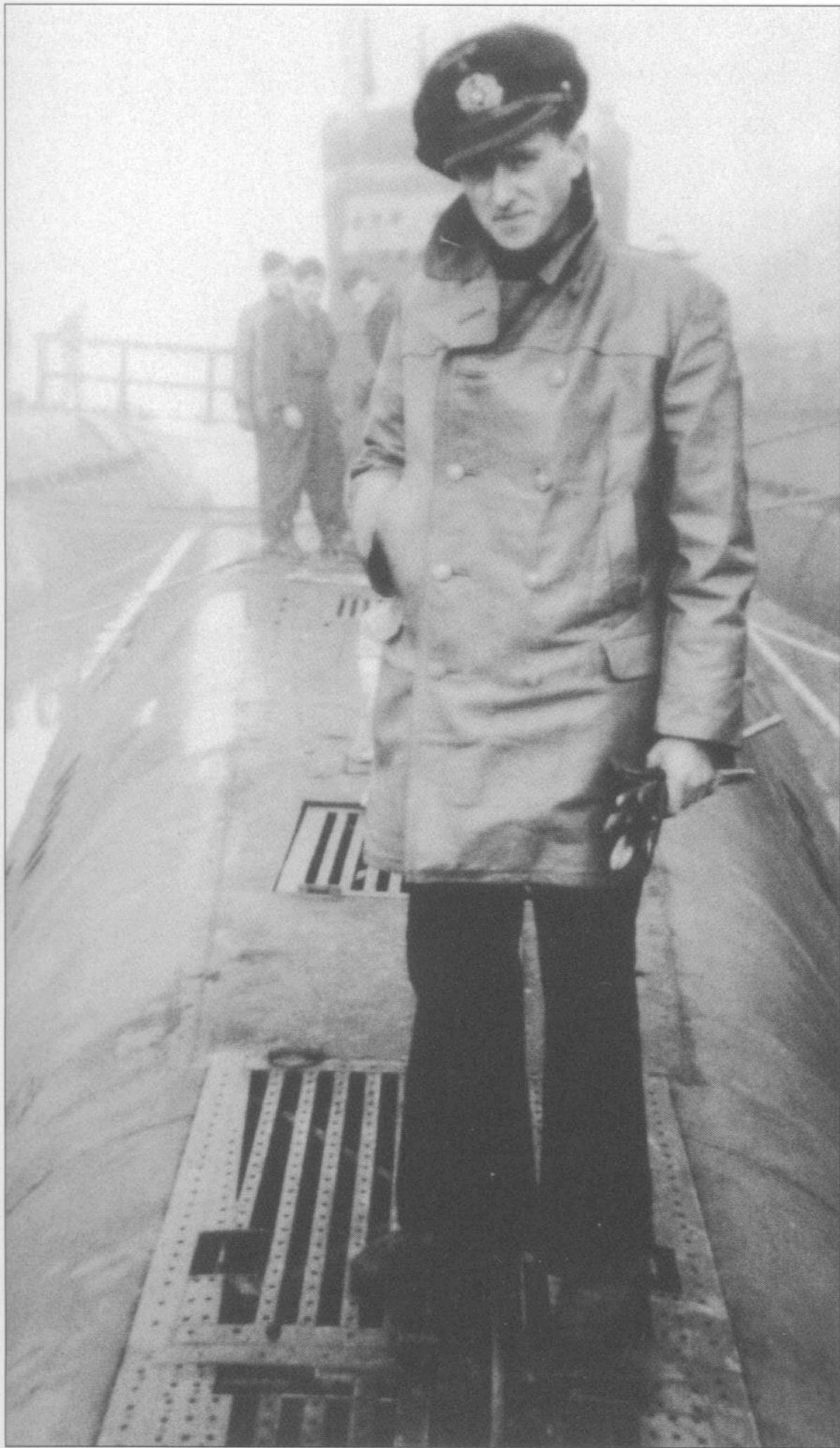
An officer from U-3022, a Type XXI, on the afterdeck. These boats were intended to spend most of their time under water, so no extensive deckworks were provided, just a narrow central walkway seen to good effect here.
