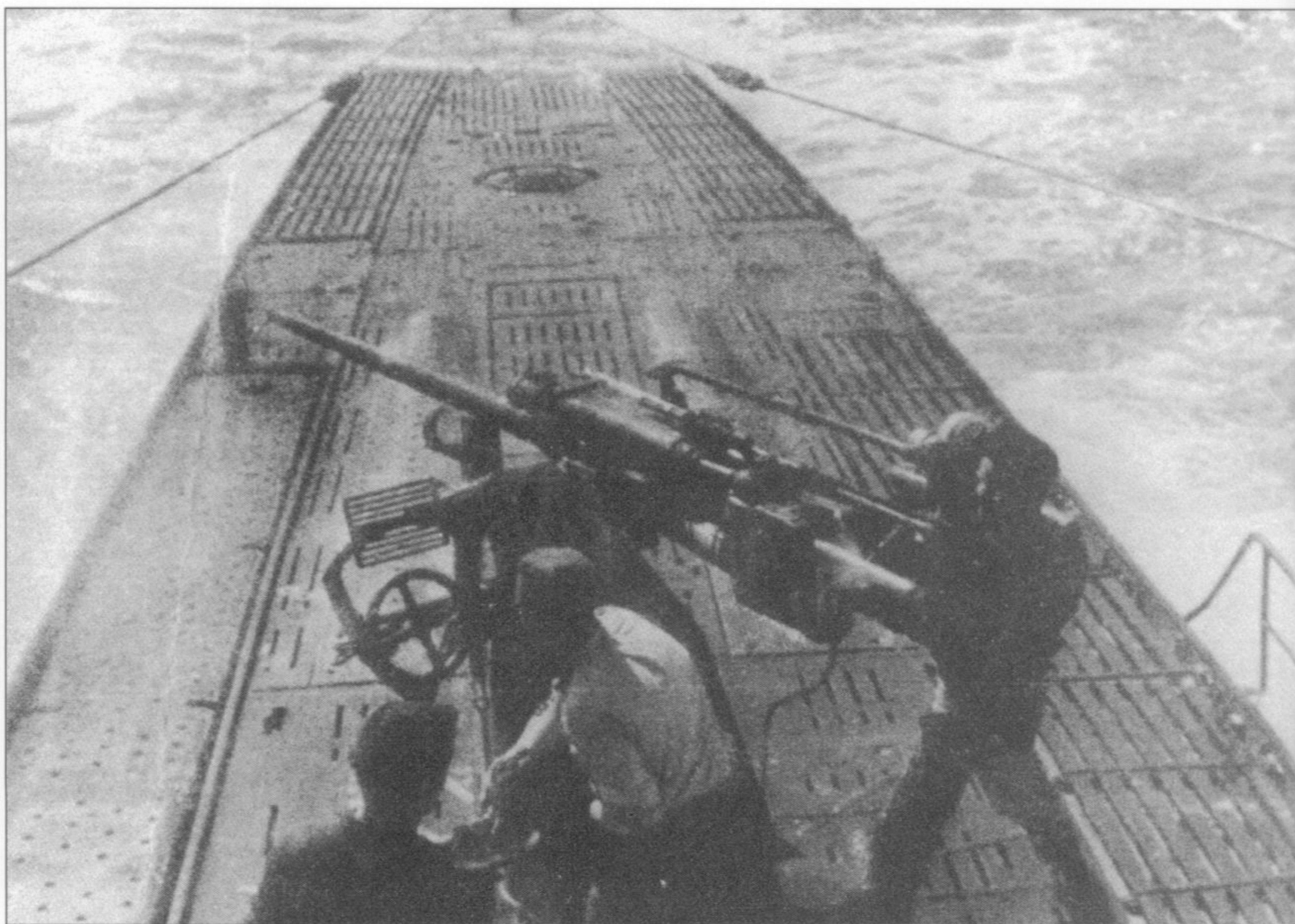
ABOVE Here we see the aft 3.7 cm flak gun, fitted to many early Type IX boats, in action. Later configurations had their flak armament concentrated on the conning tower platforms.
