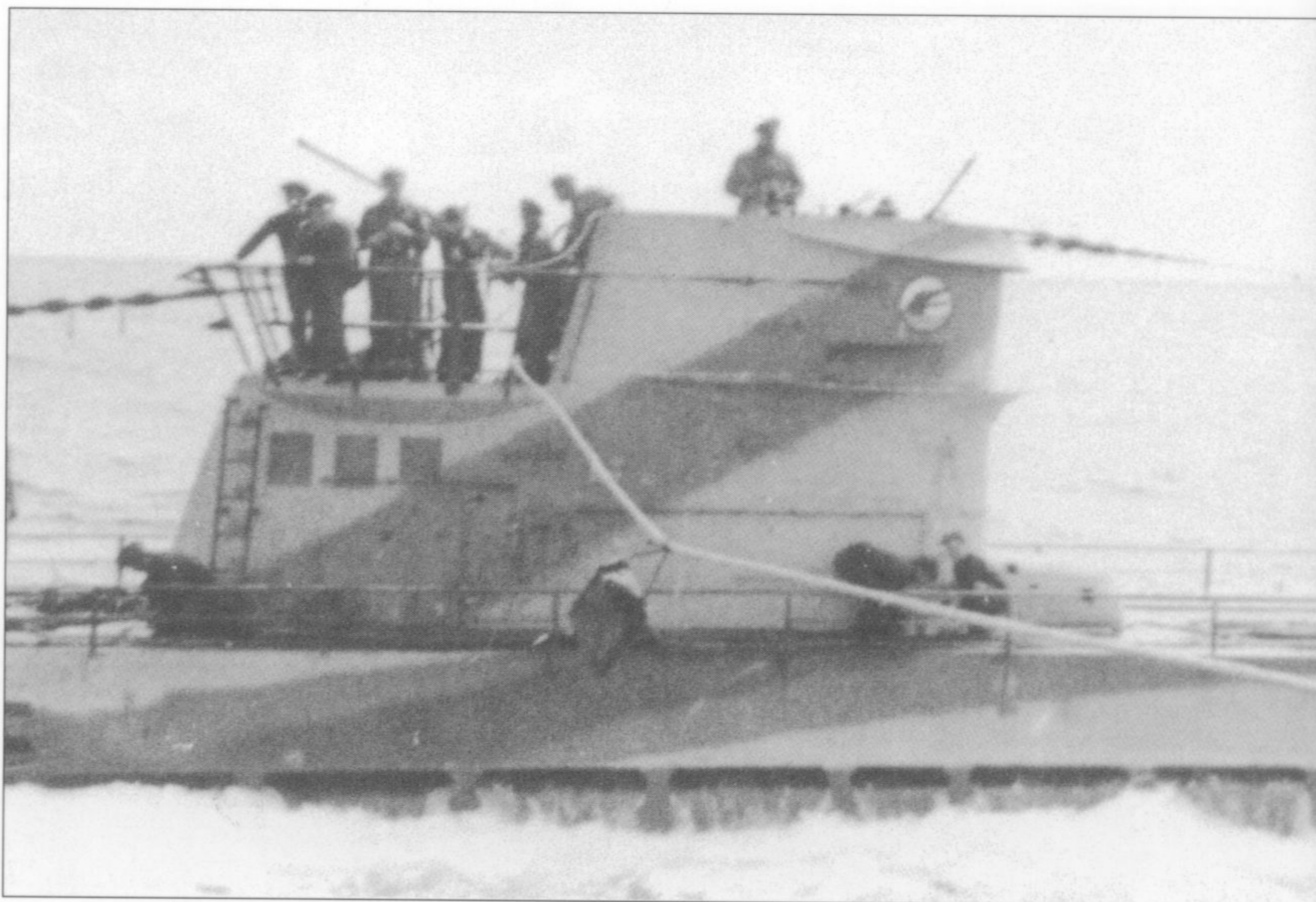
This is U-504, a Type IXC showing the early 'Turm 0' conning tower configuration with single platform. Note the unusual two-tone light/dark grey disruptive camouflage scheme.
