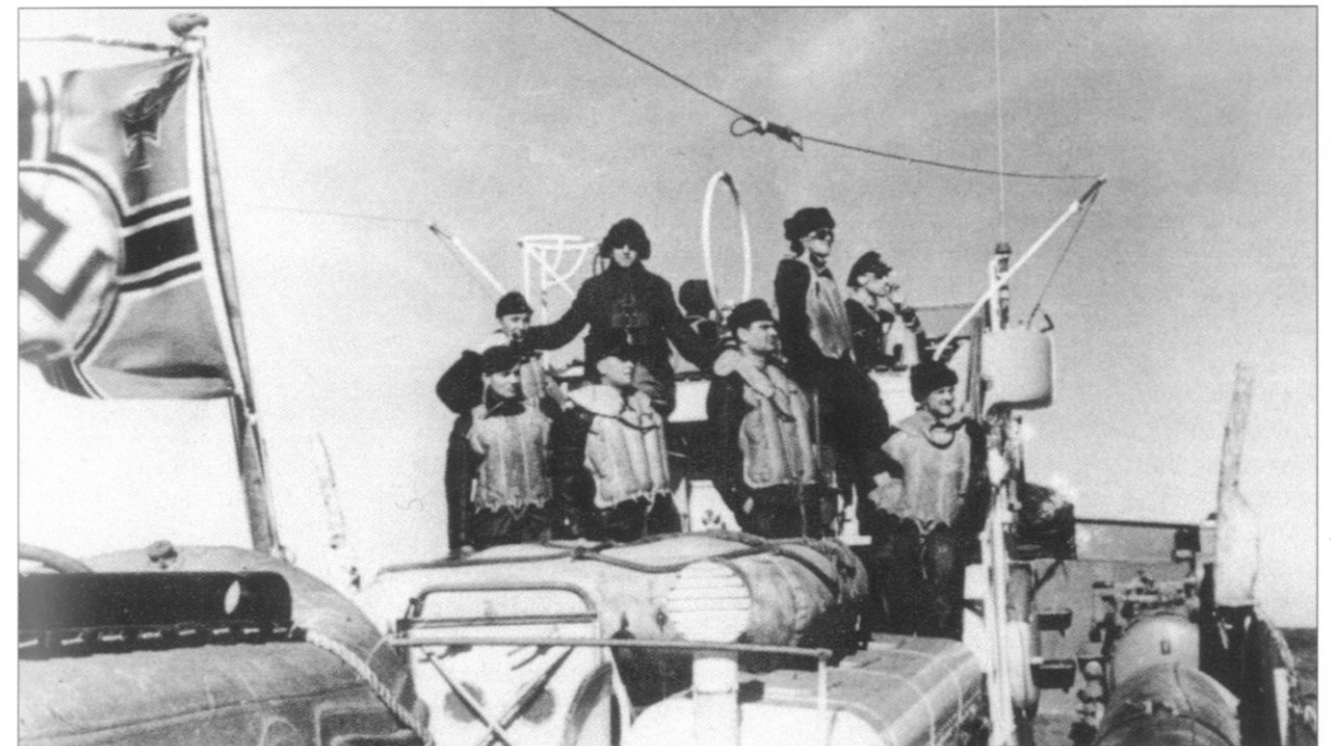
Looking up into the open bridge area from amidship. Note the large direction-finding loop. The standard large rubber dinghy is in the left foreground whilst on top of the forward engine room superstructure is a second, square inflatable life raft. This appears to have been taken on a bright winter's day, judging by the combination of fur hats and sunglasses being worn.
