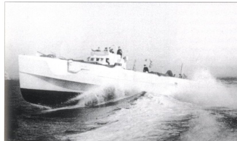
BELOW Port side view of a similar boat. The dark grey finish to the decking can just be seen on the foredeck, contrasting with the almost white vertical hull surfaces. This pale grey finish was established as being the most effective for such small, fast-moving boats.
