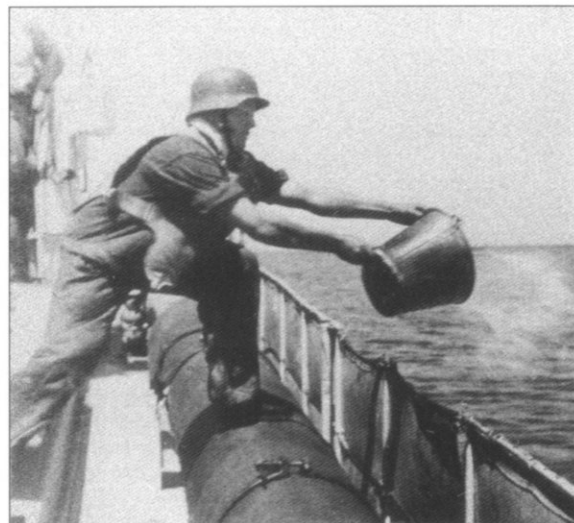
A steel-helmeted crewmember throws waste water overboard. This shot shows the spare torpedo on its rack. Note the retaining bands holding it firmly in place. Once again, this boat has the canvas dodger screens fitted.
