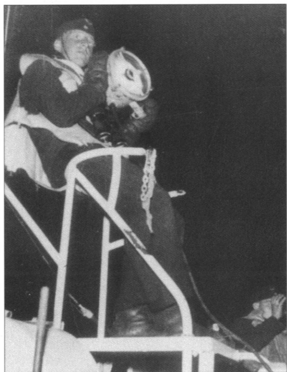
This view of the open bridge shows the small signal platform to the rear of the bridge structure, with its safety rail. Here the platform is occupied, during a night operation, by a sailor with a hand-held searchlight.
