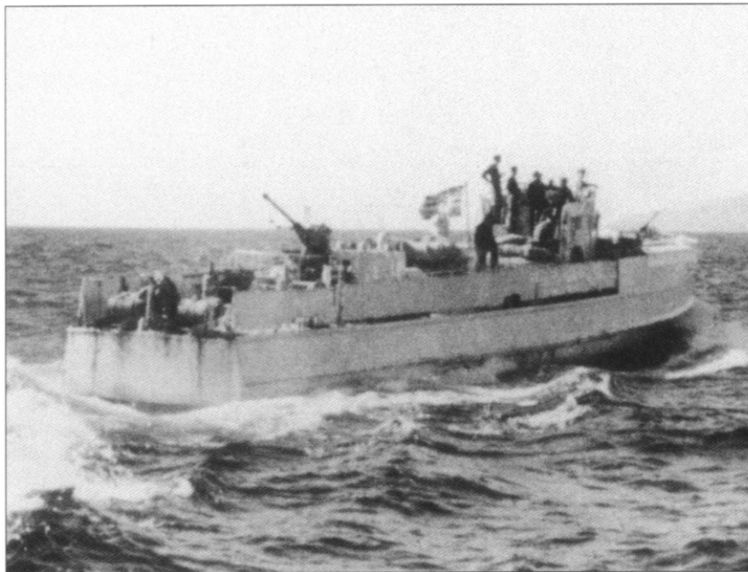
A stern view of an E-boat. Note that the canvas dodgers were only fitted over the side rails. Although this boat is clearly carrying depth charges, even when no depth charge racks were fitted, dodgers were not fitted over the stern rails. This boat carries a 4cm Bofors gun as its main stern armament.
