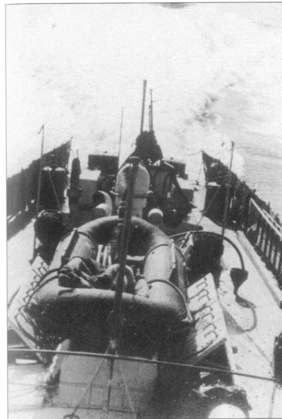
Looking astern from the bridge. Note the rubber dinghy on top of the superstructure above the engine room. The hatches are open to allow ventilation of this area. The weapon on the after deck appears to be a 2cm flak gun, going by the slender barrel.
