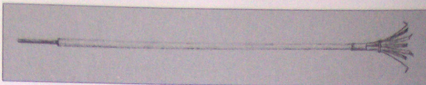
The searcher, the tool used for seeking out flaws in the metal of the gun bore. There is a ring near the base of the splayed head known as the reliever. This expanded or contracted the head when the tool was in use. (Courtesy RAHT)
