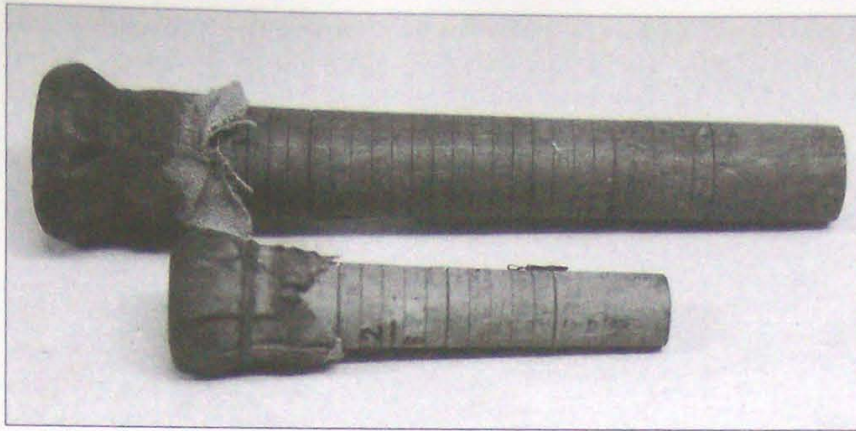
Two early fuses for howitzer shells. They still have the original cap covers, and the gradations into parts of a second corresponding to the time of flight are clearly seen. The gunner would cut the fuse to the required length. (Courtesy RAHT)
