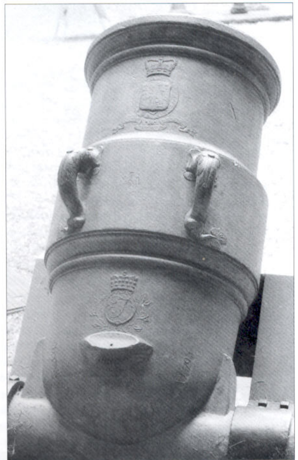
BELOW A 13-inch bronze mortar cast in 1779 and of the exact pattern used at the beginning of the Napoleonic Wars. The mounting is modern. The cipher of the Master General of the Ordnance, George Viscount Townshend, is moulded above the vent. (Courtesy of the Trustees of the Royal Armouries)
