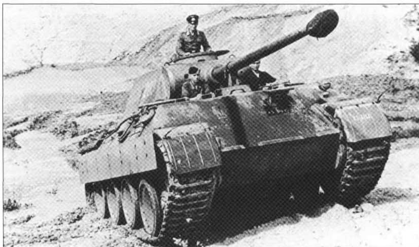
RIGHT This Daimler-Benz late Model D Panther, chassis number 211213, seen at the 15th Panzer Division training area at Sagan during autumn 1943, featured Schürzen skirting plates mounted on the side of the vehicle to protect the track and hull sides from enemy fire. (The Tank Museum, 341/H6)
