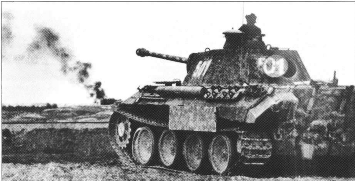
ABOVE Model A Panther, number 501, engaged in combat in the East during early 1944. As often occurred, the tank has lost some of its Schürzen plates, probably due to damage by enemy fire. (The Tank Museum, 4704/C3)
