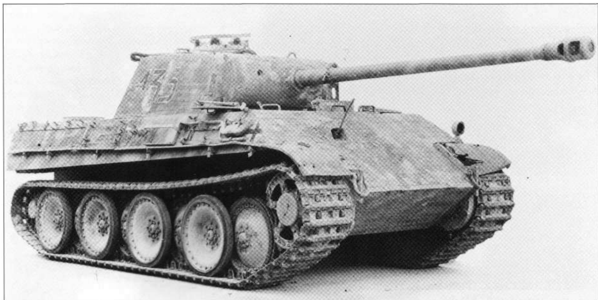
Early Model G Panther number 435 sports the ripple effect left when the tank was coated with Zimmerit anti-magnetic mine paste. After September 1944, however, German factories stopped applying the paste after post-combat reports alleged that the Zimmerit caught fire when enemy rounds hit the tank. (The Tank Museum, 6087/C6)
