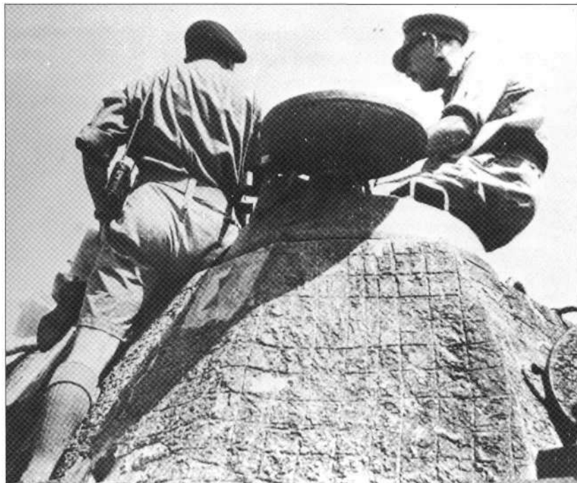
This close-up view of the rear left side of a Panther turret underneath the commander's cupola reveals the uneven texture left by Zimmerit paste. The vehicle has been captured by British forces, who are here inspecting their prize. (The Tank Museum, 2903/C1)
