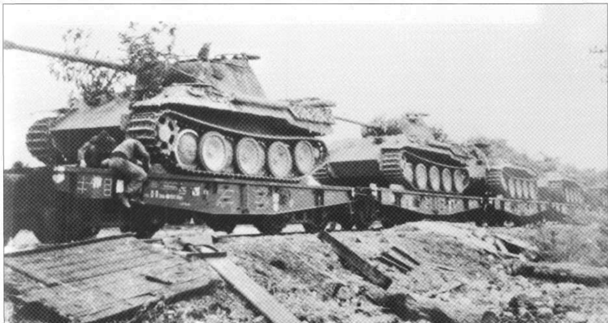
Mid-production Model A Panthers being transported by rail to the East in early 1944. The crew of the lead tank have fitted spare track sections to the vehicle's rear hull sides, although increasingly crews mounted these sections on the tank's turret sides to further protect this crucial part of the vehicle. (The Tank Museum, 4704/C4)
