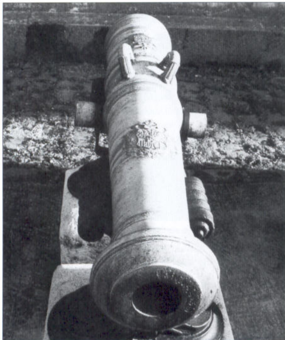
A 6-pdr barrel. Two surviving examples from the 1760s show a discrepancy of 6cm (2.3 Zoll) in length. The trunnions were 3.44 Zoll in diameter and this 1761 example has the older style, elaborate handles.
