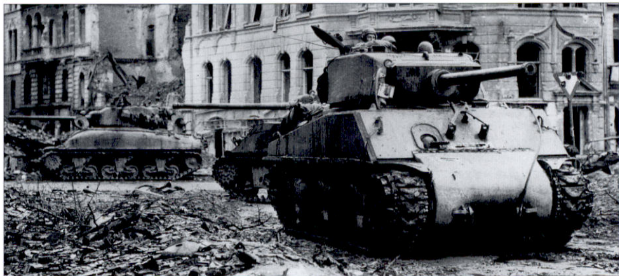
Although the plan to re-arm 75mm M4 tanks was abandoned, the gun tubes that were collected were used to re-arm most of the surviving M4A3E2 assault tanks. This M4A3E2 of the 32nd Armored Regiment, 3rd Armored Division, is seen in the ruins of Cologne during the fighting for that city in March 1945. (NARA)
