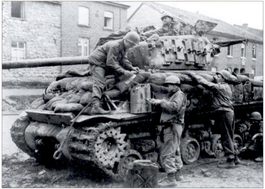
Early attempts at improving the armor on the M4A3E8 (76mm) were improvised from sandbags and spare track blocks. This is a tank of Co. A, 18th Tank Battalion, 8th Armored Division, at Bocholtz, Netherlands, on February 23, 1945. (USMA)
