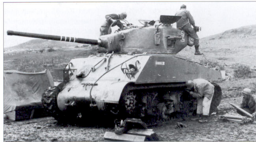
The M4A3 (76mm) that served with the 1st Armored Division in Italy had their own local modifications made. Many of the Division's tanks had a “donkey sight” added on the right front turret roof that was used for gun laying when the tank was being used in the indirect fire artillery role. This is very evident as a pair of semi-circular metal hoops were welded on either side of the sight to protect it. This tank, named Somme IV, belonged to the 4th Tank Battalion and is seen near St Lucia on October 19, 1944 prior to the attack on Bologna. (US Army)
