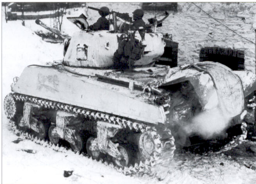
A snow-camouflaged M4A3 (76mm) of the 750th Tank Battalion moves through Salmchateau, Belgium, while supporting an attack by the 75th Division on January 16, 1945 during the Ardennes fighting. Once the ground froze hard in late December 1944, extended end connectors for the track were no longer needed and are absent on this tank. (US Army)
