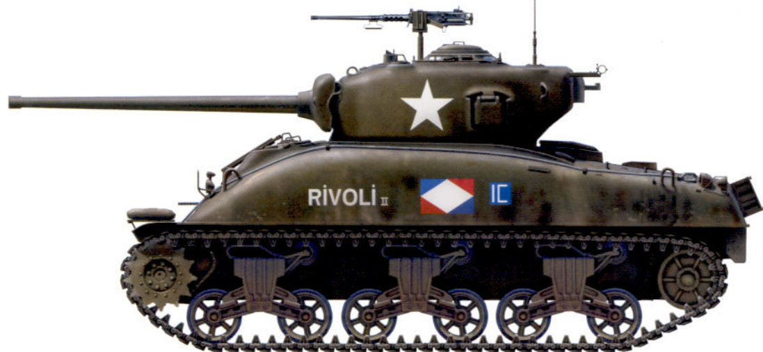
C1: M4A1 (76mm), 2e Regiment de Chasseurs d'Afrique, French 1st Armored Division, Germany, April 1945
