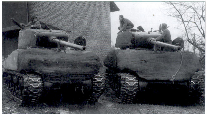
Ordnance units of the Ninth Army developed an armor appliqué consisting of a steel track welded to the armor, covered with sandbags, and with a final cover of camouflage net as seen on these M4A3 (76mm) of the 747th Tank Battalion near Schleiden, Germany, on January 31, 1945. (NARA)
