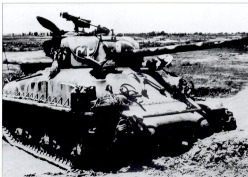
Among the MDAP clients for the M4 conversions was Pakistan, which received both the M4A1E4 (76mm) as seen here, as well as the M4A3E4 (76mm). This particular tank served with the 26th Cavalry Regiment. (George Balin)
