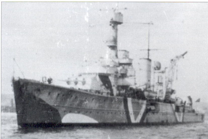
Köln is shown here wearing her so-called 'Baltic' camouflage in 1941. Note the dark area at the bow and the white-painted false bow wave. The broad black/white bands were painted across the hull and up over the superstructure.
