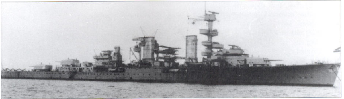
An excellent later (though still pre-war) shot of Köln . Note the searchlight platforms on the derrick towers and the addition of the pole mast to the rear face of her second funnel. The number of platforms on her battlemast has been reduced.
