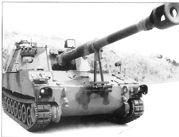
Germany's M109A3G introduced a lengthened 155mm cannon which can be easily distinguished from its American counterpart by the different muzzle brake. Many other German improvements are evident, such as the driver's mirrors, new track, and smoke mortar dischargers. (Rheinmetall)
