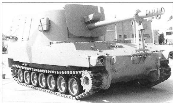
One of the more unusual vehicles built on the M109 chassis was the Egyptian SP122, which used Egyptian-manufactured copies of the Soviet D-30 howitzer instead of the usual 155mm howitzer. (Christopher Foss)
