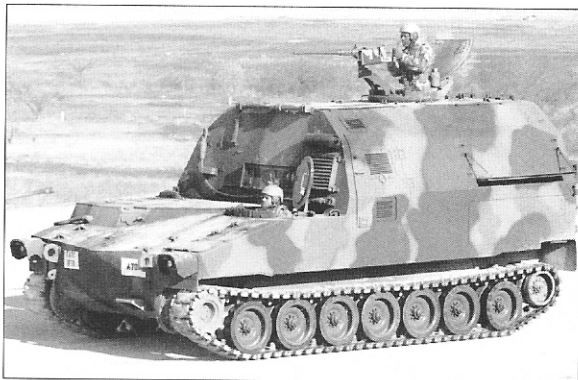
An M992 FAASV of Battery A, 1-78th Artillery, at the Field Artillery Training Center at Ft Sill, Oklahoma, painted in the standard NATO three-color scheme. (Author)
