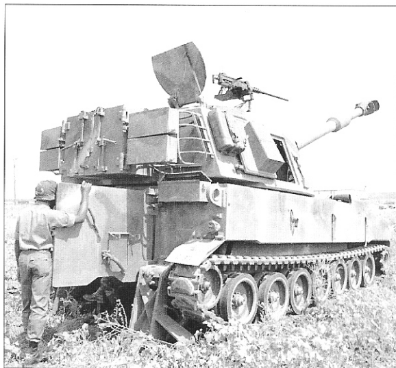
This rear view of an M109A2 of Battery C, 1-3d Artillery, 2d Armored Division, Ft Hood, Texas, shows the distinctive change of the M109A2/A3 upgrade: the extended bustle rack in the center of the turret rear that permitted more ammunition to be carried. This photo also shows the recoil spades extended for firing. (Author)
