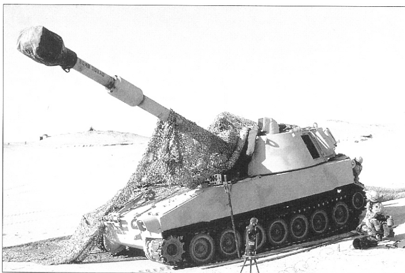
The ballistic cover over the gunner's sight is clearly visible on this M109A2/A3 during the joint US-Egyptian Bright Star exercises in 1982. The M109A2 was the new-construction vehicle, and the -A3 the upgraded model, and they are impossible to distinguish externally. (US Army)
