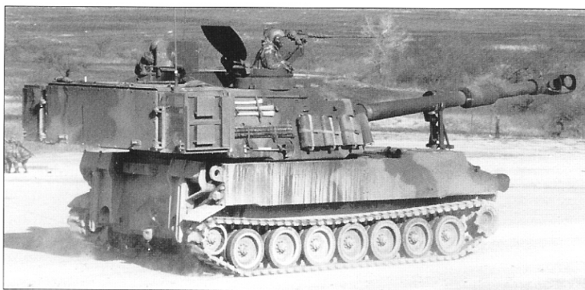
Another view of an M109A6 Paladin at the US Army Field Artillery Training Center at Ft Sill, Oklahoma, showing the much larger rear turret bustle on this version. (Author)
