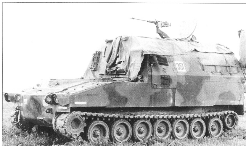
An important innovation in artillery tactics in the 1980s was the adoption of the M992 FAASV artillery supply vehicle based on the M109 chassis. This example is from Battery B, 4-82d Artillery of the 3d Armored Division, seen during a Reforger exercise in the 1980s. The tactical number on the side in a blue rectangle indicates it was part of the "Blue" forces during the wargame. (Pierre Touzin)
