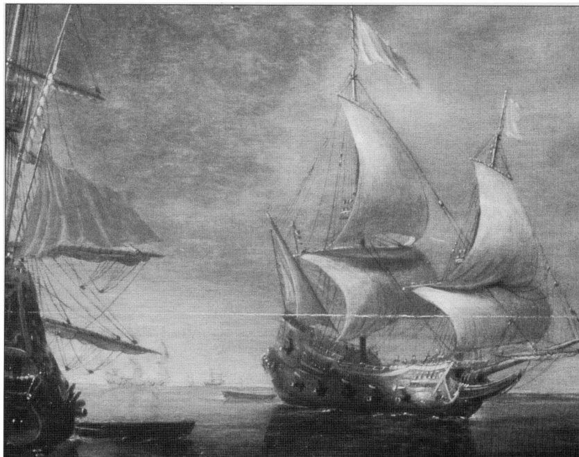
Despite purporting to be a vessel from the Barbary coast, this vessel is clearly a small Spanish galleon. Her appearance is typical of the 400- or 500-tonelada galleons which made up the bulk of the escort vessels assigned to guard the Indies flotas during the early 17th century. An Algerine ship off a Barbary Port ; oil painting by Andries van Eertvelt. (National Maritime Museum, Greenwich, London)
