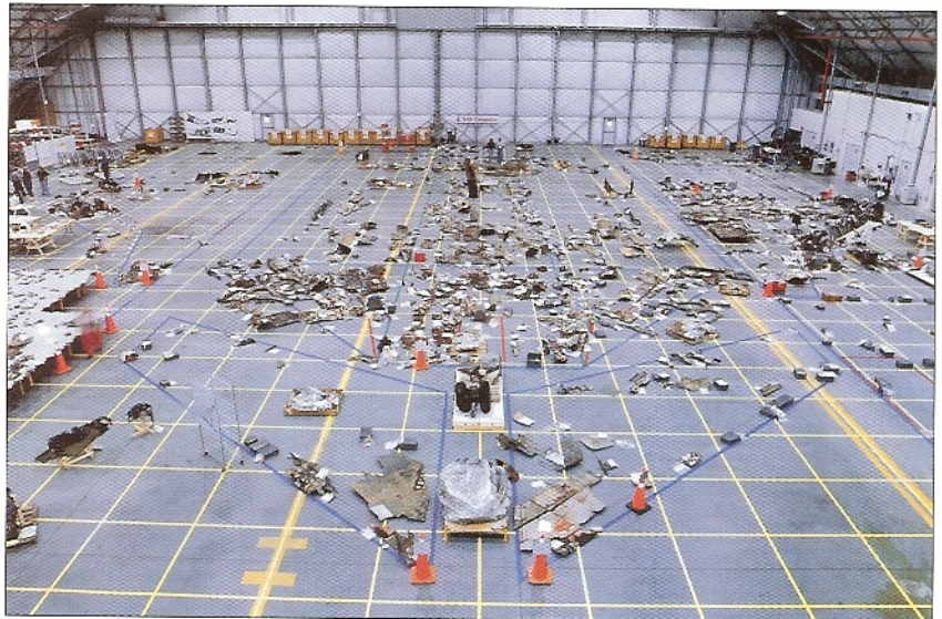
RIGHT All that remains. Recovered debris from Columbia in a hangar at KSC. Following the loss of Columbia in February 2003, NASA scoured the Texas countryside for pieces of the Orbiter as part of the effort to determine what caused the breakup.
