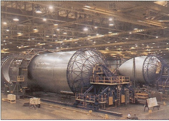
An External Tank under assembly in what was then the Martin Marietta Aerospace factory in Michoud, LA. Today, this plant is run by Lockheed-Martin.
