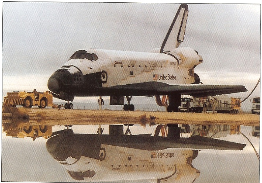
Columbia at Edwards AFB being towed to the Shuttle Processing Area at NASA's Dryden Flight Research Center following landing on STS-5. Orbiter landing servicing vehicles can be seen behind the Orbiter, while a tug pulls the Orbiter.
