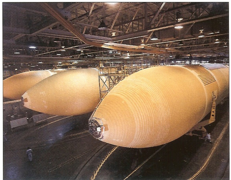
Three completed lightweight ETs at the Michoud assembly plant awaiting delivery to KSC in 1981.
