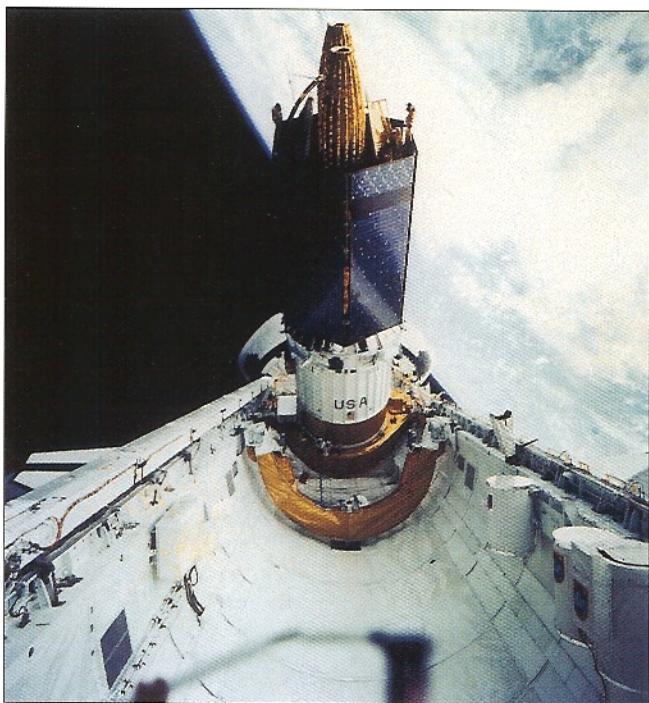
Deployment of a TDRSS satellite from the Orbiter. A spring-loaded platform in the harness holding the satellite in the cargo bay pushes the satellite out of the Orbiter. An IUS upper stage (white portion on bottom) then boosts the satellite (gold and black upper portion) to a geostationary orbit.
