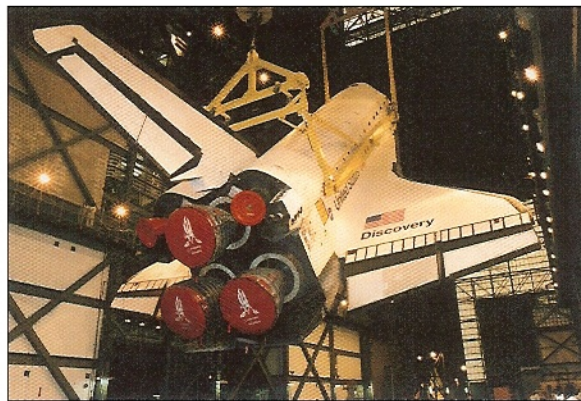
In the Vehicle Assembly Building, Discovery is being lifted in preparation to being mated with the External Tank for STS-95.
