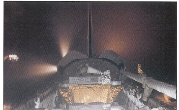
The Orbiter is controlled in space with using a 44-jet Reaction Control System. Here, two aft primary RCS jets can be seen firing.
