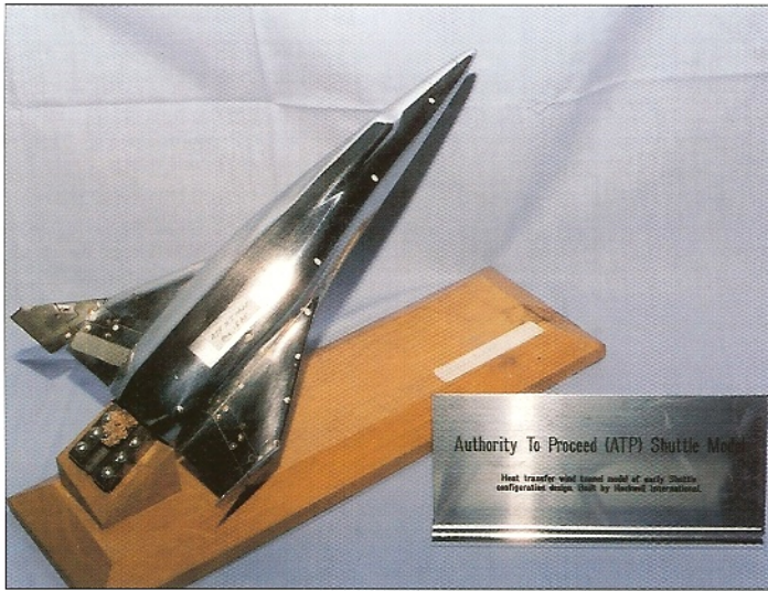
By Authority to Proceed, the Orbiter design had evolved to a double-delta wing, but one with twin rudders, raised wing tips, and jet engines for landing. This was a heat transfer model of the design used by Rockwell to refine the craft. (Author's collection)
