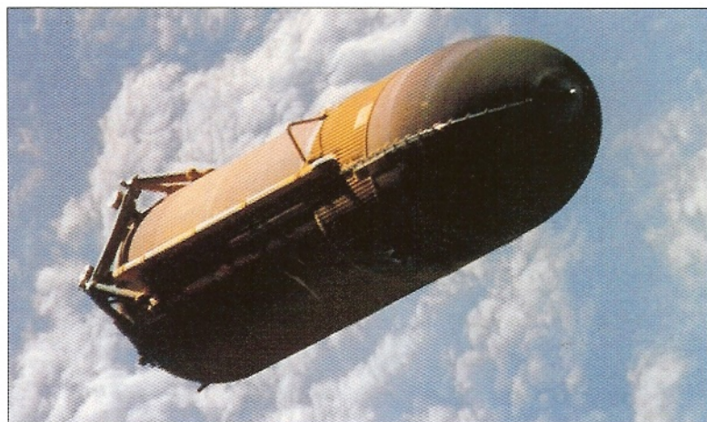
BELOW The External Tank photographed drifting back to Earth after a successful ascent in 2002.
