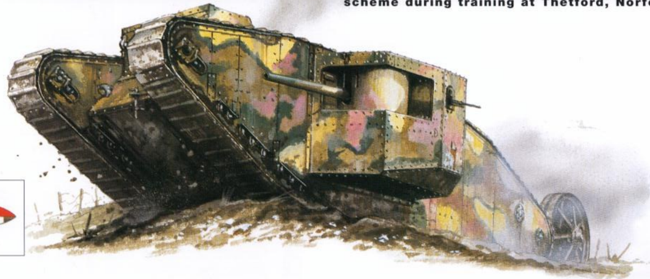
C1: A Mark I (Male) tank in the original camouflage scheme during training at Thetford, Norfolk
