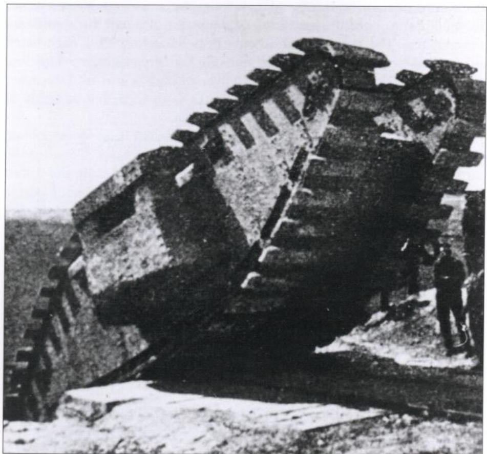
A poor but rare photo of a Female tank, fitted with special climbing spuds, tackling a mock sea wall during training for Operation Hush. This climb must have been a driver's nightmare. Had the operation gone ahead Mark IV tanks would have been employed.
