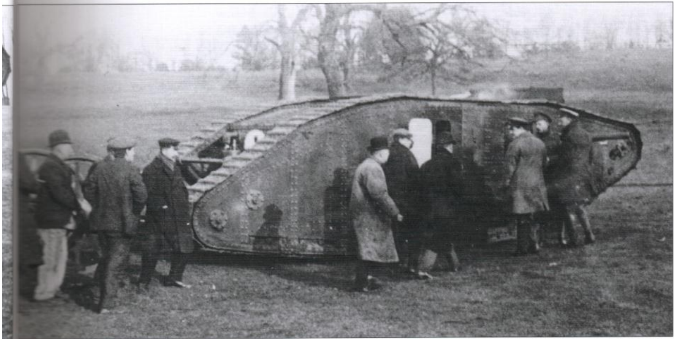
he Tritton, Wilson and Stern are p among the group gathered to around Mother's starboard n sponson. Notice how the door e swings outwards but against the hull. The small, oval door at the rear is also open and can just be seen over the tracks.
