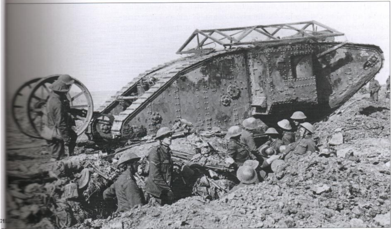
Another classic photograph; C15 moving up for the attack on Thiepval on 26 September 1916. The tank is thickly plastered at the front and seems to have utilised much of the camouflage. The tank is running with its tail clear of the ground, the gun on full elevation and steam shut.
