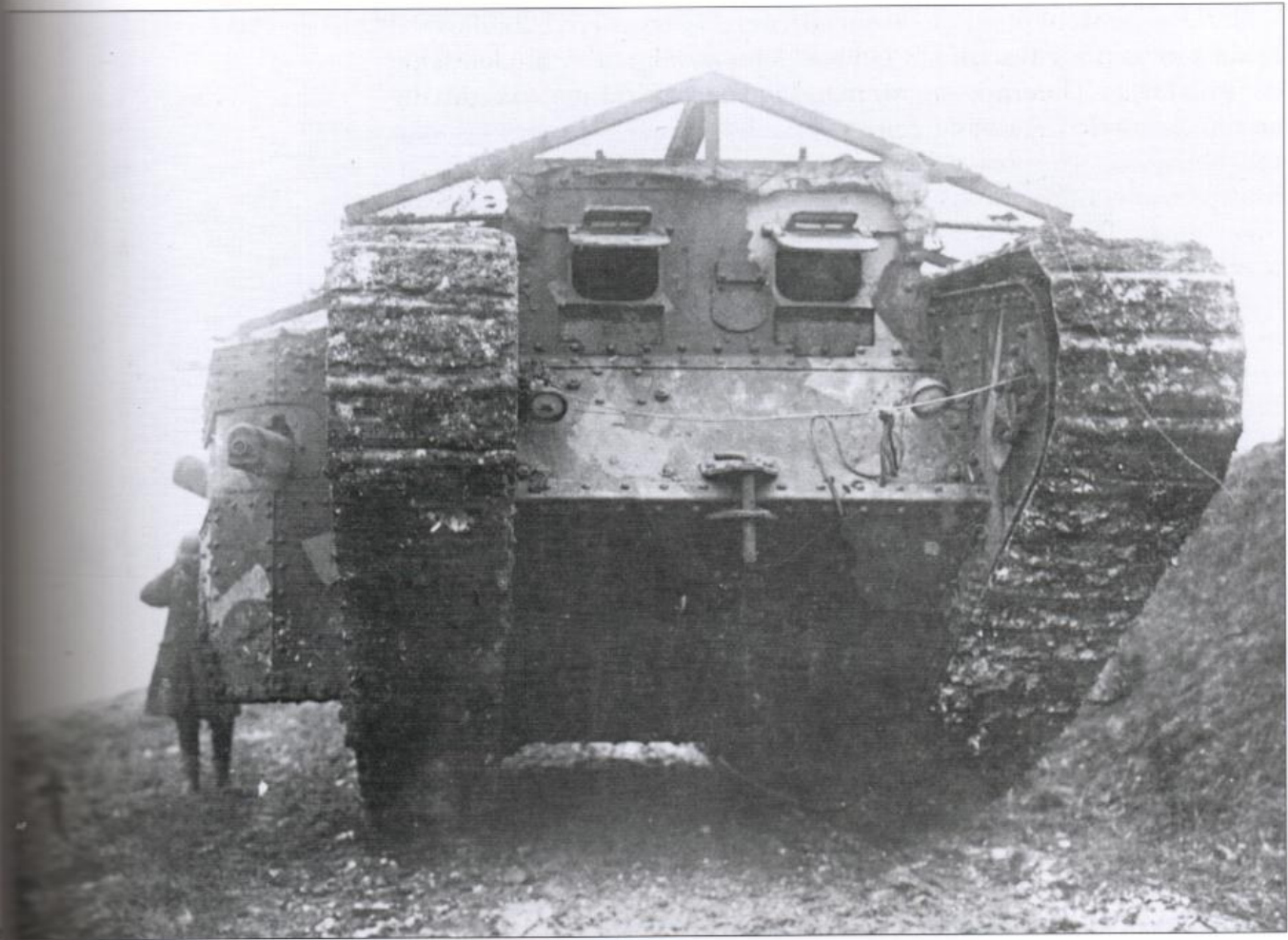
Close-up frontal view of a female Mark I, probably of A Company during the November 1916 actions. This company also employed the grenade-proof roof, but this one seems to have an extension over the top of the turret, which would make sense.
