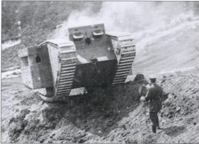
BELOW An excellent view of a Mark III Female with the smaller Lewis gun sponson. The escape hatches below the sponson are wide open and the two rotating shields for the machine guns have been turned to face inwards. Notice also the clevises, or hooks, at each end of the sponson for lifting it off.
