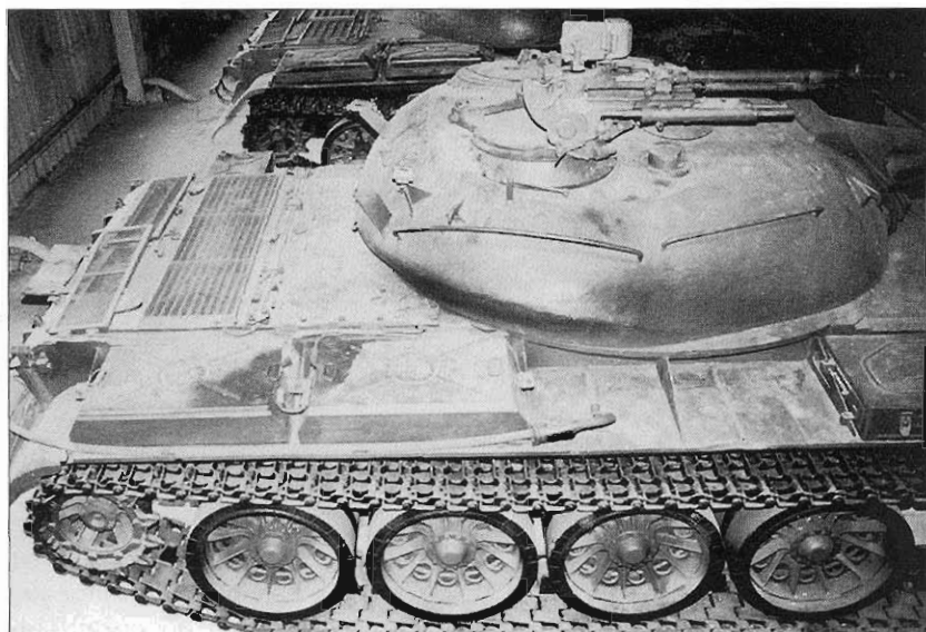
This overhead shot shows several of the distinctive features of the T-54-2 tanks, notably the overhang at the rear of the turret. It is also noteworthy since it is still fitted with the original welded external fuel cells. By the mid-1950s, these gave way to the more typical stamped fuel cells. (S. Zaloga)
