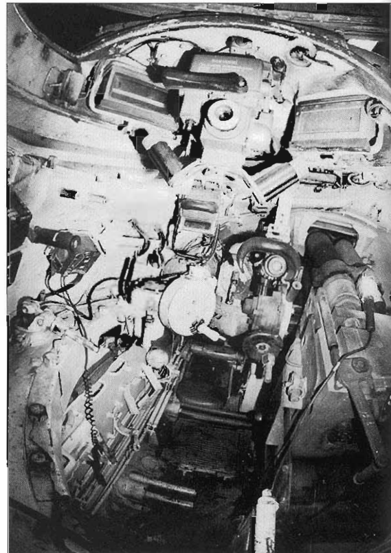
A view inside the T-54A from the commander’s station looking forward towards the gunner’s station. The driver’s seat has been removed, so it’s possible to see the driver’s seat, which in this case has its backrest folded back. The large breech of the D-10T gun is evident to the right and the gunner’s telescopic sight is towards the center of the photo along with the various traverse and elevation controls. (S. Zaloga)
