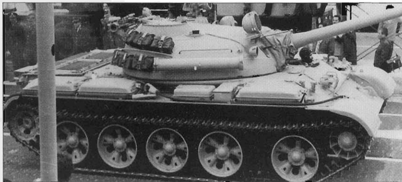
The final production T-55 tanks intended for export had all of the changes of the T-55A, but lacked the anti-radiation lining. Several features were distinctive including the stowage of the OPVT snorkel on the right turret side, the 12.7mm machine gun combing, the added 12.7mm ammunition stowage on the right turret rear, and the provisions for stowing the 12.7mm machine gun on the turret rear. This is a Peruvian T-55 on parade in Lima in the 1980s. (US DoD)
