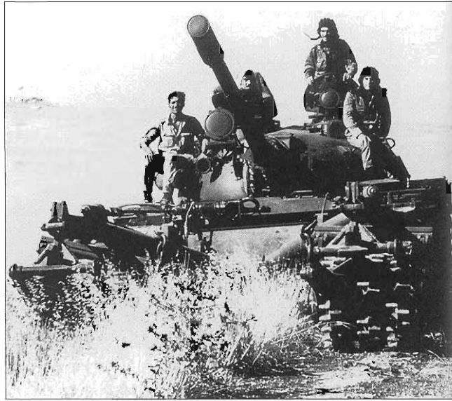
The most common of the T-55 mine trowls was the KMT-5 system. This Syrian T-55 was photographed on the Golan Heights in the wake of the 1973 war after the UN-sponsored ceasefire. (UN)
