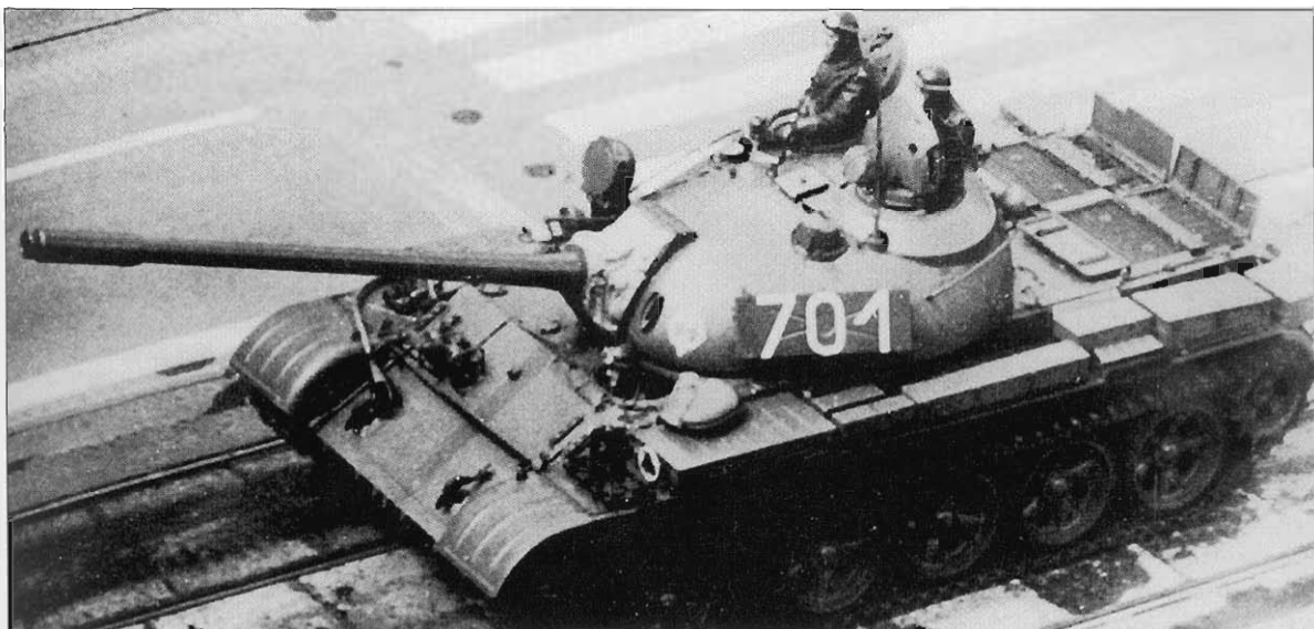
The T-55 tanks manufactured in Poland and Czechoslovakia had many small detail differences from the original Soviet design. The Poles fitted an extra ZIP tool stowage bin on the left side of the turret, and the fan door on the right rear corner of the hull has a distinctive notched shape instead of the rectangular shape of the original Soviet design. This Polish T-55A shows the distinctive features of this version such as the prominent combing around the turret hatches which contained a protective anti-radiation lining. (US Army)
