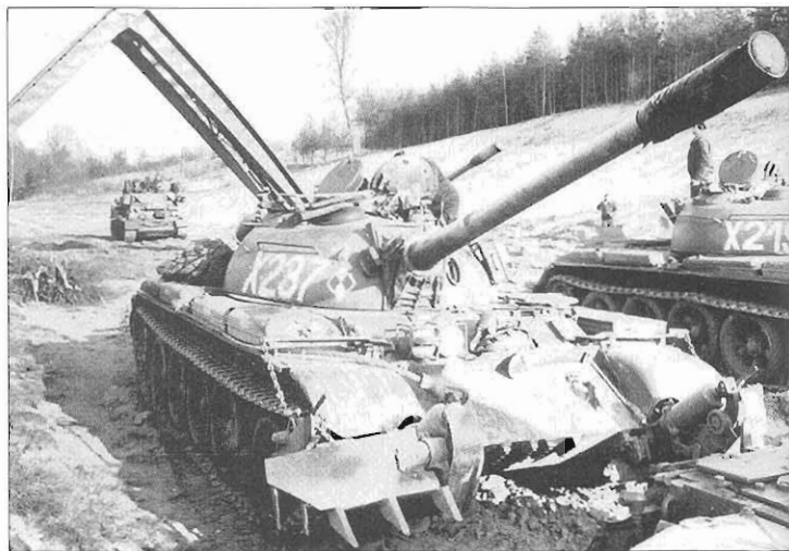
The KMT-4 mine rake was used to rapidly breach a minefield by scooping up mines and pushing them to one side. This Polish T-54A is fitted with the KMT-4 and behind it are some other engineer support vehicles including a BLG-60 bridge-layer and a WPT-34 armored recovery vehicle. (Janusz Magnuski)
