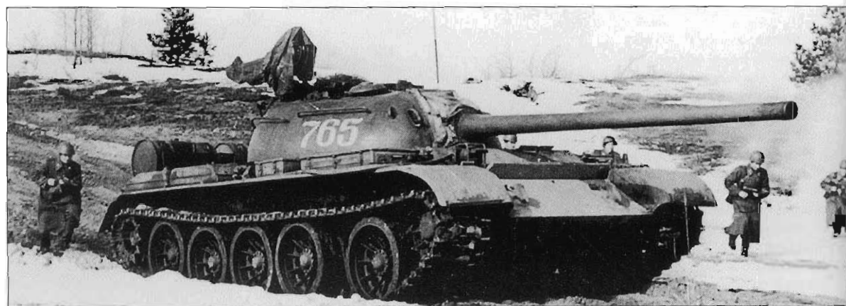
The T-54-3 was the definitive version of the early T-54 series, debuting the standard turret shape. This is a relatively rare view of a production tank prior to rebuilding with the original spider wheels and the single front headlight.
