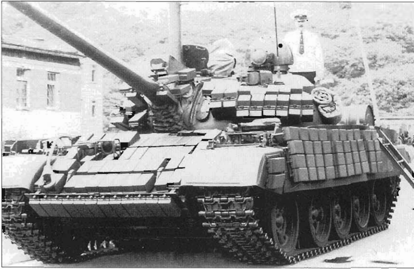
The T-55AMV incorporates the Kontakt explosive reactive armor instead of the passive "brow" armor of the T-55AM. This example displays the other upgrades including the 1K13 gunner's sight for use of the Bastion guided projectile, the new RMSH tracks, and the KTD-2 laser rangefinder. It is seen here in service with a Soviet Naval Infantry regiment in the 1980s. (US DoD)
