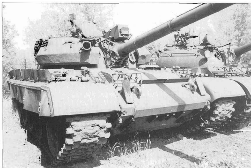
The T-55M/AM program aimed at a deep modernization of the T-55 series. This particular example is a tank sold to Poland that formed the basis for its T-55AM-2 upgrade program. It shows some of the distinctive elements of the program, such as the "brow" armor, KTD-2 laser rangefinder, side skirts, Tucha smoke mortars, and thermal sleeve for the 100mm gun. (S. Zaloga)
