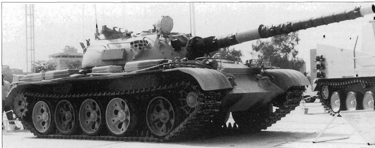
An Egyptian requirement for a large-scale upgrade of its T-55 fleet led to many foreign competitors developing modification kits. This example by Britain's Royal Ordnance substituted the NATO-standard 105mm gun and included many fire control improvements. (C. Foss)
