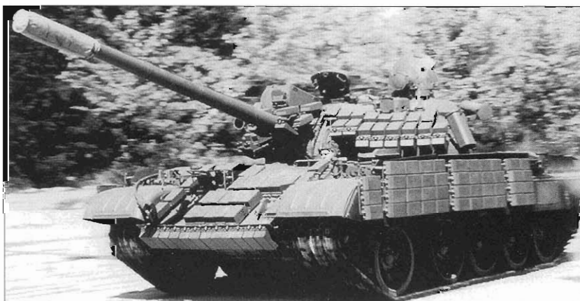
Ukraine was the center for many of the T-55 rebuilding efforts, including the T-55AMV tank with Kontakt reactive armor. This is an example with the full suite of Kontakt reactive armor in place. (Ukrspetsekспорт)
