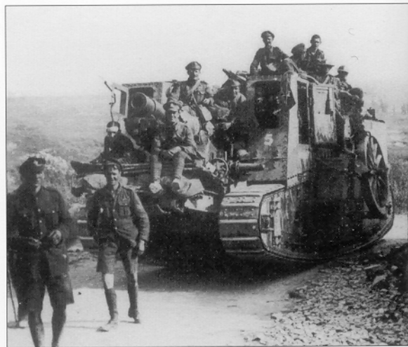
Gun carrier Dublin transporting a BL 6-in. 26cwt howitzer, its ammunition and detachment. Irlles, the Somme, 25 August 1918. (IWM Q61069)
