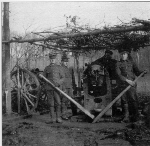
BL 6-in. 30cwt howitzer of 6th Siege Battery, RGA, 1914–15. The ammunition wagon has been placed alongside the howitzer, which is mounted on its siege platform. The detachment is posing with handspikes. The overhead camouflage screen is typical of British World War I siege artillery positions. (RAHT AL190.3.27)
