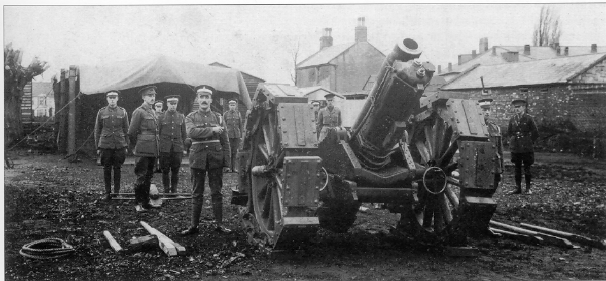
BL 6-in. 26cwt howitzer at the Officer Training Establishment, Trowbridge, 1916. The wheels have been fitted with 'girdles', and the 'side arms' (drag ropes, handspikes etc.) laid out for inspection. (RAHT AL1164.1)
