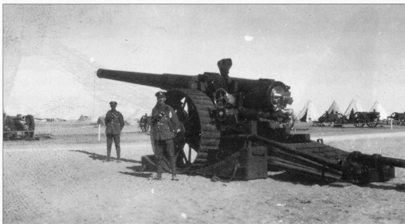
BL 6-in. gun Mk. VII – another view of Bessie , 43 Siege Battery, RGA, 1919. Note the distinctive 'flat' on top of the breech and the stepped, straight-edged profile of the barrel, which identify this as a Mk. VII. (RAHT AL317.122)
