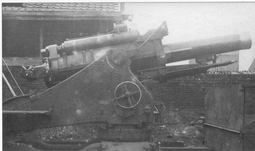
BL 9.2-in. siege howitzer Mk. II, Dora , of 154th Siege Battery, RGA, July 1917. Notable differences from the Mk. I howitzer are the profile of the barrel, the cranked bedplate girders (bottom centre) and the link bar from trunnion to buffer (top centre right). (RAHT AL1136.2)
