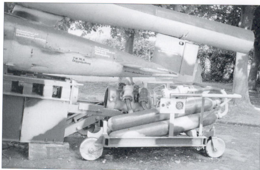
The ramp catapult was powered by a gas generator mounted on the Dampferzeuger trolley which was wheeled into place behind the ramp. These were nicknamed the Kinderwagen and were built by the Mansfeld GmbH in Leipzig beginning in September 1943. Each firing site had two of these. (T. Desautels)
