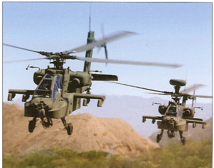
A pair of AH-64D Apaches fly at low level over the desert. The aircraft in the rear is a Longbow Apache, fitted with a mast-mounted millimetric radar system. The standard AH-64D in front has been equipped with all of the Longbow’s upgrades barring the radar system. It can be upgraded to full Longbow configuration in four hours. (Boeing)
