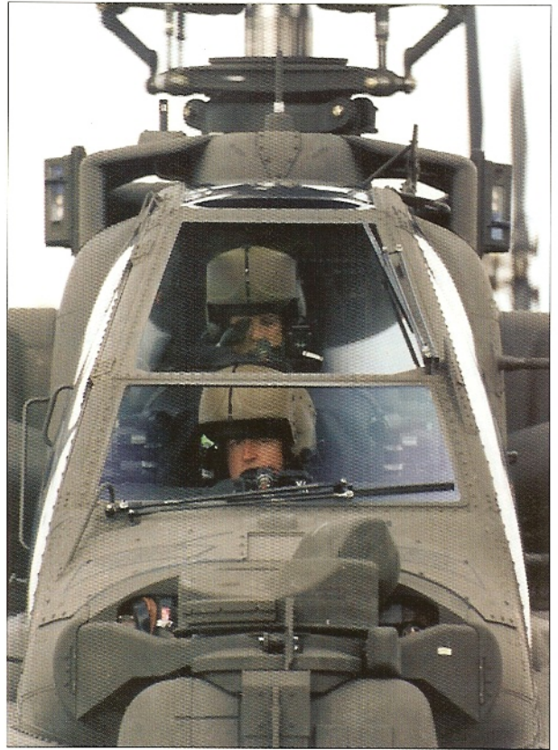
The two-man cockpit of the Apache follows the pattern established by Bell for the pioneering Model 209 Cobra, with the pilot behind and above the weapons operator. The Apache differs from its predecessor, however, in being provided with much more armor protection for its crew. (Westland)
