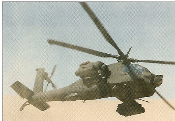
Desert flying in the Gulf brought its own unique hazards. The fine sand encountered in the region caused dangerous "brownouts:" the aircraft was enveloped by a thick cloud of rotor wash-blown sand on take off or landing. (McDonnell Douglas)
