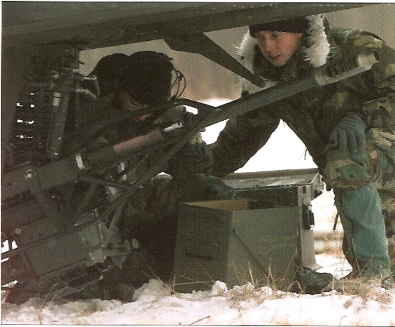
Ground crewmen load 30mm cannon rounds into an Apache's M230 30mm Chain Gun. Apaches have been and can be expected to be deployed to any climatic area from the desert to the Arctic: training in Alaska proved invaluable in dealing with the harsh conditions encountered in Balkan winters during peacekeeping operations. (DOD)
