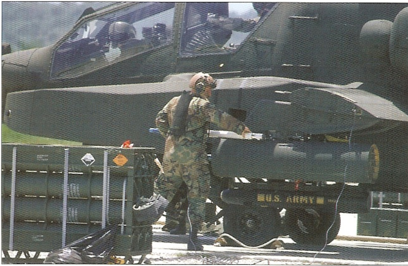
A ground crewman loads the rocket pods of an AH-64D Longbow Apache with an inert, practice air-to-air missile. Apaches have carried Sidewinder, Stinger, and Matra Mistral missiles, and are currently being tested with an air-to-air variant of the British Starstreak high-velocity man-portable SAM. (Boeing)
