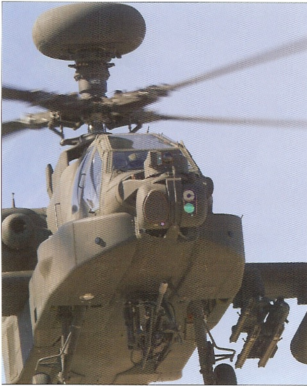
An AH-64D Apache Longbow equipped with the Modernized Target Acquisition Designation Sight/Pilot Night Vision Sensor (M-TADS/PNVS) lifts off on the first test flight of the new system. The M-TADS/PNVS provides a 150 percent improvement in performance and reliability over its predecessor. (Boeing)
