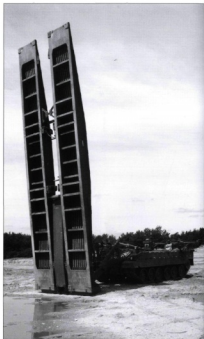
The Challenger 2 bridgelayer is named Titan. With the three-man crew completely protected under armour, Titan can carry and launch the 26m-long No 10 Tank Bridge within two minutes to span gaps up to 24.5m. It can also carry and launch the 13.5m-long No 12 Tank Bridge, as shown here, within 90 seconds. These bridges can be retrieved from either end for maximum tactical flexibility. Like Trojan, Titan can be fitted with the universal dozer kit or track-width mine plough. (Simon Dunstan)
