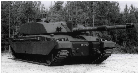
06SP93, or prototype V7, displays to good effect the main armament of Challenger 2 – the 55-calibre long L30A1 120mm rifled gun. Above the barrel is the barbette housing of the Thermal Imaging System (TIS) that is an improved version of the one fitted to Challenger. This device provides outstanding night vision to both the commander and gunner, as well as in bad weather or through battlefield smoke. (VDS)
