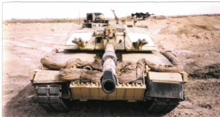
A worn and battered Challenger 2 of 12th Troop, Egypt Squadron, 2 RTR, illustrates the configuration of the explosive reactive armour (ERA) array on the toe plate and the appliqué armour on the glacis plate, masked here by an Israeli camouflage net. Note the prominent CIPs on the front turret faces. These were mutual recognition devices for the Coalition forces and relied on the principle of varying thermal characteristics of different materials. (RTR)
