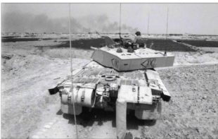
Zero Charlie, the Challenger 2 of the second-in-command (2i/c) of Cyclops Squadron, 2 RTR, takes up position among the tomato fields on the outskirts of Az Zubayr. Of particular note is the position of the GPS antenna, just visible behind the loader's hatch, and the white box of the Blue Force Tracker on the turret roof. As its name implies, this device assisted in identifying the positions of friendly forces and was commonly fitted to the tank of the 2i/c in each armoured squadron. (RTR)
