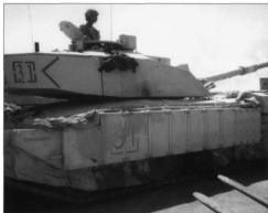
'Crusader', the Challenger 2 of the troop sergeant, Sergeant Andy Topping, of 7th Troop, Cyclops Squadron, 2 RTR, halts at the replenishment point after the decisive action at Az Zubayr on 26 March 2003 when the tanks of 7th Troop were hit repeatedly by RPG rockets without any significant damage. Note the impact point of an RPG-7 on the turret side of callsign Three One. (Andy Topping)
