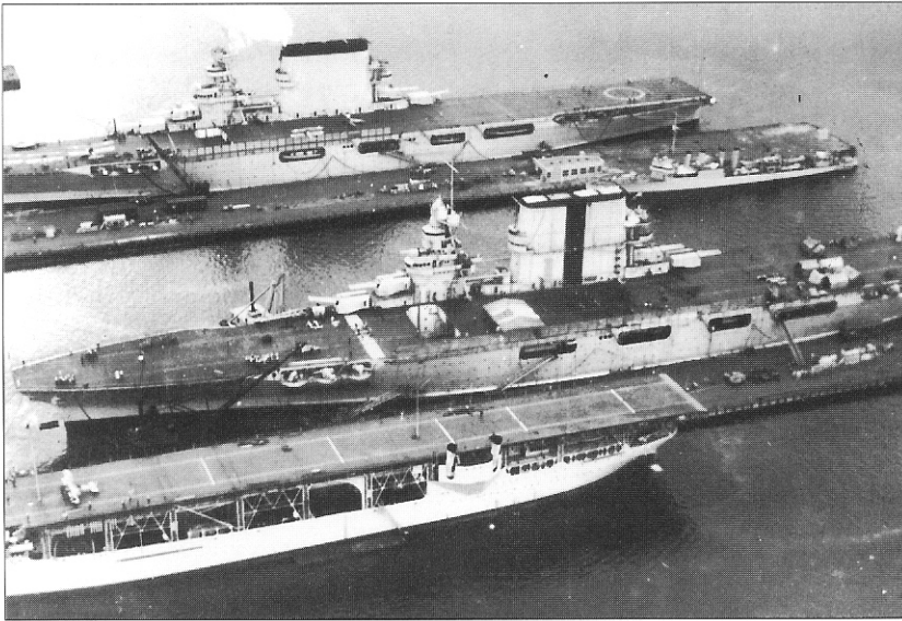
The US Navy's first three carriers shown c.1930 in Bremerton, Washington. The immense size of the converted battle cruisers Lexington and Saratoga compared to the experimental Langley is striking.
