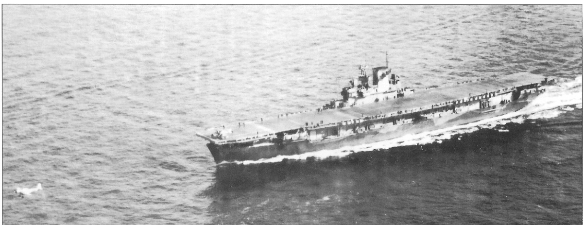
Wasp shown in March 1942 in her Measure 12 (modified) scheme; she would retain this camouflage until her loss. The aircraft spotted forward is a Grumman J2F utility aircraft.
