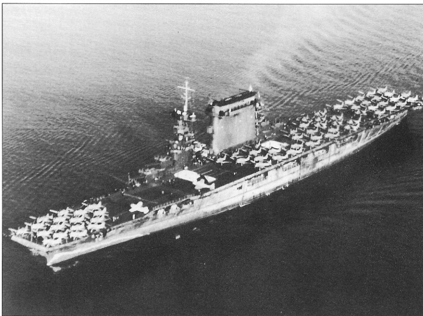
Lexington on October 14, 1941 with her air group. She is carrying F2A Buffalo fighters forward, SBD Dauntlesses amidships, and TBD-1 Devastators aft. The ship is wearing a Measure 1 camouflage scheme with a Measure 5 false bow wave.
