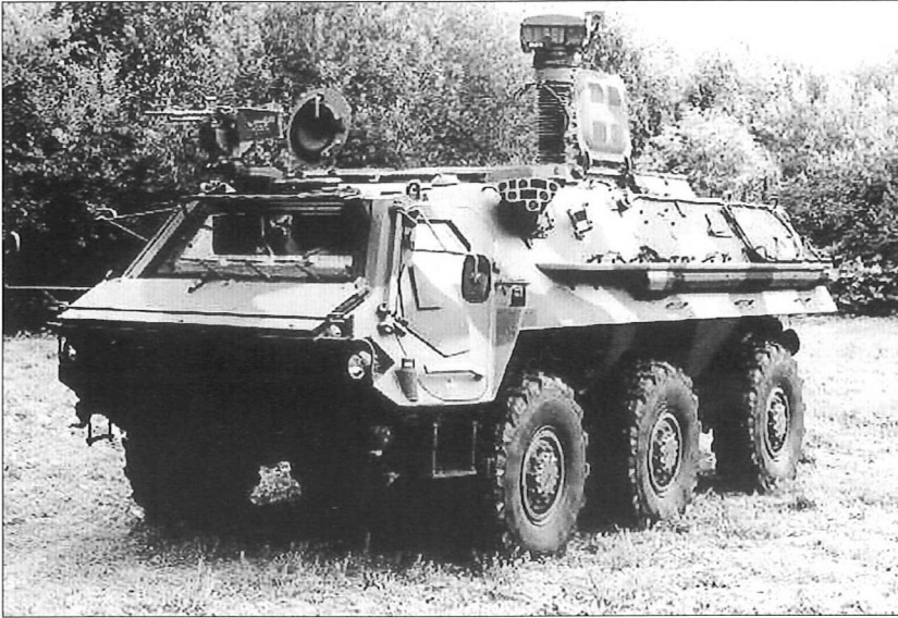
The German-built 6x6 M93A1 Fox NBC reconnaissance system is presently used in lieu of the M1135 NBCRV, which will be fielded later. The 17-ton Fox is amphibious and crewed by three personnel. This one is painted in the NATO three-color European camouflage scheme. (US Army)
