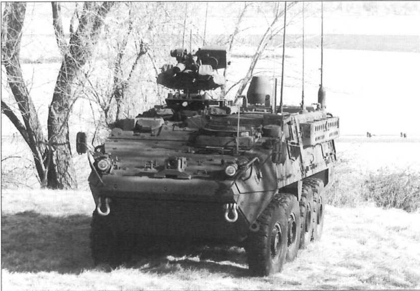
An M1130 Command Vehicle (CV) carries commanders at battalion and higher echelons. It mounts numerous radios and command-and-control systems. This CV has a 40mm automatic grenade launcher on its RWS, but it is usually fitted with a .50cal. machine gun. (GDLS)
