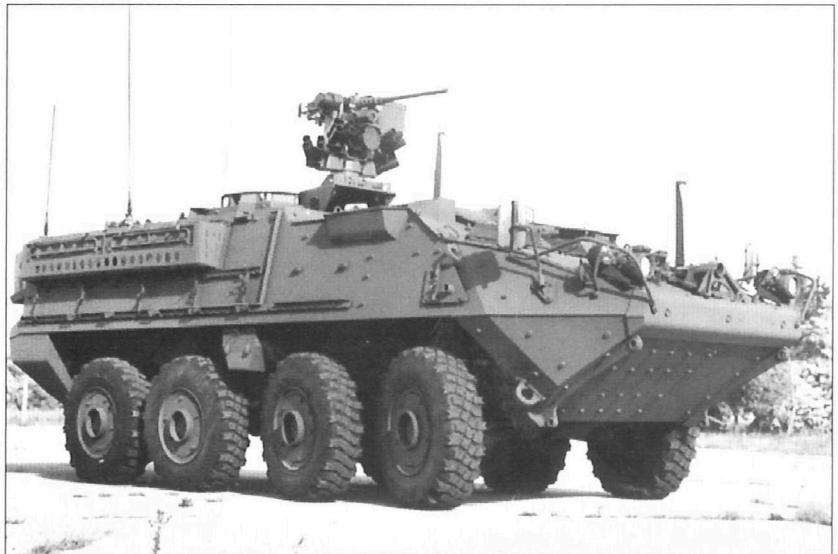
A right front view of the Stryker M1126 Infantry Carrier Vehicle (ICV). Because of limited interior space, exterior equipment racks were fitted to the sides. The vertical wire-cutter bars can be seen on the front bow and forward of the weapons station. (GDLS)
