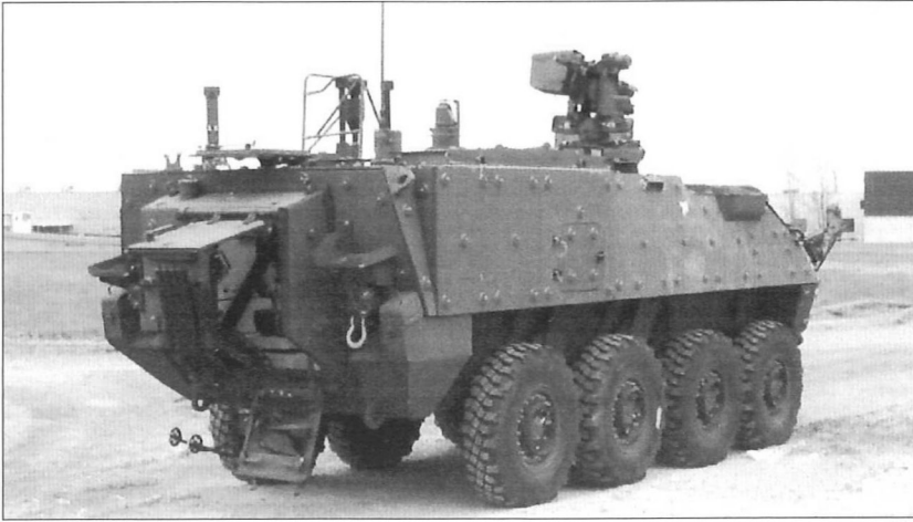
The rear housing hatch, similar to that found on the Fox NBC reconnaissance vehicle, is open on this M113 NBC Reconnaissance Vehicle (NBCRV). This housing contains ground sample collection systems and marker dispersers. Note the NBC airborne sample collection masts atop the vehicle. This NBCRV has experimental appliqué armor. (US Army)
