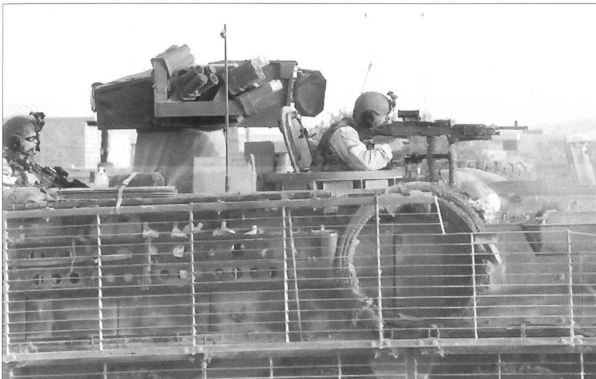
An ATGM vehicle commander scans for targets with a 7.62mm M240B machine gun. Another crewman searches for targets from a rear "air-guard" hatch. The four M6 smoke grenade launchers are evident. (US Army)
