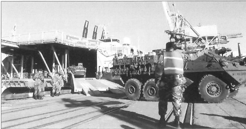
Sealift is another deployment option for Stryker Brigade Combat Teams (SBCTs). Here an ICV is backed on to a roll-on/roll-off (RO/RO) cargo ship. (US Army)
