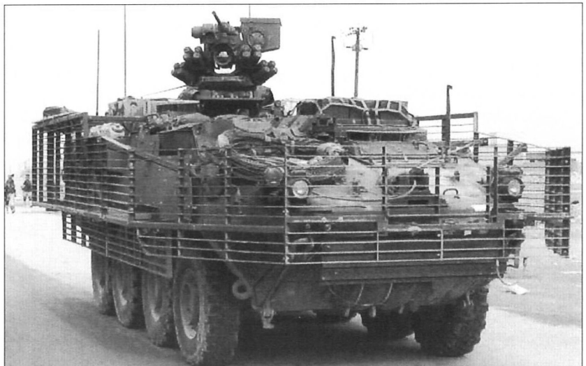
Here shown in Iraq, this ICV is fitted with the controversial slat armor. While the armor adds a great deal of weight, adversely affecting its off-road capability and making it top heavy with increased roll-over hazard, it has proved to be effective against RPG fire. (US Army)
