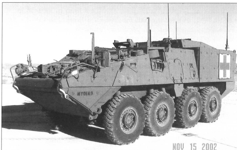
The M1133 Medical Evacuation Vehicle (MEV) is unarmed. The heightened and widened casualty compartment is evident. It is the only Stryker with a heightened rear compartment, although the MC-B and NBCRV have similar widened structures. (US Army)
