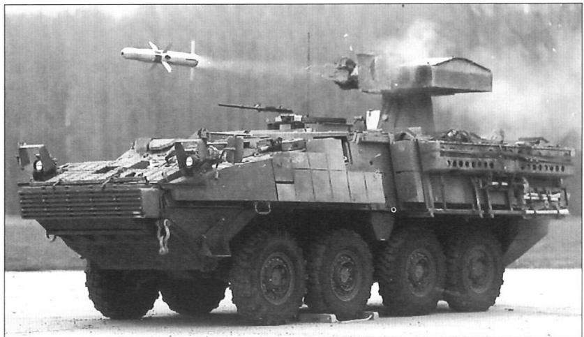
A TOW 2 missile is launched from this M1134 Antitank Guided Missile Vehicle (ATGM). The launcher pod is elevated 20in for firing. This ATGM is fitted with MEXAS 2 ceramic appliqué armor tiles. Note the gap in the appliqué tiles for the engine air intake and side hatch. (GDLS)
