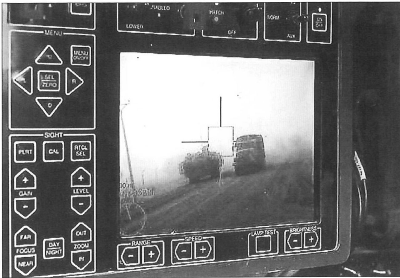
The RWS Video Display Terminal (VDT) at the vehicle commander's station. This monitor displays the view seen by the RWS' video thermal imager camera. (US Army)
