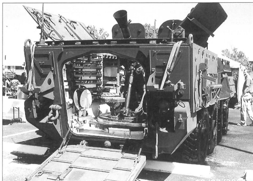
An M1129B Mortar Carrier (MC-B) showing the 120mm M121 mortar on its 360-degree turntable. The muzzle attenuator device reduces muzzle blast. The mortar can be fired with the rear ramp closed, but it is better opened to reduce blast overpressure and to allow ammunition to be passed from the 1 1/2-ton trailer to conserve ready ammunition in the internal side racks. The MC-A was essentially a modified ICV carrying a 120mm M120 mortar that could only be fired dismounted. (US Army)
