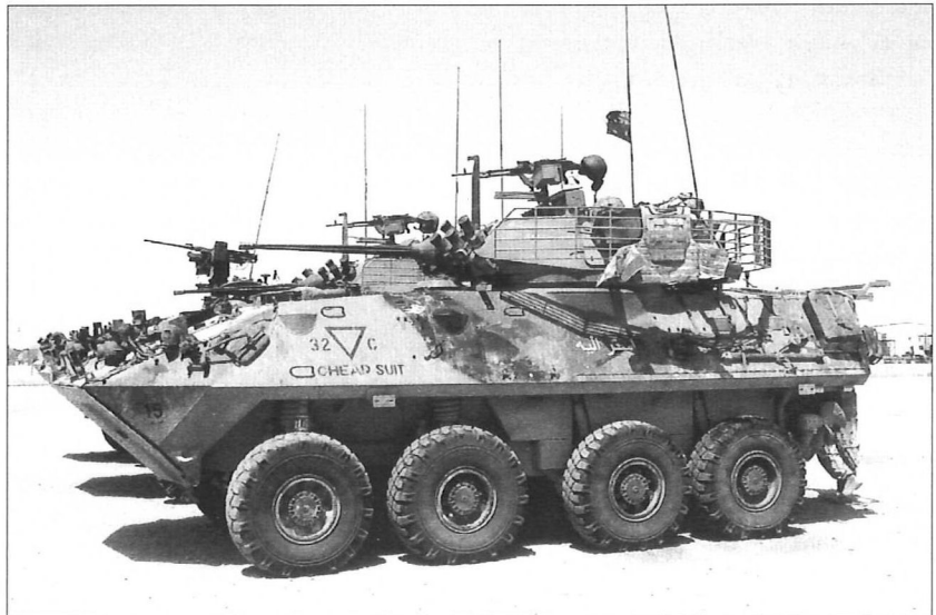
The Stryker was derived from the 8x8 Piranha III, variants of which are used by a couple of dozen countries. Here are Australian ASLAV-25s deployed to southern Iraq and in use since 1996. (Ken Caputo)
