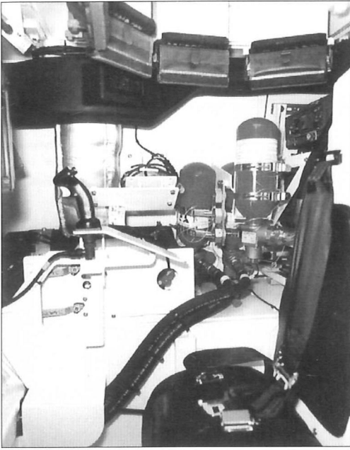
The vehicle commander's station with its seat, RWS control joystick, and automatic fire extinguishers. Stryker interiors are painted acrylic glossy white. (GDLS)
