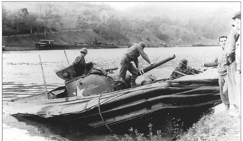
An American Sherman DD in trouble during training for the Rhine crossing. Owing to shortages both American battalions involved in this operation were brought up to strength with British-built M4A2 and M4A4 types; however this would appear to be a regular American M4A1 type.
