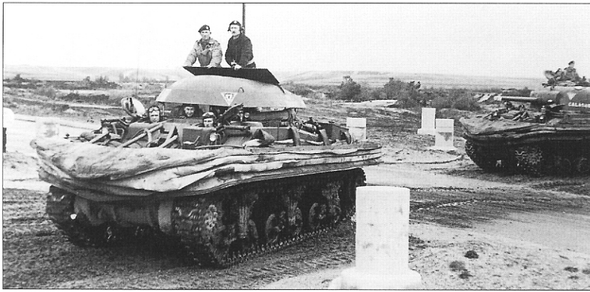
The unique Sherman Kangaroo DD, here in the M4A4 form, showing the protective cover over the turret ring from which infantry peer out. A regular DD gun tank named Galashiels follows the Kangaroo.
