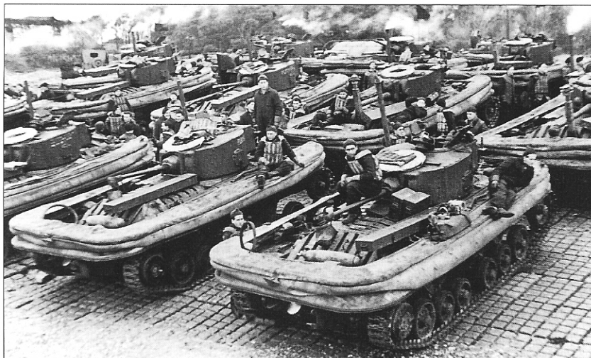
Stokes Bay, on the mainland side of the Solent, was the principal centre for training DD crews to work in conjunction with the Royal Navy. Here Mark V (foreground) and Mark XI Valentines DD wait, with turrets traversed, to back onto landing craft. Crews wear conventional life preservers while the tank carries one lifebelt. Note the air cylinders on the engine decks of the nearest tanks.
