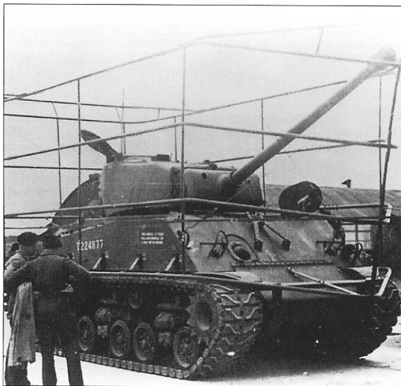
In the United States production of 76mm gun DD Shermans was undertaken to fulfil British requirements. Meanwhile in Britain a similar tank is fitted out with a replica of the tubular framework to show how it will accommodate the longer gun.
