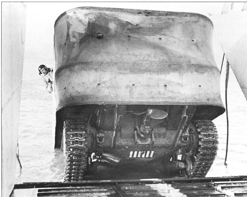
Viewed from aboard an LCT, a Valentine DD enters the water. The propeller is visible, ready to engage, but the commander is more interested in the safety of his screen. The stripes painted beneath the propeller at the back are a night driving aid.
