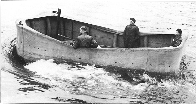
An early Valentine DD afloat. These first examples have a characteristic dip in the middle of the screen, and on this one the driver appears to have an extended periscope to view over the screen. The studied nonchalance of the rest of the crew suggests very calm water.
