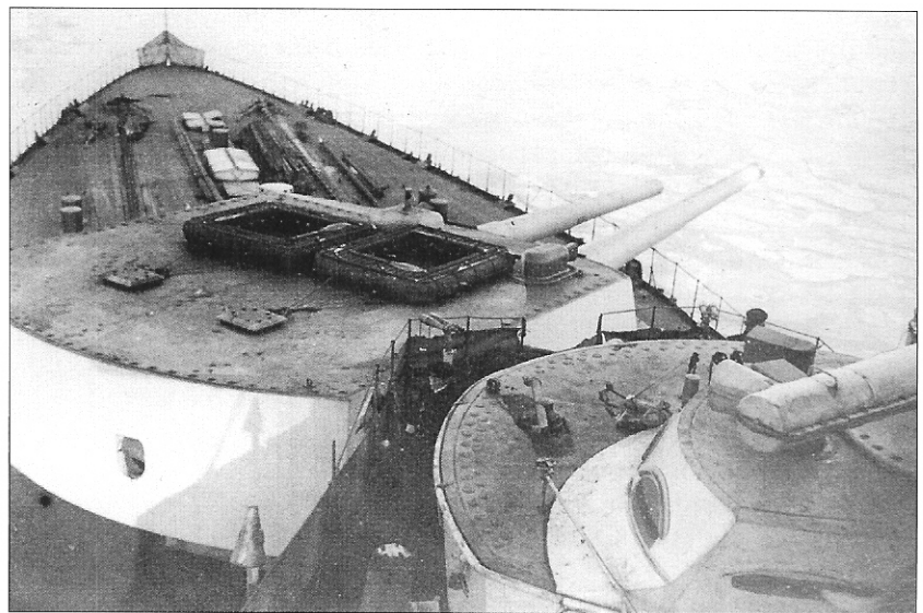
RIGHT A view of Seydlitz ' conning tower and A turret. This picture offers a good view of the various periscopes on the tower and the rangefinder fitted to the Artillery Direction Position, the raised part of the heavily armoured conning tower. On top of A turret are vents for expelling gases, and at the rear the hatches for installing sub calibre guns. Each turret also has a rangefinder fitted at the front, in this case just behind the life rafts. (Courtesy of Stuart Haller)
