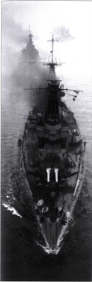
Aerial view of HMAS Australia showing foremast, rangefinder and training scale on A turret. (IWM)
