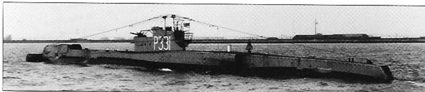
HMS Trenchant showing its aft-facing external tubes amidships and on the stern. This submarine claimed the cruiser Ashigara in 1945.
