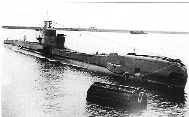
The successful HMS Torbay in Barry in 1945. Note the upward-folded forward hydroplanes and the absence of forward external torpedo doors.
