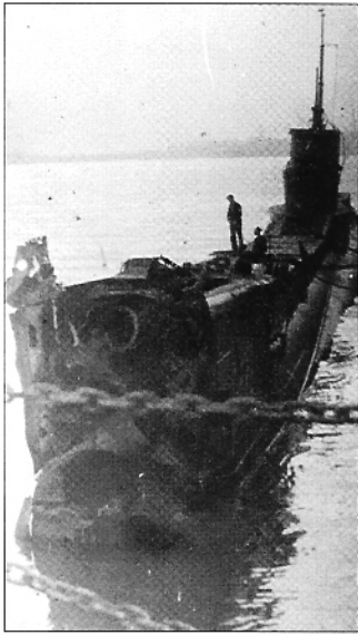
An early T-Class, HMS Triumph , luckily escaped destruction after being mined in the North Sea in December 1939. It is thought to have been lost to a mine in the Mediterranean two years later.
