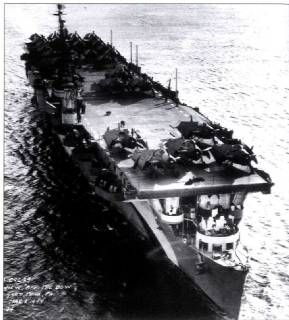
Bataan off the Philadelphia Navy Yard in early March 1944 before departing for the Pacific. The 40mm quadruple mount fitted on the bow is clearly shown, as are several 20mm single mounts. Two dual 40mm mounts are shown on the starboard side forward of the island. The size of the larger quadruple mounts meant that they could only be fitted on the bow and stern of the light carriers.
