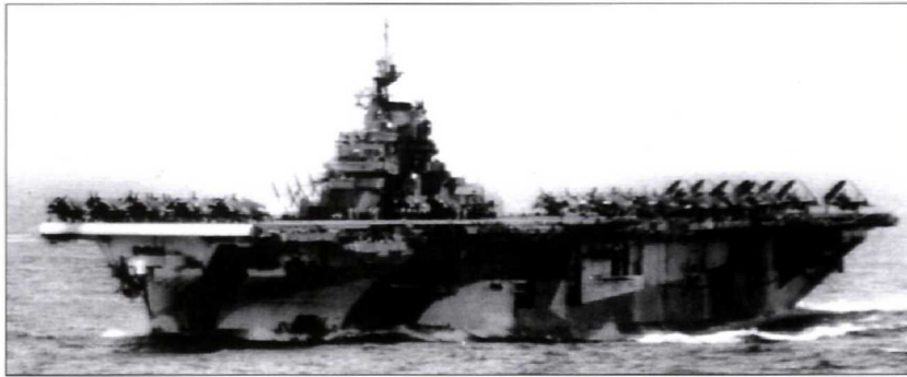
Hornet on March 27, 1945, operating off Okinawa. The ship is in a Measure 33/3a scheme. The large deck park is typical of American fleet carriers. The many aircraft still spotted forward suggest that she has just recovered aircraft and is in the process of re-spotting the flight deck for future operations.
