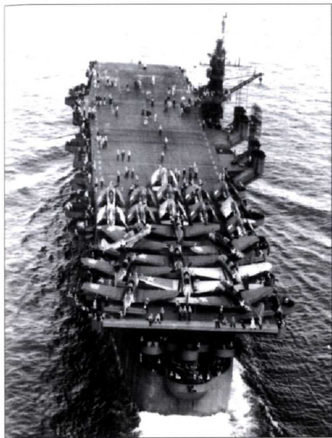
Princeton during her shakedown cruise in May 1943. On deck are nine SBD Dauntless dive bombers and 12 F6F Hellcat fighters. The Dauntless dive bombers did not possess folding wings and proved difficult to operate on the limited flight deck of the light carriers.
