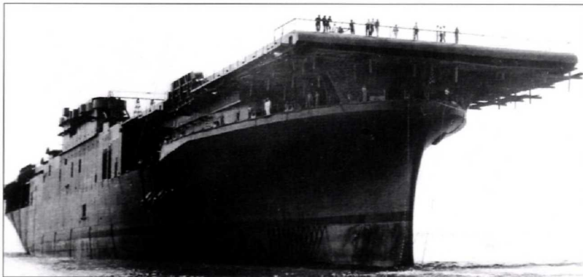
Essex was launched on July 31, 1942, many months ahead of schedule. At 27,500 tons (33,003 tonnes) design standard displacement, she was the largest American carrier built to date, with the exception of the two Lexington class carriers that were converted from battlecruisers.
