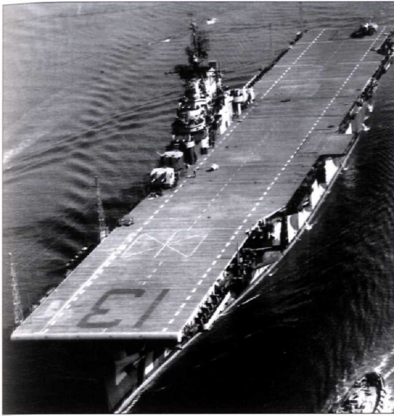
A fine study of Franklin as she was commissioned in February 1944. The radio masts were brought into an upright position when flight operations were not underway. Many of the galleries for 20mm guns alongside the flight deck are visible. The outrigger for the hangar catapult is also visible in its upright position just aft of the port side 5in guns.
