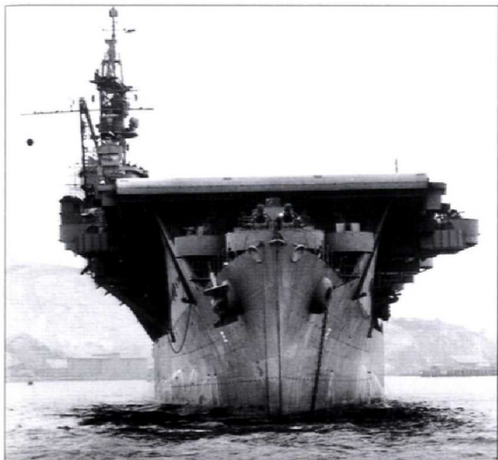
Independence viewed from the bow in July 1943. The bow 5in gun has been removed and has been replaced with a quadruple 40mm mount. Two additional bow-mounted 20mm single mounts were also fitted.
