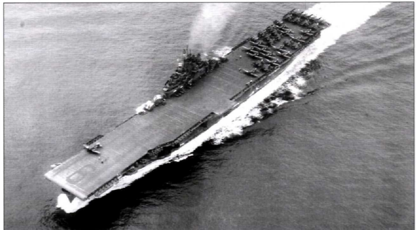
Essex during the Okinawa campaign in May 1945 with her late war air group. Between F6F Hellcats and F4U Corsairs (both visible on deck), over 70 percent of the air group was made up of fighters. Note the modified bridge.
