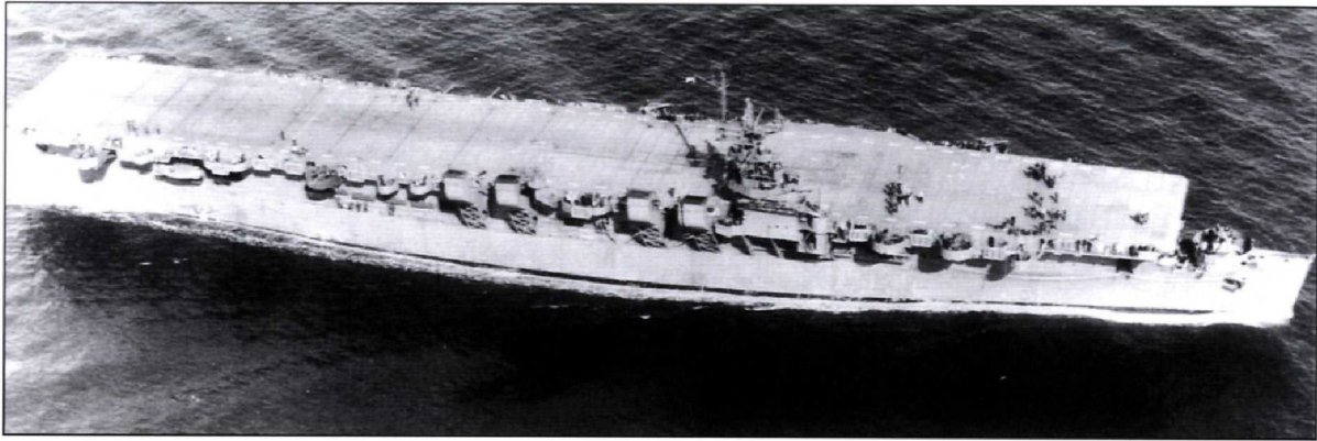
Independence in her original configuration with a bow-mounted single 5in/38 gun. Not visible is the second 5in gun fitted on the stern. Both were removed within weeks of commissioning. The ship is in a Measure 14 scheme.
