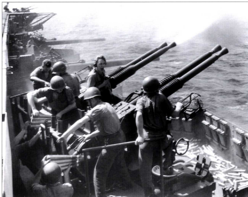
Shown here is a 40mm quadruple mount on Hornet in February 1945, during the raids on Tokyo. This is the gun mount on the port side of the flight deck, just forward of the aft pair of 5in/38 single guns. Note the expended shells to the right of the photo and the ready rounds lining the gun tub. The 40mm gun was probably the most successful medium-range antiaircraft gun of the war.
