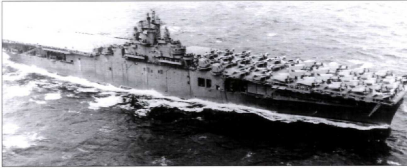
Lexington in November 1943 after having recovered from an air strike. The ship appears in her early configuration with five radio masts (lowered for flight operations), an unmodified bridge, and no outboard starboard side sponsons. The two 40mm quadruple mounts located on the aft starboard portion of the hangar deck were later moved into sponsons to increase their fields of fire.
