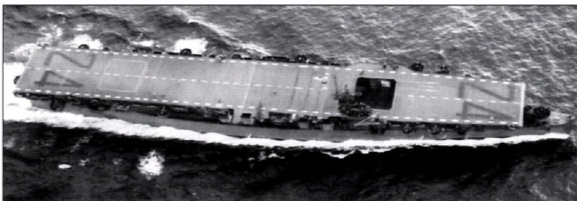
The deck markings of an Independence class carrier are clearly shown in this December 1943 view of Belleau Wood . The deck is in a dark blue stain with large numbers in black fore and aft. The flight deck stripes are in what appears to be white with yellow elevator edge markings.
