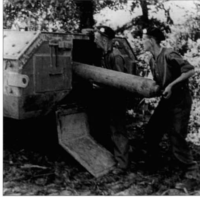
Two troopers, with their cap badges conveniently blotted out by the censor (but probably 141st RAC), demonstrate that fitting pressure cylinders, all five of them, into a Crocodile trailer is no easy task.
