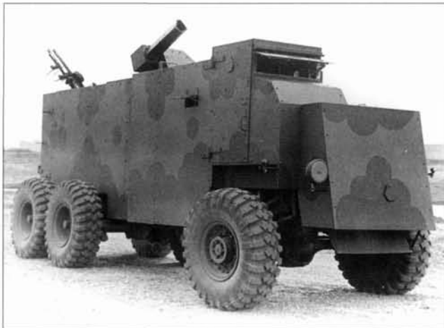
This is the Mark IA Heavy Cockatrice, an odd, asymmetrical vehicle that used the same AEC 6x6 chassis as the Heavy Pump Unit. The flame-projector turret is behind the cab and the two machine guns are worked from an open section at the back.
