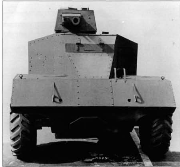
Rackham's Basilisk armoured car on the AEC Matador chassis. The flame-projector is in the turret and it may be that the third crew member, designated as observer, would be located alongside where a periscope head may be seen. If so, his view would be very limited.
