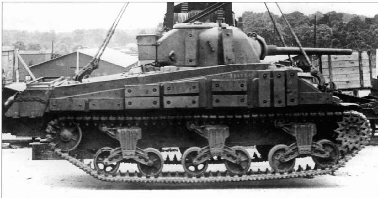
A Sherman V (M4A4) Adder with ballast weights to represent stowage is hoisted clear of the ground by a crane, probably to establish the centre of gravity. For details of the additions refer to the colour plates. Surviving publications also refer to an M4A2 (Sherman III) version of Adder.
