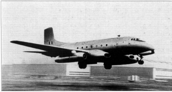
Test Pilot, Wg. Cdr. Waite Gibbs. Photographed on 2 February 1955, the machine carries two reheated Bristol Siddeley Olympus outboard of the Nenes. (Bristol Siddeley)
