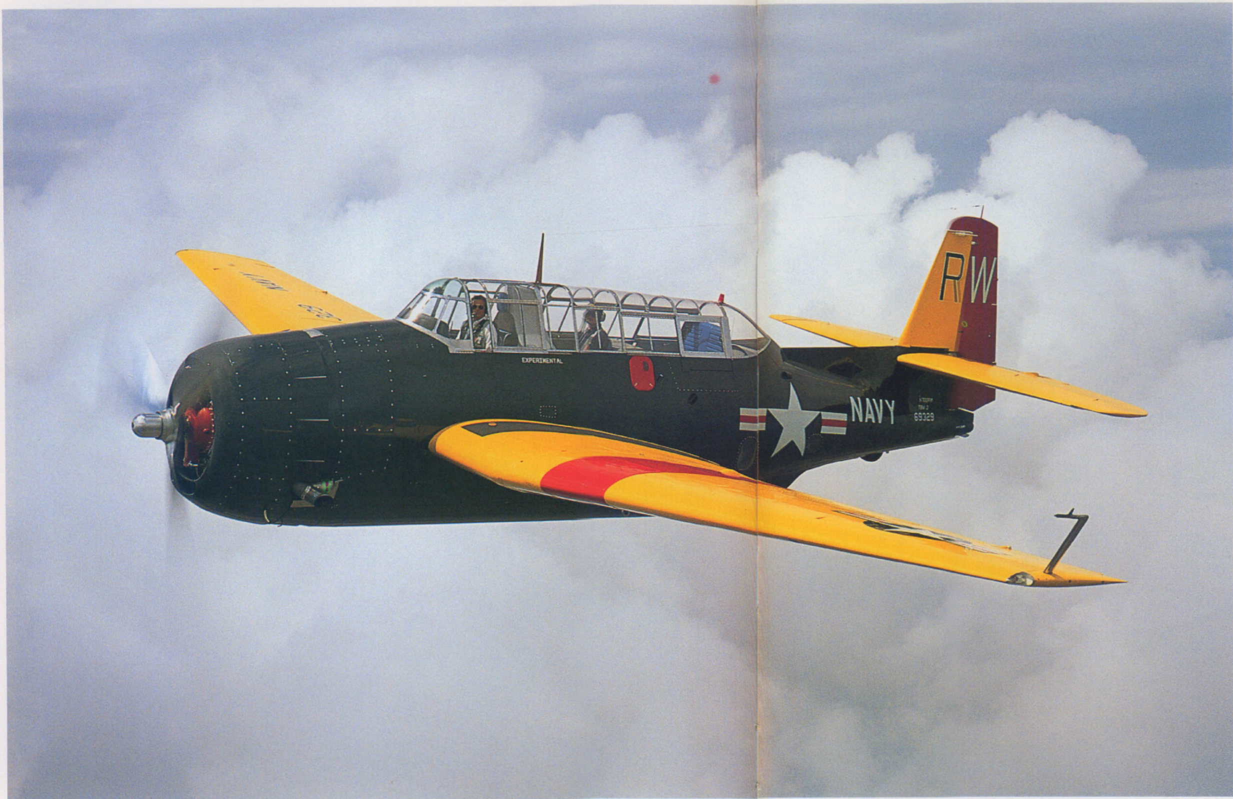
After the war, Avengers soldiered on in a variety of second-line duties, operating until 1954 with the Fleet and longer with the Reserves. TBM-3E (BuNo 69329) N700RW (ex-N73642) is finished in colourful post-war utility squadron markings and the modified canopy was fitted to some Avengers that were utilized for COD (carrier onboard delivery) missions, and designated TBM-3Rs or 3Us. This aircraft flew as tanker 23 with Reeder Flying Service at Twin Falls, Idaho, during the 1960s and then lapsed into dereliction before being rescued for restoration. N700RW is owned and operated by the Lone Star Flight Museum, Galveston, Texas. Approximately 35 Avengers remain airworthy today, while around a dozen are under restoration and another 20 are on display in museums
