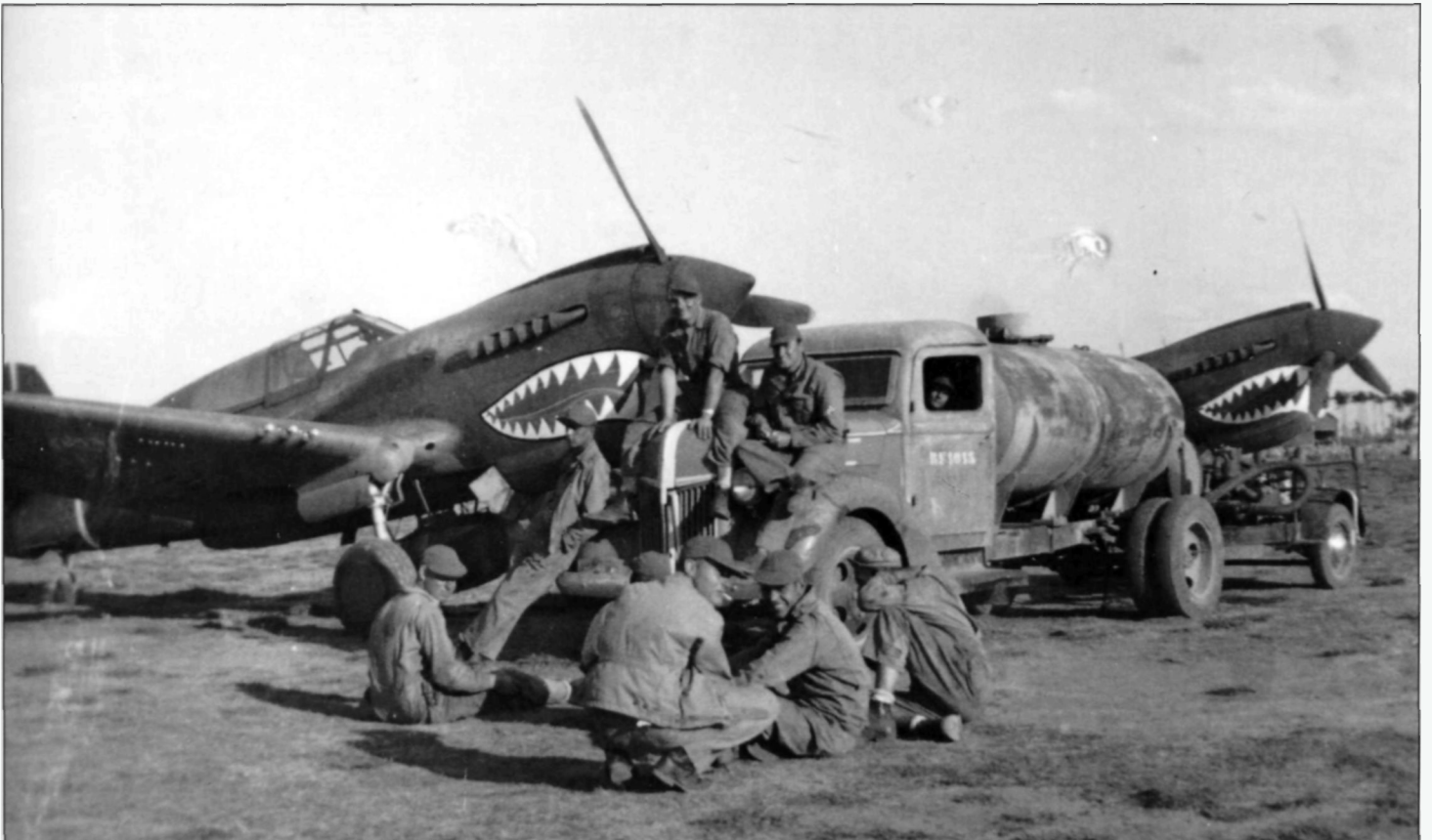
Groundcrewmembers from the 75th FS take a break from refuelling aircraft on the flightline at Hengyang. The P40K at left is fitted with mounting brackets for small bombs beneath its wing. Note also that the outline for the shark's tongue has been chalked on, although it has not yet been painted, and that neither P-40K has a shark's eye on its nose (via Carl Molesworth)
