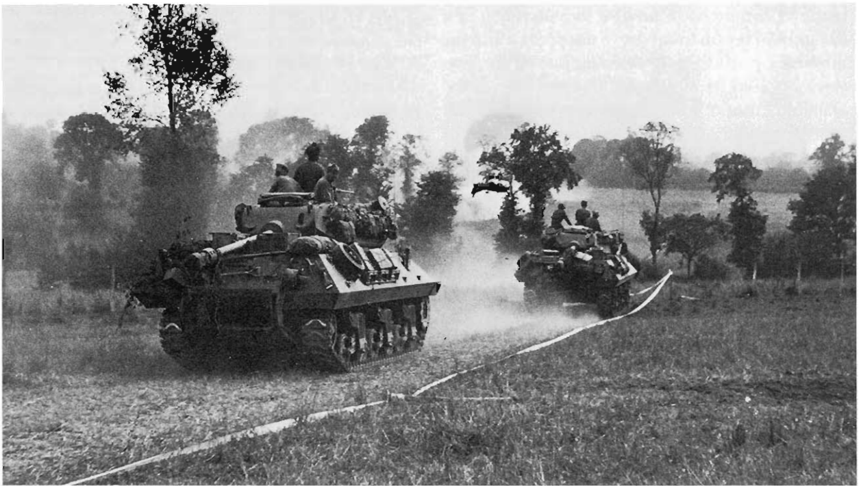
24 Achilles M10 self-propelled 17pdr anti-tank guns follow a taped 'safe' lane in the bocage of Normandy. At least one battery of the divisional A/T regiment in NW Europe was self-propelled to work with the armoured brigade; the remainder supported the infantry with towed 17pdrs. (Imperial War Museum)
