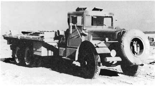
8 White-Ruxton 6x4 tank transporter—one of the early models used by the division in 1941. The following year they were largely replaced in recovery units by Scammell semi-trailers. The vehicle shown appears to have been sprayed with a dark coloured camouflage over the basic stone shade; the soft edges are untypical, as most Middle East theatre camouflage directives stressed the need for sharp-edged patterns. (Coniford)
