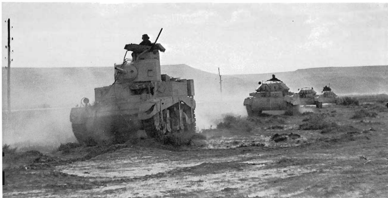
4 Stuart "Honey" followed by Crusader Mk Is, late 1941, in typical desert scrub country with escarpment in background. All appear to be finished plain stone without added camouflage or markings. (Imperial War Museum)
