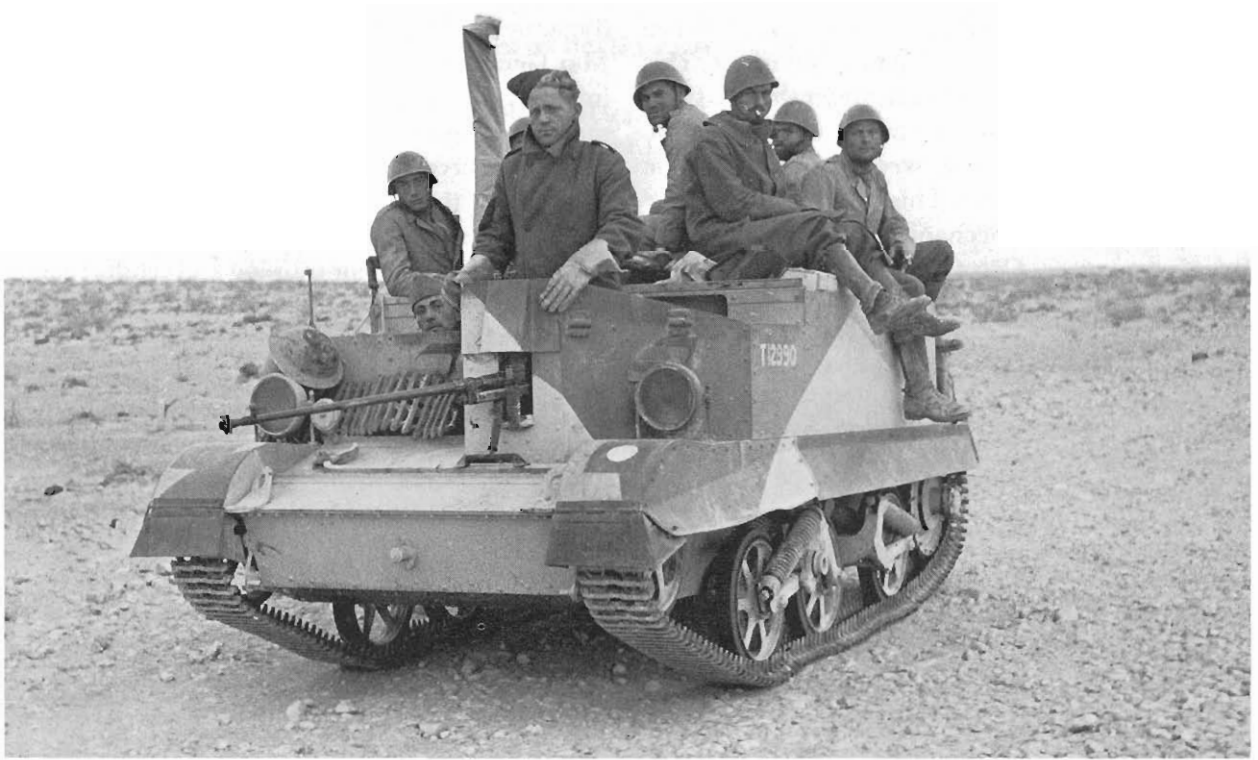
1 Universal carrier of a motor battalion with Italian prisoners, late 1940; typical armament of Boys anti-tank rifle in front sponson and (covered) Bren gun on A/A mounting. These vehicles were subsequently used by carrier platoons in lorried infantry battalions, and as artillery OP vehicles, ambulances, mortar and machine-gun carriers in NW Europe. (Imperial War Museum)
