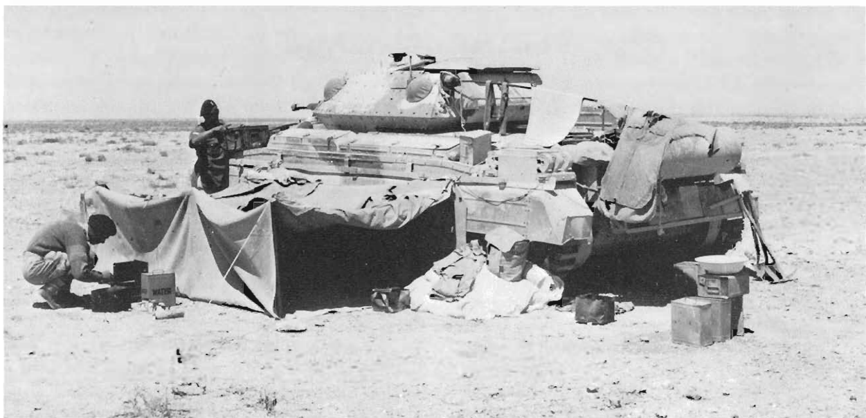
3 Crusader Mk II of 3rd County of London Yeomanry, photographed at a moment of domestic tranquillity! The markings of 'A' Sqn, 4 Troop are just visible on the rear of the turret bin, beyond the lowered No. 9 set aerial which is here being used as a washing-line. A name ('AILSA II?') is dimly visible on the turret side, but there are no divisional or unit tactical signs. The rack of 2gal water tins, and the use of cut-down 4gal 'flimsies' as stoves, are typical, as is the tarpaulin bivouac slung from a side rail originally fitted to mount a hessian 'lorry' camouflage rig. (Sharpshooters)
