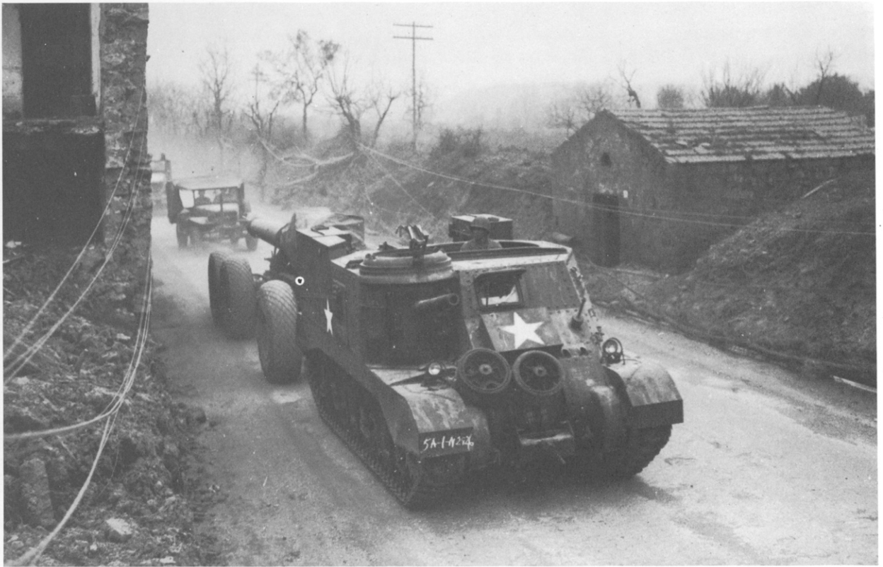
A 240mm howitzer towed by the turretless converted chassis of a Lee tank on an Italian road— this was the largest mobile gun employed on this front. Note chalked 5th Army tactical signs on trackguard. (US Signal Corps)
