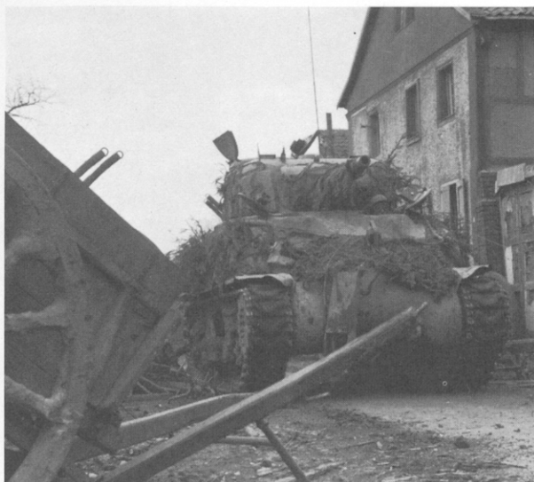
A Sherman tank of one of the division's armoured battalions—converted into a 'tank retriever', according to the original caption—crashes a road-block of wagons in Kelz, Germany, early in March 1945. On the original print heavy applique turret armour can be seen beneath the scrim and foliage camouflage. (US Army)
