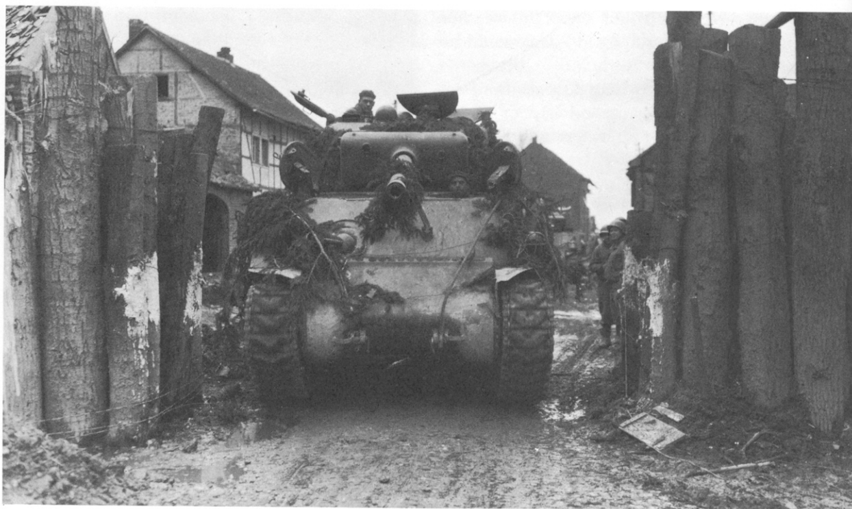
1 March 1945, Gladbach, Germany: a Sherman tank of the 745th Tank Bn. attached to 'Big Red One'. This appears to be a late-model M4A2 with 76mm gun mounted in the T23 turret. (US Army)
