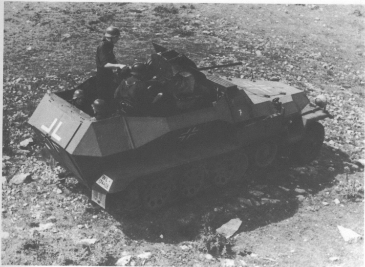
The SdKfz 251/17 half-track, with its specially widened body to allow traverse space for the 20mm anti-aircraft cannon. The red-on-white unit insignia identifies these vehicles as belonging to 10th Light Battery, 2nd Battalion, Flak Regiment 'HG'. (Bundesarchiv 639/4276/34 & 4288/11)
