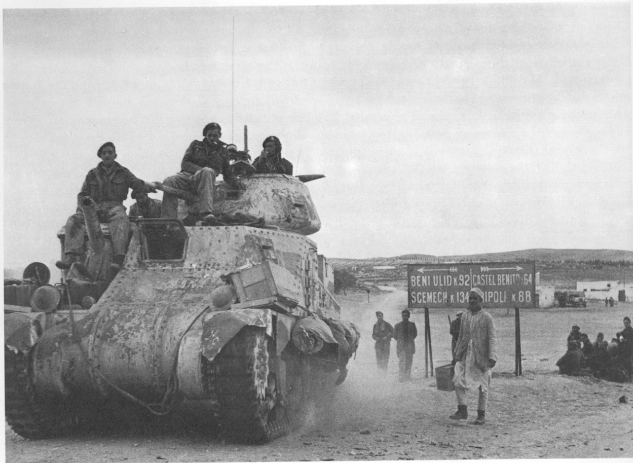
This Grant shows signs of wear after its long advance; the torn sandguards and sand-blasted paintwork are typical.
