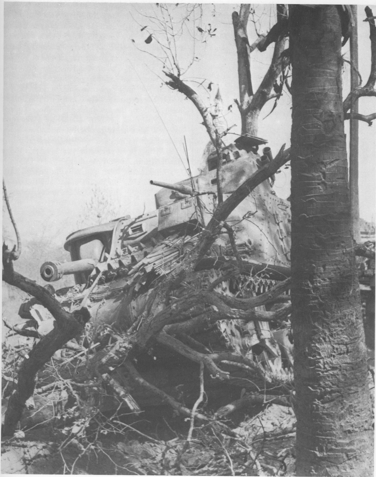
The last earthly sight of many a Japanese soldier. The counterweight fitted to the M2 gun provided a better working balance for the stabilizer, which worked in elevation only.
