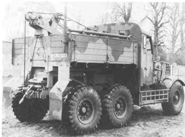
Scammell SV/2S heavy recovery tractor showing the extending jib and winch gear that enabled it to recover vehicles that could not be handled by the ARVs. Each armoured battalion's REME LAD had two Scammells, and the infantry brigade workshop had another four; the armoured brigade workshop had six transporters for recovery purposes. (Conniford)
