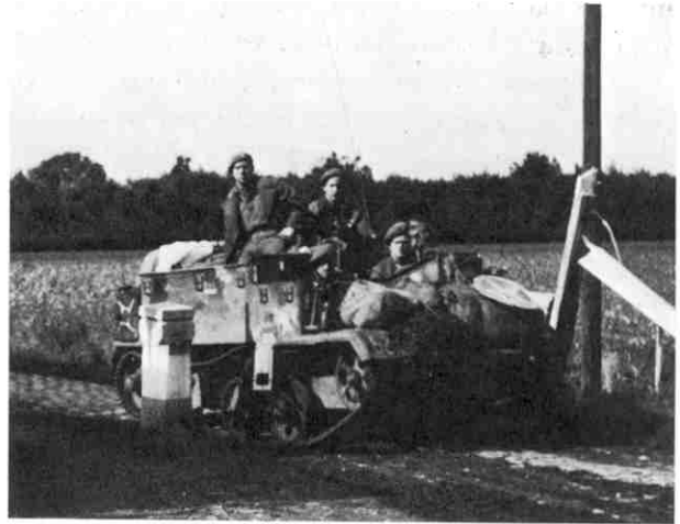
Universal Carrier MkII of 3rd Bn. (Infantry) Irish Guards, armed with a pivot-mounted .30 cal. Browning machine gun and fitted with wireless, probably an '18' or '38' set. As the upper surfaces of carriers were small and tended to get covered with loose gear, the air recognition sign—a white star in a circle—was sometimes painted on a plate, as here, that could be put on top of the pile. The unit tacsign—'62' on green—can be seen in front of the driver, and there is a water jerrycan, with the indentations filled in white, on the back.
