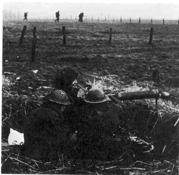
Vickers .303 MMG in action. These guns were used both by the Northumberland Fusiliers and the support company of the 1st Motor Bn., Grenadiers. The condenser tin for the cooling water jacket and an ammunition box can be seen under the front of the gun, and the dial sight for indirect fire is just visible above the loading number's helmet.
