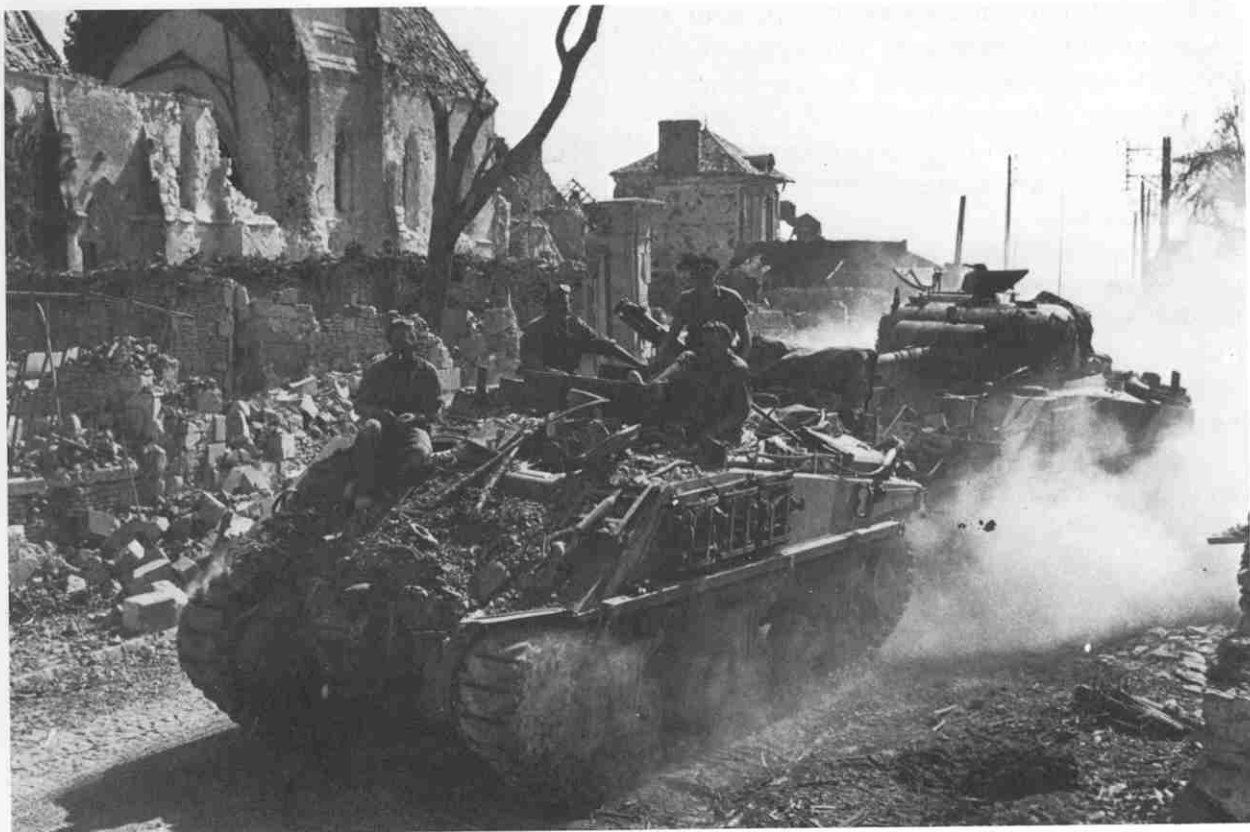
Sherman ARV recovering a Sherman gun tank. Each squadron had one ARV, virtually a turretless gun tank with a .50 cal. Browning. Although good for towing, they could not recover vehicles with damaged running gear which were unable to 'roll'.
