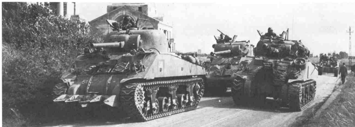
Tanks of the 2nd Grenadiers in France. The nearest is a Sherman V 'Rhino' fitted with the American-designed Culin cutter for breaking through hedgerows; a Sherman Ic Firefly is in the centre, and a Vc Firefly on the right, both with 17pdr. guns. The unit tassign—'51' on red—the divisional sign, and 'B' Squadron sign enclosing tanks' individual numbers within the battalion can be seen on the 'Rhino', while the Ic Firefly appears to have a name painted on the plate in front of the driver's hatch. (This, and all other photographs not specifically credited otherwise, are from the Imperial War Museum collections.)
