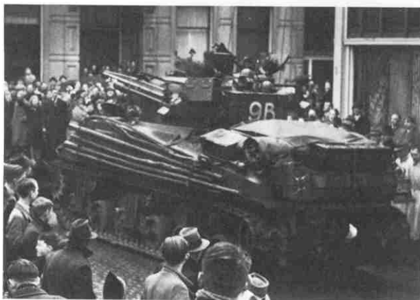
A Sherman V of 1st Coldstream fitted with Typhoon rocket launching rails. These were a local modification unique to the Coldstream; they were aimed using the blade vane on the turret top, one being aligned for a range of 400 yards and the other for 800. They proved good for clearing roadblocks but no opportunity occurred to evaluate them against armour. The tank has its troop number and individual letter—a different system from the straight-through numbering used by the Grenadiers—on the turret box, and the 'B' Squadron square on the rear hull plate. The tacsign—'52' on red—can just be seen on the right trackguard.
