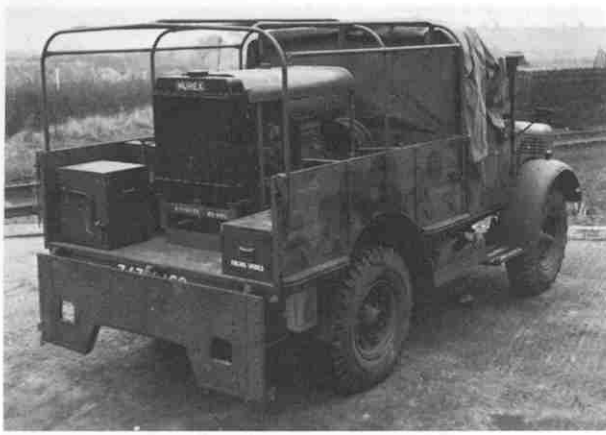
Bedford MWD 15cwt truck. This vehicle provided the bulk of the Division's light transport in all units. The example above is fitted with a welding generator, but office, compressor, W/T, water truck and various other versions were used as well as the simple general service open-bodied type. (Conniford)
