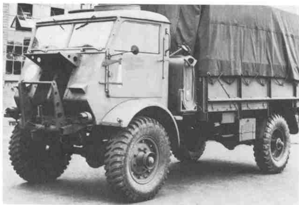
Fordson 3-ton 4x4 GS WOT6 lorry. This vehicle provided much of the Division's softskinned transport, equipping 310 Coy. RASC and unit echelons. The official camouflage scheme for softskins consisted of globular black patches on khaki, but many Guards vehicles appear to have been left plain khaki. (Conniford)
