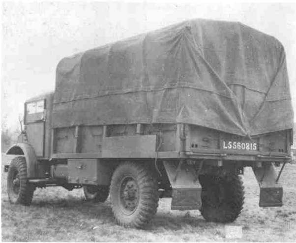
Canadian Ford CMP 4 × 4 3-tonner with metal panel GS body. The third main load carrier within the Division, although less numerous than the Fordsons and Bedfords; some were used by 224 Coy. RASC. (Conniford)
