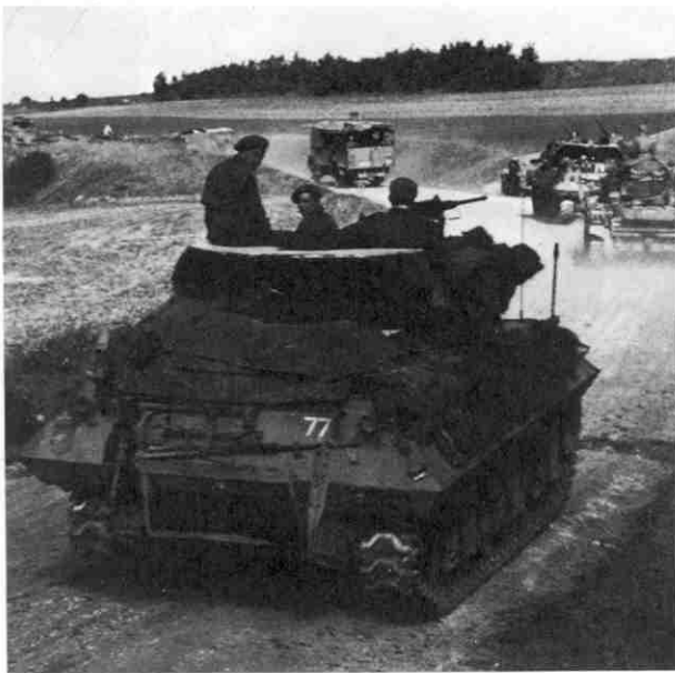
M10 self-propelled anti-tank gun following a Crusader OP tank, both of 21st Anti-Tank Regiment, RA. Both 3in and 17pdr. M10s were used in the Division; this one has its .50 cal. Browning machine gun mounted on the turret top and has the divisional sign on the left and the unit tacsign on the right of the rear plate. There is a troop sign above the tacsign but this is obscured by the tarpaulin. The Crusader could be a redundant AA tank.
