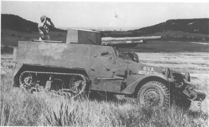
75mm Gun Motor Carriage M3, with front and side-door screens raised. (RAC Tank Museum)
