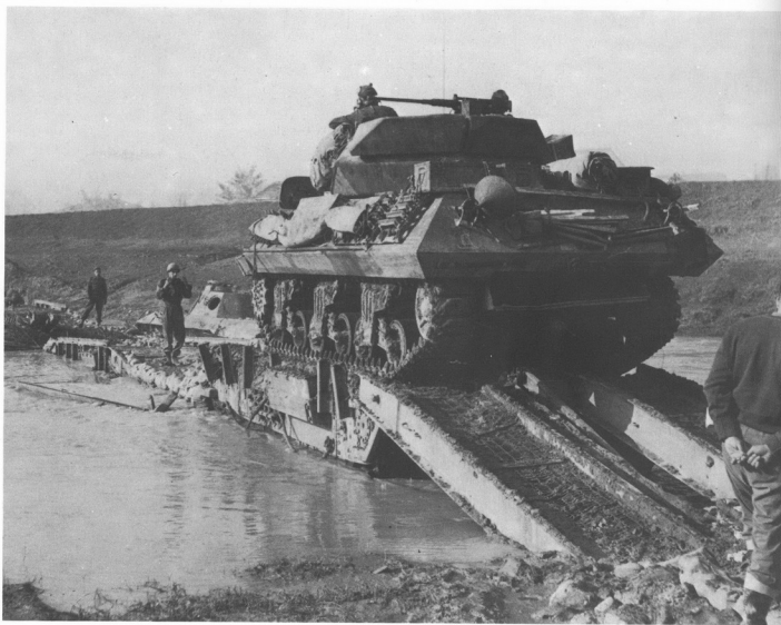
In British service the M10 was known as the Wolverine. This V Corps vehicle is seen being guided across the River Savio on 24 October 1944, using a causeway of Churchill ARKs. A 'dead' Panther lies beyond. The crew are clearly experienced at looking after themselves, as can be seen by the neat, secure stowage, the 'acquired' oversize funnel (an invaluable aid during replenishment), bivouac stakes and bucket. (Imp. War Mus.)
