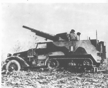
M3 in British service, firing in the supplementary artillery rôle. Maximum elevation obtainable was +29 degrees. (RAC Tank Museum)
