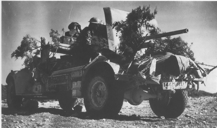
2pdr. portee and crew at range practice. In action as many of the crew as possible worked on the ground, as a direct hit would often dismount the gun, which would be thrown backwards, killing or injuring the men on the vehicle. (Imperial War Museum)
