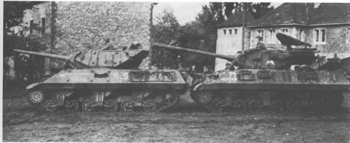
Although the two vehicles were carried on similar suspensions, the M36 (right) can easily be distinguished from the M10 (left) by its larger gun and distinctive turret. (Imp. War Mus.)
