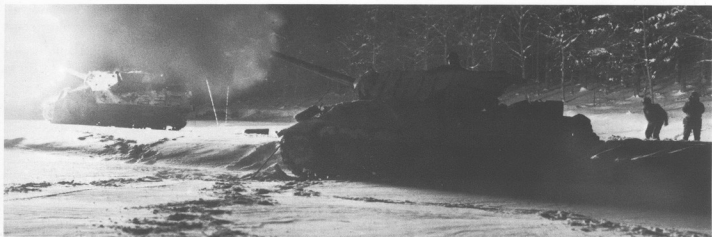
M10s firing in the indirect rôle at night. The occasion is an operational test of high/low flash propellants. The vehicle on the left is using standard ammunition, which produced a brilliant white muzzle flash, while that on the right is using a specially prepared charge which gave only a dull, red glow. (US Army)
