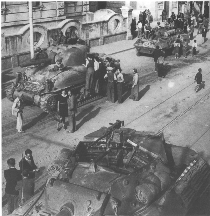
Elements of the American advance guard in Rome, 4 June 1944. Details of the close-defence .50 cal. mounting and stowage of 'ready' ammunition are clearly visible on the M10 in the foreground. Behind is an M4 medium tank and one of the unpopular M8 armored cars. (Imp. War Mus.)
