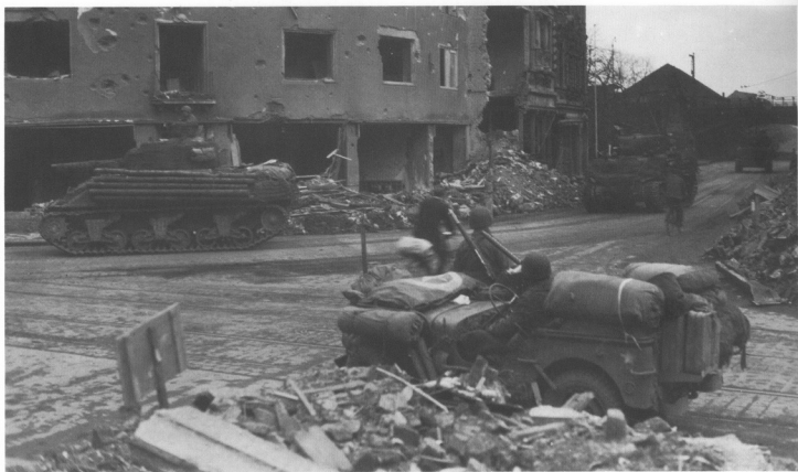
Krefeld, Germany, March 1945: Shermans of the Division with heavy logs lashed along the hull sides, and green cheese-cloth material strung round the vehicle as camouflage. In the foreground, a heavily-loaded jeep, with its lowered windshield in a canvas cover marked with the star and circle.
