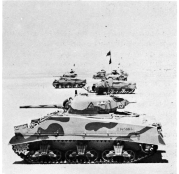
There were official Middle East camouflage schemes and patterns for Shermans which at least some units used. Here, at the end of the North African campaign, Sherman Is of 3rd CLY wear that laid down in June 1943 of Blue-Black over Light Mud; from December 1942 it had been Dark Green over Desert Pink, and before that a contrasting colour, at the CO's discretion, over Light or Portland Stone. (Sharpshooters)
