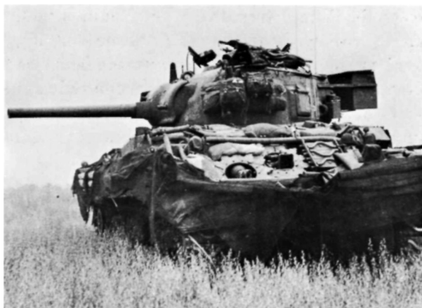
Sherman DD in action ashore. The flotation screen has been collapsed and partly cut away to give a field of fire to the 'lap' gun. Spare sprockets, track-plates and sandbags have been ingeniously arranged to give added frontal protection. It does not seem to have been a very general practice for the crew's packs to be hung around the turret, but this tank has a neat stowage rail added.
