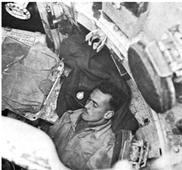
The inside of the turret was fairly cramped. Here a crew member (Canadian judging from the cap badge) sleeps under the gun between the gunner's seat and the commander's folding one. Some of the lavish supply of spare periscope heads can be seen round the gunner's seat.
