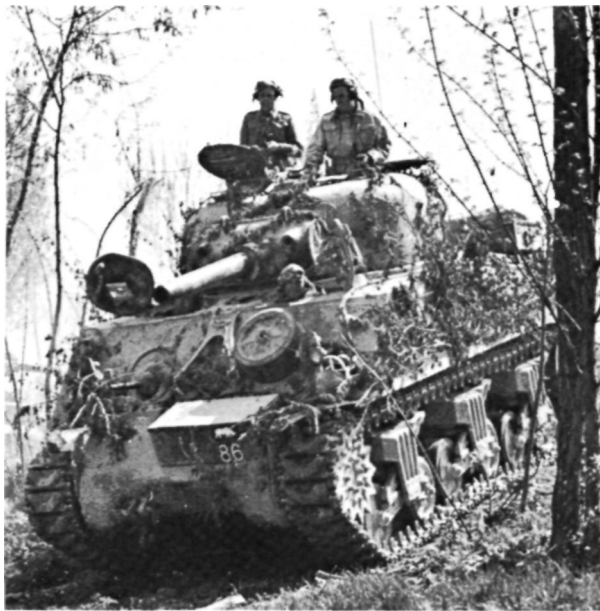
105mm Sherman IB of 9th Lancers in Italy. This tank has the cast nosepiece, 47° front plate with larger angled hatches, and the vision cupola for the commander.
