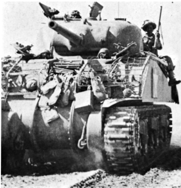
Sherman V on the move near Meiktila with anti-mine netting rigged and Bombay Grenadier escort embarked. Burma was the only theatre where tank crews regularly wore the American-style tank crash helmet.
