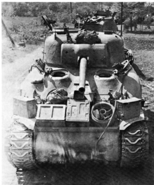
A Sherman II of 3rd CLY; the M34A1 combination gun mount and the extended end connectors on the metal chevron tracks can be clearly seen here. (Sharpshooters)
