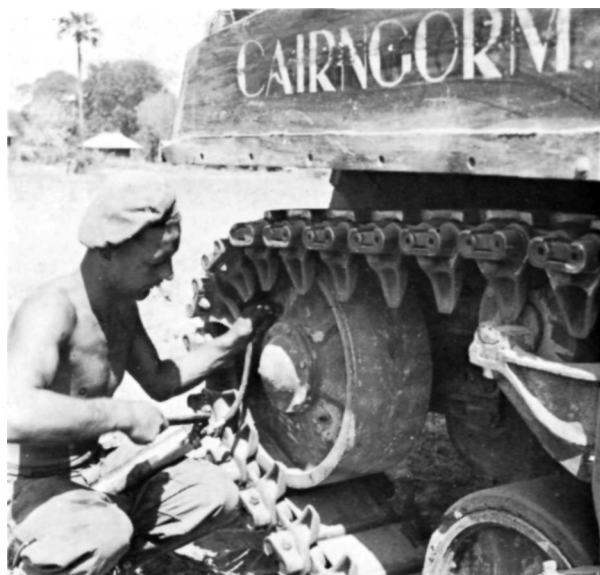
Even Shermans appreciated some maintenance! 'Cairngorm', the tank of the CO of 'C' Sqn., 116 RAC undergoes routine greasing in Burma.
