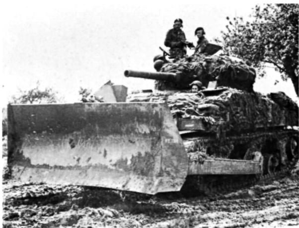
A variant which saw much use in Italy; the Sherman tank-dozer. This particular vehicle (in fact photographed in North-West Europe) has the heavy net and hessian strip camouflage used by some units in preference to vegetation, while the gun is wrapped in what looks like sacking, presumably to prevent reflections.
