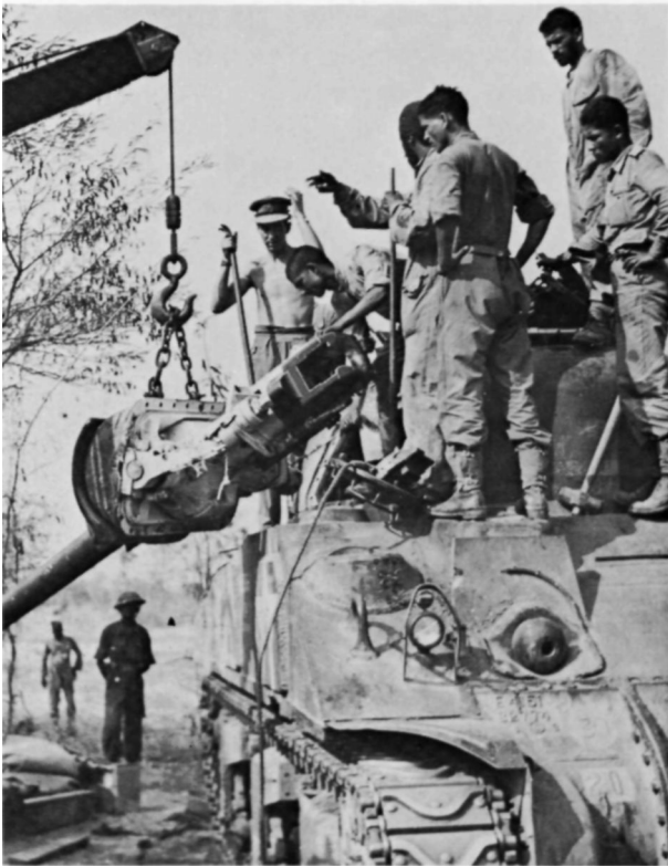
The M3 75mm gun in its M34A1 combination mount being lifted out of a Sherman in Burma. The co-axial Browning has already been removed from the mounting, and the 'lap' gun is not fitted in this tank, which has had additional armour welded in front of the co-driver's hatch; from the chip taken out of it, this was probably just as well !
