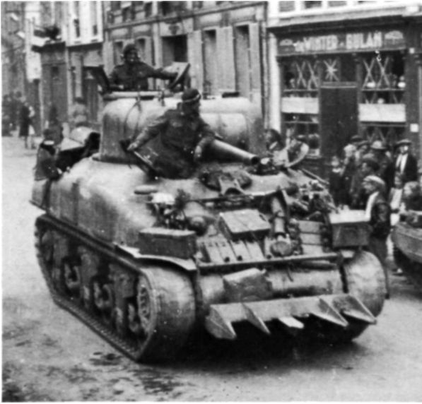
Sherman II of 3rd CLY fitted with the Culin prong device for cutting through bocage hedgerows. Many British units received these too late to be of much use. This tank is typically stowed for North-West Europe, with gear fore and aft but the sides clear. (Sharpshooters)
