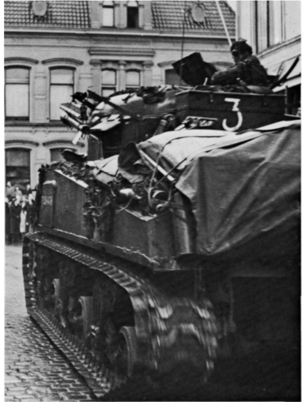
Sherman V of the Coldstream Guards in early 1945 with aircraft rocket rails rigged on either side of the turret. A troop number has been roughly painted on the turret bin, and the tank tarpaulin is being used to contain and protect loose gear on the back of the hull.
