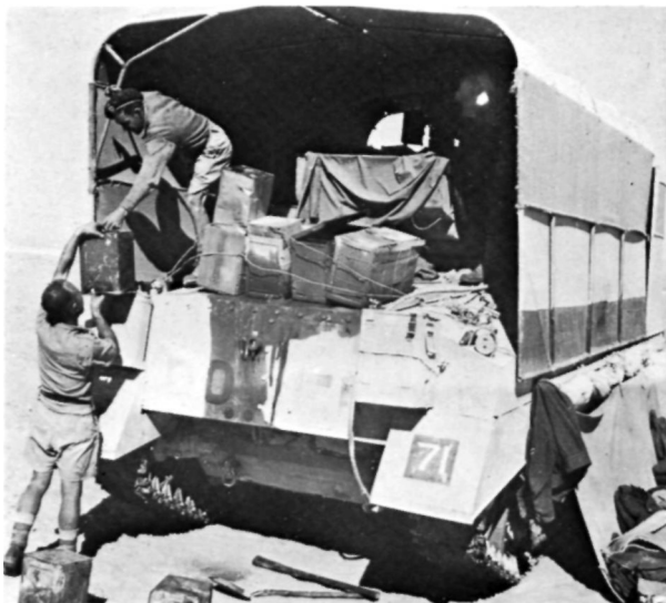
A diesel-engined Sherman III marked as belonging to an armoured regimental HQ, with its 'sunshade' camouflage rigged to make it look like a lorry. This disguise was used extensively before Alamein, and was the real reason that tanks had side rails fitted. Although the Shermans came with 'Ameri'cans, fuel was still supplied in four-gallon 'flimsies', as seen here, at this time.
