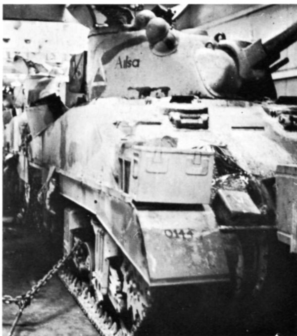
Tanks of 'A' Sqn., 3rd CLY en route to Sicily in the hold of a Landing Ship Tank (LST). The crew of the nearest tank, 'Ailsa', seem to have a mixture of the infantry-type rimmed helmets and the newer rimless RAC pattern. Side coamings and old ammunition boxes have been welded to this tank to provide improved storage. (Sharpshooters)
