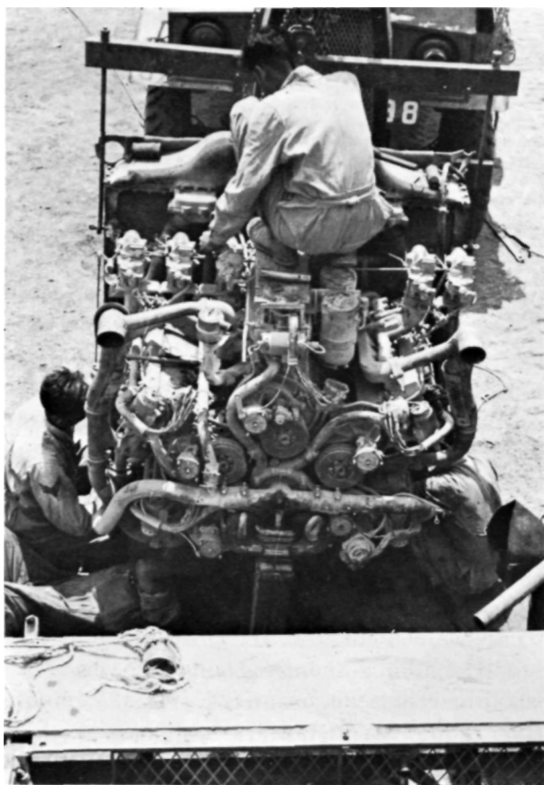
The Chrysler Multibank engine of a Sherman V. This is one of the later models, and all five carburettors can be seen at the top. The engine has been turned through 180° since lifting from the tank, and the radiators at the front of the engine can be seen beyond the fitter squatting on top.
