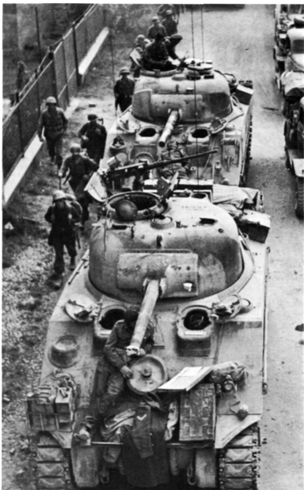
The end in Italy: Shermans near Bologna. The farther of the two tanks is a command or OP vehicle with a fitted cable reel and extra aerials mounted on the hull; it also has a late-pattern turret with applique armour and a loader's hatch. The nearer has rubber block chevron tracks.
