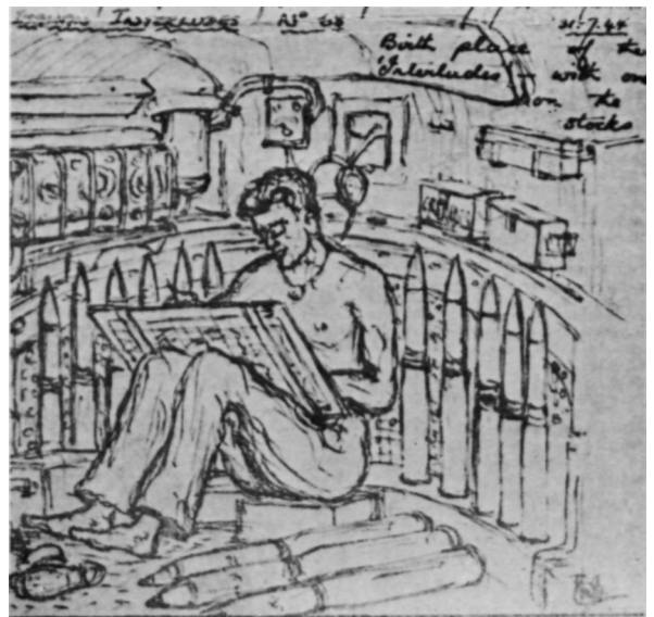
Inside the Sherman turret in action; and writing home during a quiet moment. The loader's glove was necessary to protect the hand when punching the round home, and when handling hot cases. The rounds stowed loose on the turret floor were common in Italy, and proved something of a hazard to the crew when the tank was bouncing over rough country. (Cessford)
