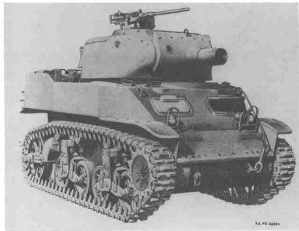
The M8 Howitzer Motor Carriage, showing driving compartment hatches moved down onto the glacis plate. (RAC Tank Museum)
