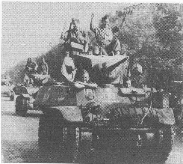
M5A1 of 1 er Escadron, 1 er Régiment de Marche de Spahis Marocains, 2 e Division Blindée parading in triumph down the Champs-Élysées, 26 August 1944. Below the bridge disc on the glacis are the French tricolour outlined in yellow, and white number '420463'. The yellow regimental code 'R' between two yellow bars is on a dark blue square. The divisional sign is painted on the right side of the hull. The Spahis wear scarlet sidecaps, and American overalls. (Daniel Ambrogi)
