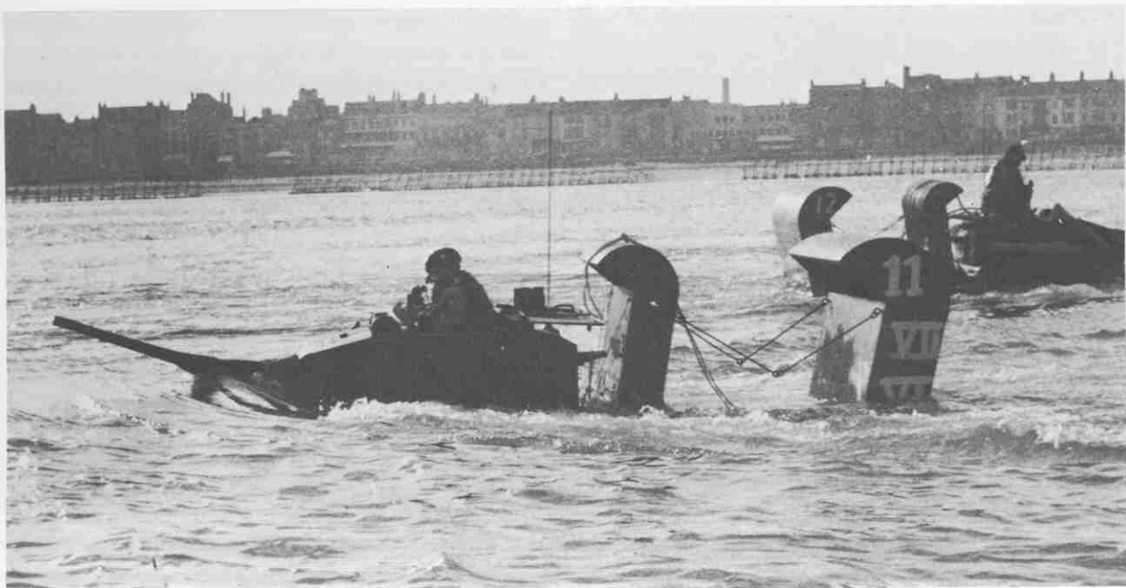
Some Stuarts were used experimentally as DD trials vehicles, but the tank lacked the heavy punch required for the rôle. (Imperial War Museum)
