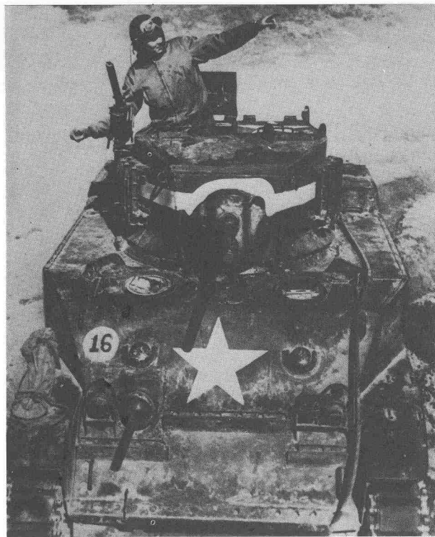
The M5 employed the same turret as the M3A1, but the shape of the engine compartment had to be altered to accommodate the twin Cadillac engines. (RAC Tank Museum)
