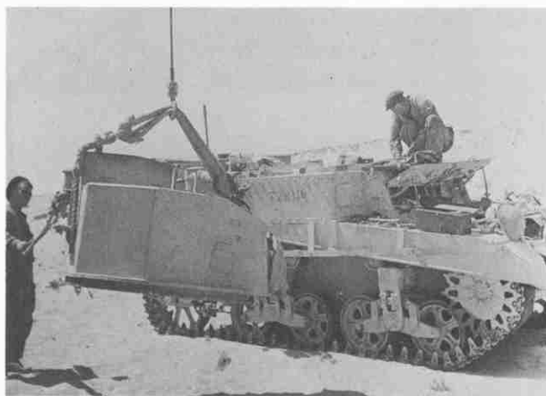
Ease of maintenance was one of the Stuart's prime virtues. Even in the Spartan conditions of a desert workshop it was a simple matter to remove the entire turret assembly, which rested on three support rollers set 120° apart. (Imperial War Museum)
