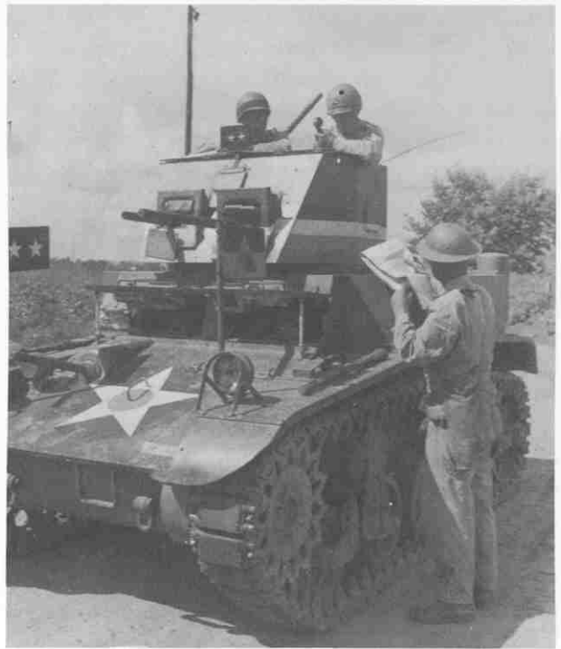
M1A1 Combat Car command vehicle used by Maj.-Gen. George S. Patton, commanding 2nd Armored Division, during 3rd Army's 1941 Louisiana Manoeuvres. The colour scheme is illustrated in Vanguard 11, US 2nd Armored Division, Plate A1. (US National Archives)
