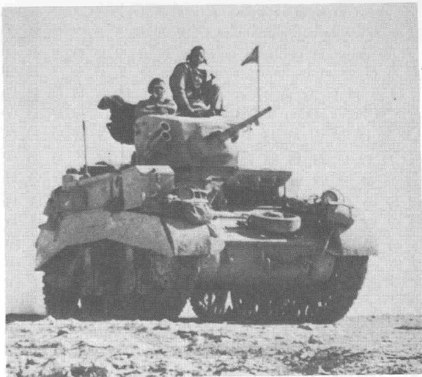
The M3A1 dispensed with the cupola, thus lowering the height to 7ft 6½in., and introduced hatches for both commander and gunner. This tank, serving with the British 8th Army in the desert, has been fitted with smoke-grenade dischargers; the sponson guns have been removed and an additional stowage locker has been welded in place on the left front, as viewed. (RAC Tank Museum)
