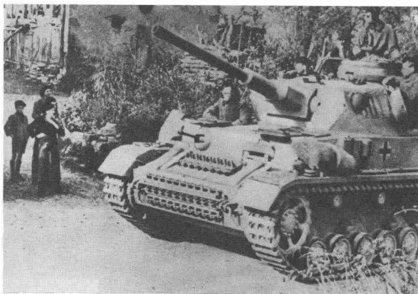
An unusual shot of an early Ausf. F2 L/43 without its muzzle brake. (RAC Tank Museum)
