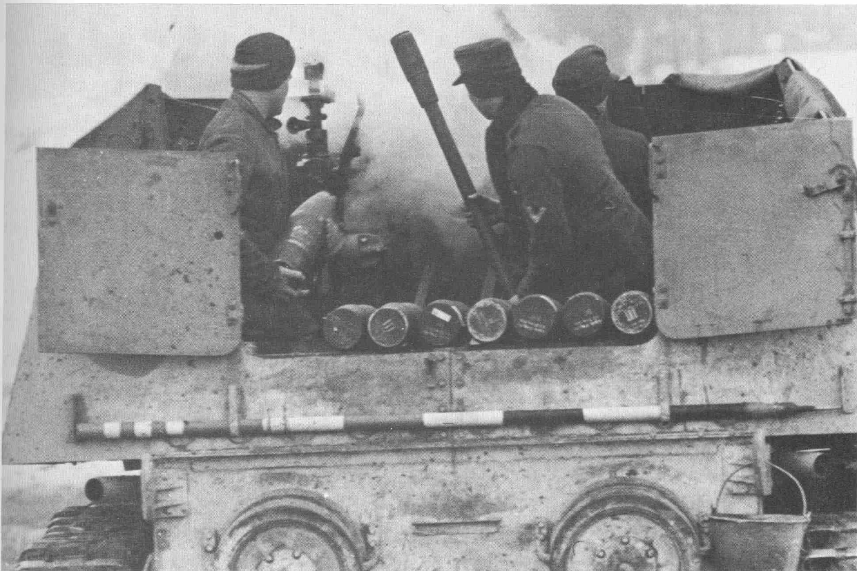
The Hummel in action. The striped pole forms part of the battery's survey equipment. (Bundesarchiv)
