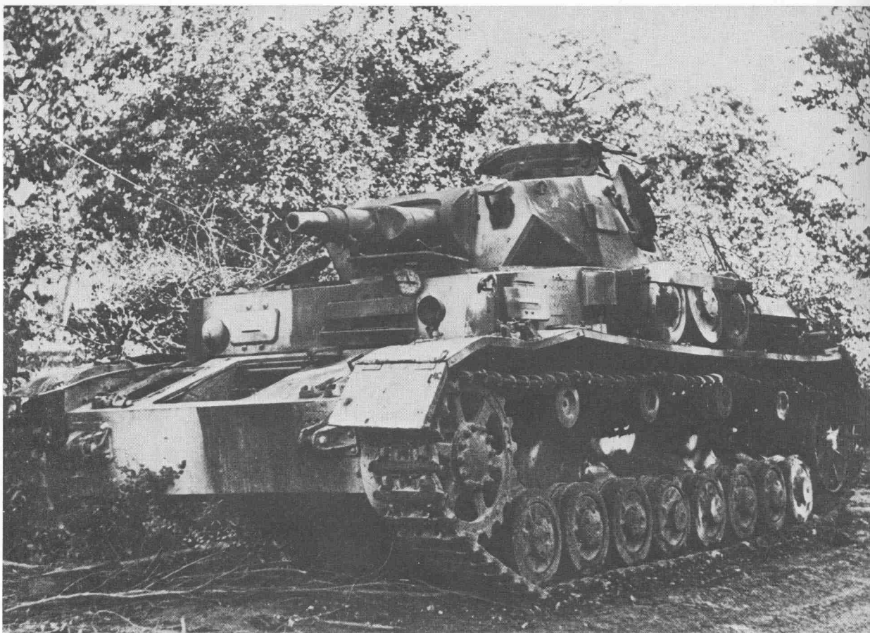
The Ausf. C was built in greater numbers than either of the earlier models. The hull machine gun was not fitted to this version, being replaced by a carbine port covered by a small circular hatch. See Plate A2. (RAC Tank Museum)
