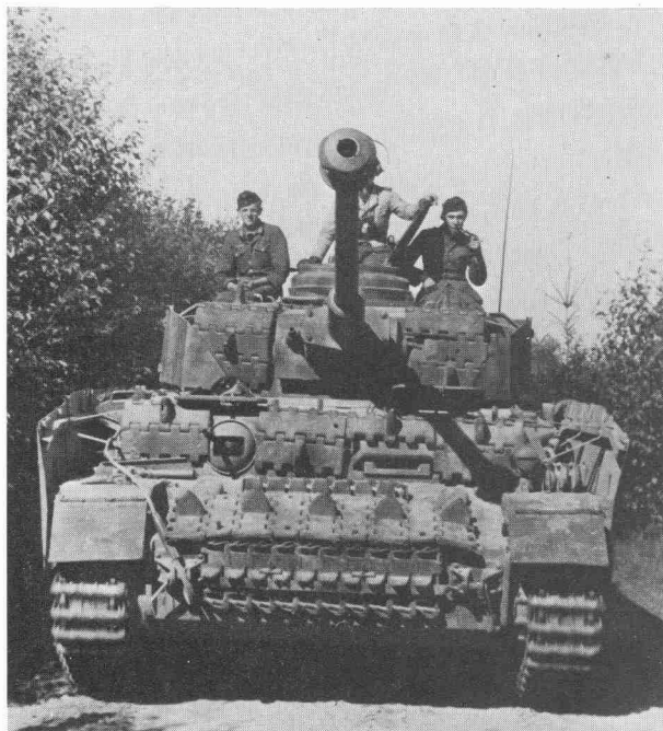
The final production version of the PzKpfw IV, the Ausf. J, dispensed with the power traverse system in favour of an increased fuel capacity. The crew of this vehicle have made good use of captured T-34 and other track links. (Bundesarchiv)
