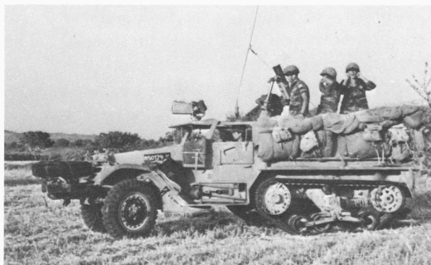
To give tank battalions close support, Zahal Ordnance developed this M9 half-track mounting the 120mm Soltam mortar. Perhaps their most surprising successes came on the Jordanian front, where they were credited with destroying a number of Pattons of the Jordanian 40th Armd. Bde. in the Six-Day War.
