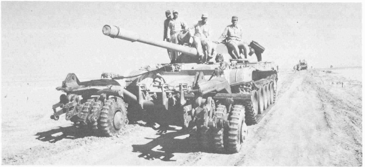
Egyptian PT-54 mine-roller clearing paths in the UN's Sinai buffer zone in March 1974. It is painted in the usual sand and drab brown camouflage. Many Egyptian tanks in 1973 bore two white stripes painted down the edges of the front fenders, as here; the significance is uncertain. (United Nations)
