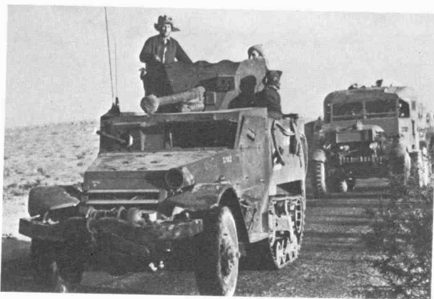
Probably the most potent Israeli AFV conversion—an M9 half-track with a British 6pdr. anti-tank gun mounted leads a column in the Negev, December 1948. This particular vehicle served with 8th Armd. Bde.; see Plate Br. Behind it is a Scammell wrecker.
