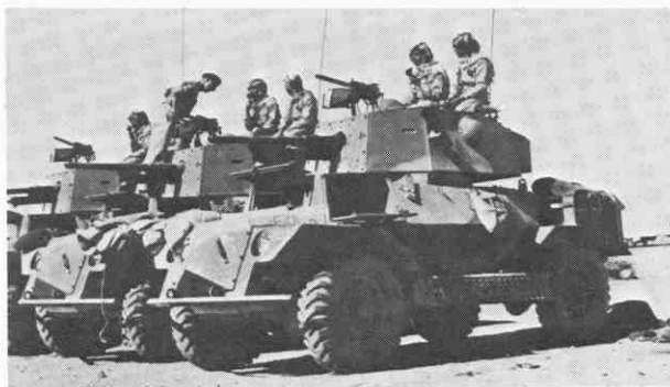
Platoon of Arab Legion Marmon-Herrington Mk IVF armoured cars—the most numerous single type of combat vehicle on the Arab side in the 1948 fighting. A company of Marmon-Herringtons was attached to each infantry battalion of the Legion; the nearest vehicle in this photo is the subject of Plate Az. (Imp. War Mus.)
