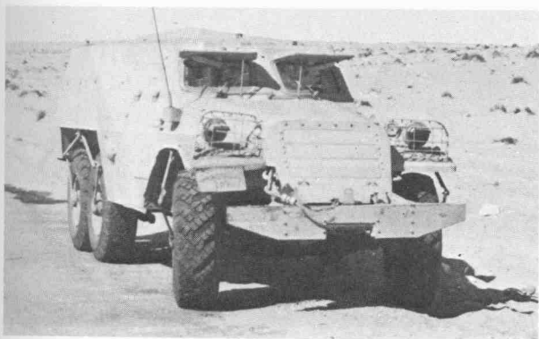
The standard Egyptian APC in 1956 and 1967 was the BTR-152, an armoured derivative of the ZIL-151 truck. This is the BTR-152 VI version, characterized by unusual external tyre pressure regulators on the wheels.
