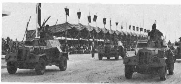
Egyptian Army Humber Mk III Reconnaissance Cars in a pre-war parade. Widely used on patrol duties, these elderly vehicles mounted a light machine gun and a Boys .5 anti-tank rifle—paltry armament by European standards, but perfectly effective against the improvised armoured vehicles on which the Israelis had to rely. (Imp. War Mus.)
